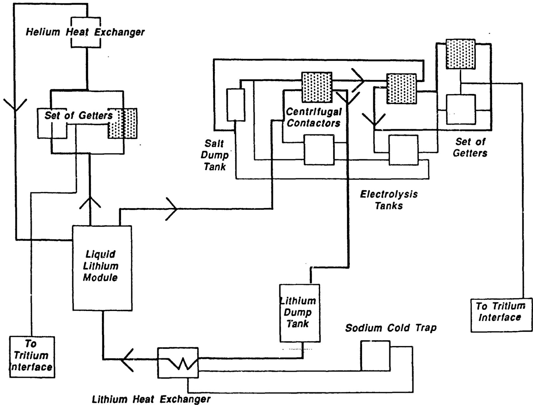
Fig. 3. Tritium Systems for Liquid Lithium Test Module.
