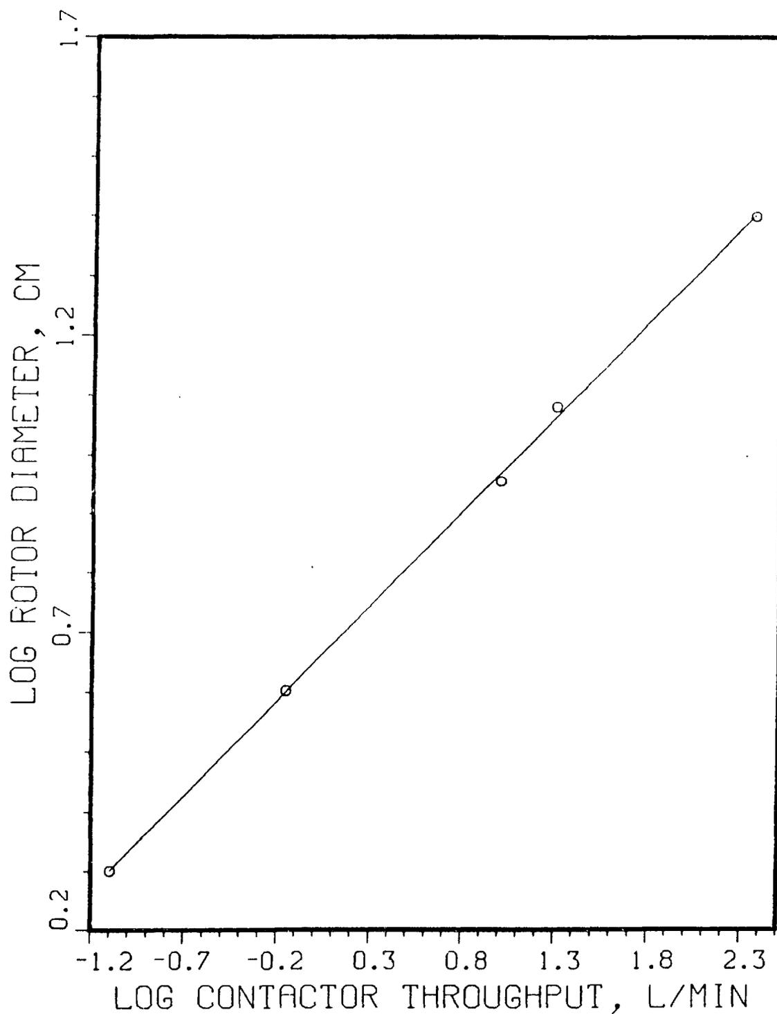
Fig. 1. Plot of Contactor Throughput as a Function of Rotor Diameter.
