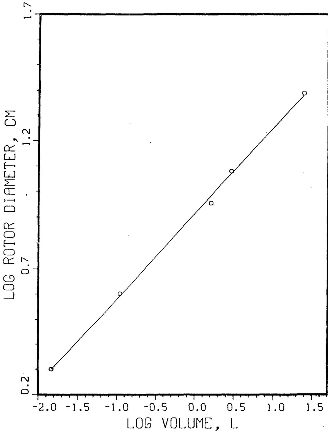
Fig. 2. Plot of Contactor Volume as a Function of Rotor Diameter.
