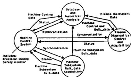
Figure 1. Instrument and Control System logical View
