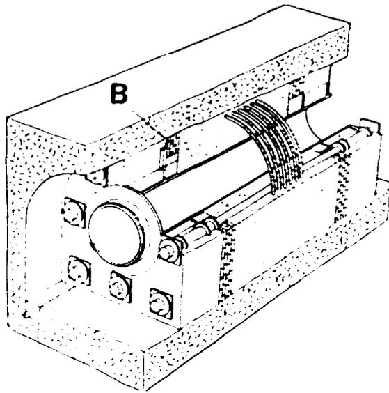
Figure 3-20. General view of the test arrangement with the central steel casing and tie-rods passing through the concrete plugs with bentonite sealings (B) at the ends and the sand-filled chamber. The latter simulated a richly water-bearing rock zone.
