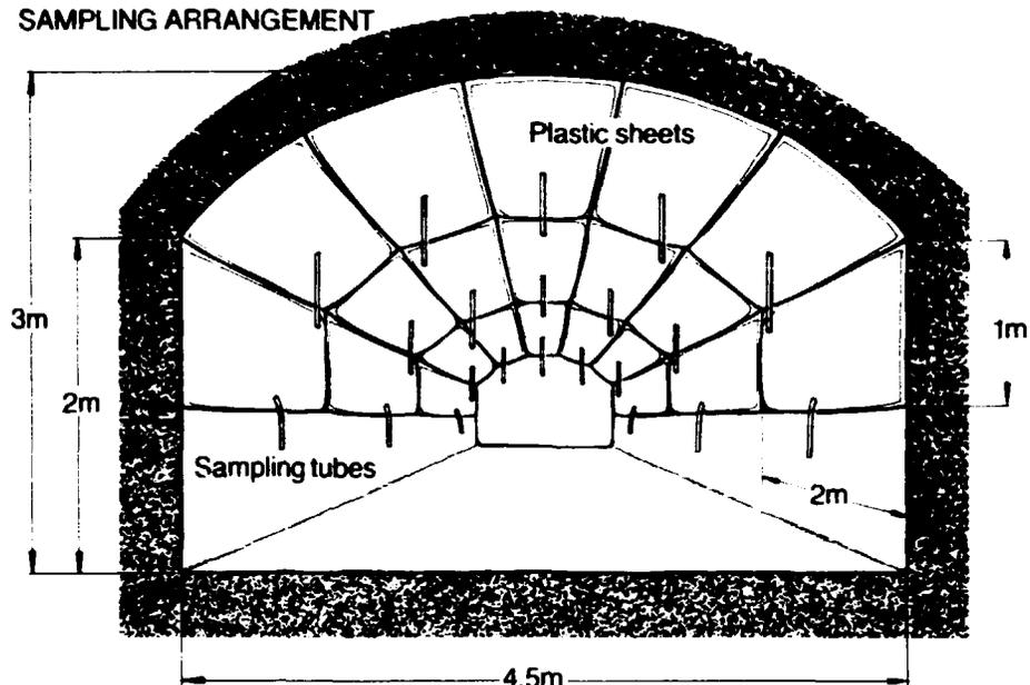
Figure 3-16. Sampling arrangement in the 3-D test site.
