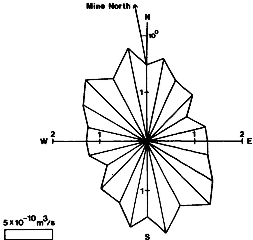
Figure 3-7. Relative flowrates for different directions of flow through the fracture network in Figure 3-6.
