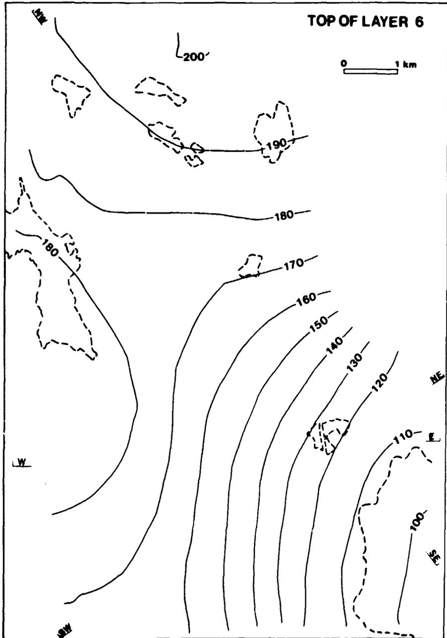
Figure 3-12. Contour map of the hydraulic head distribution on the top of layer 6, regional model.
