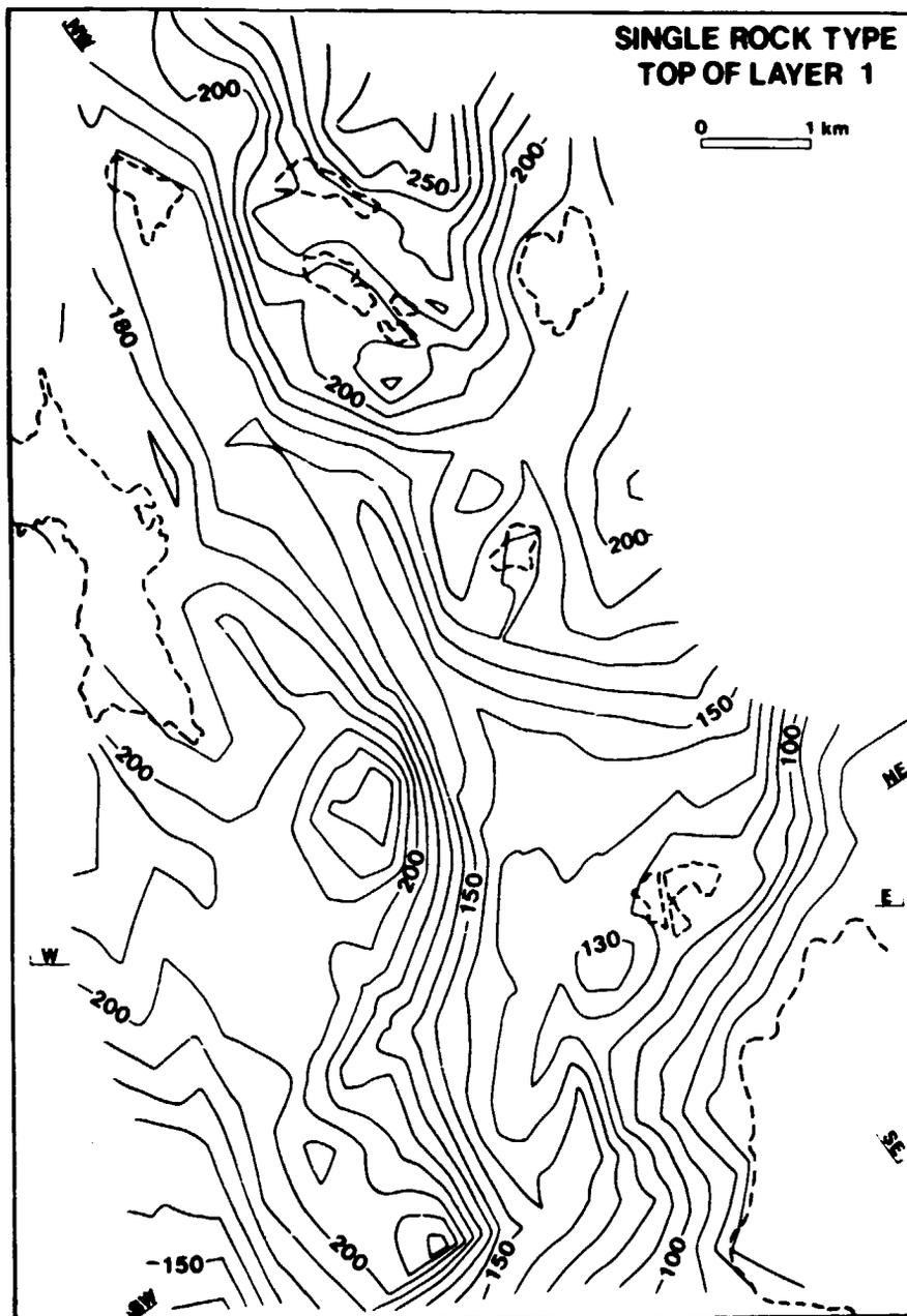
Figure 3-11. Contour map of the hydraulic head distribution on the top of the layer 1 (water table), regional model.
