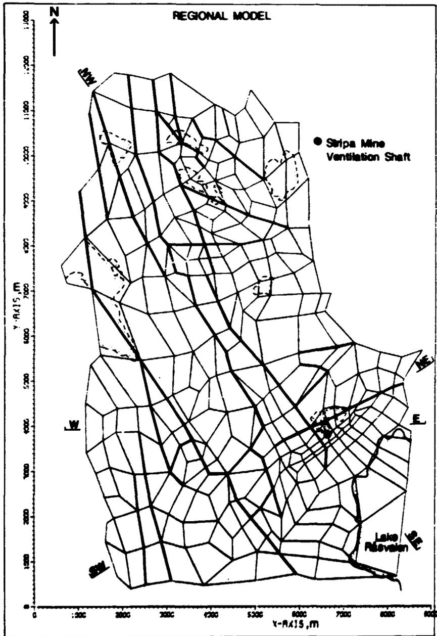
Figure 3-9. Finite element mesh for the regional model showing the location of the major lakes, fracture zones and the location of referenced cross-sections.
