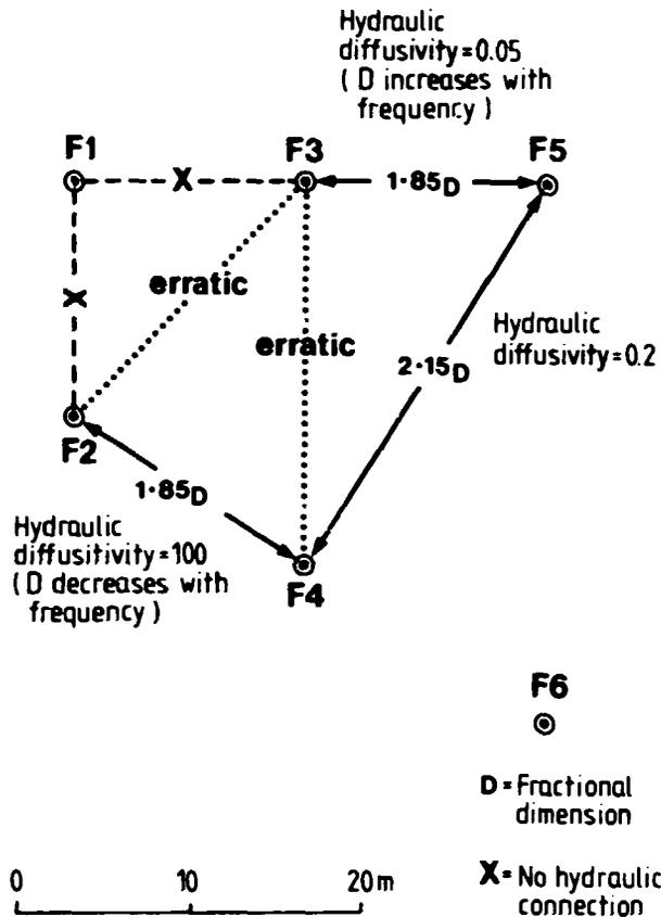
Figure 3-5. Values of hydraulic diffusivity and fractional dimension obtained from crosshole sinusoidal testing in Zone A.
