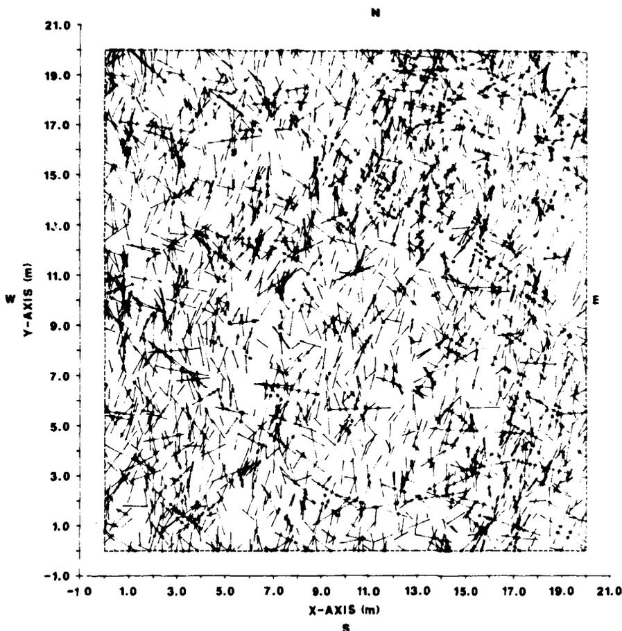
Figure 3-6. Simulation of the fracture network in the horizontal plane based on fracture geometry data from the Buffer Mass Test area.
