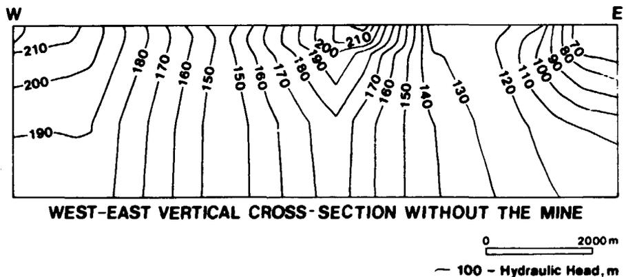
Figure 3-13. A west to east vertical cross-section (see Figure 3-9 for location) showing the distribution of hydraulic heads for the 3-D model with fracture zones but without simulating the effects of the mine.
