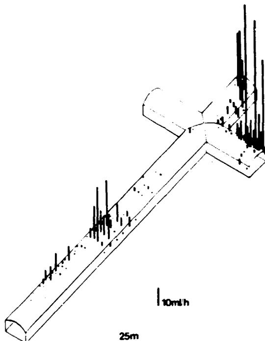
Figure 3-17. Water inflow rates into the upper part of the drift.
