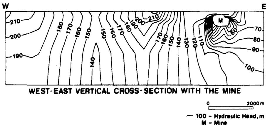
Figure 3-14. The same cross-section as shown in Figure 3-13 but including the dewatering effects produced by the mine on the hydraulic head distribution.
