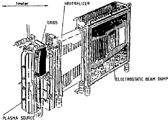
Figure 2: The neutral beam injection line including the source, neutralizer, and electrostatic beam dump (from Fumelli).
