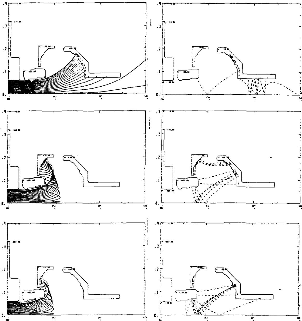
Figure 4: Fractional energy ion trajectories and secondary electrons with the fractional recovery electrode (FRE) present.
