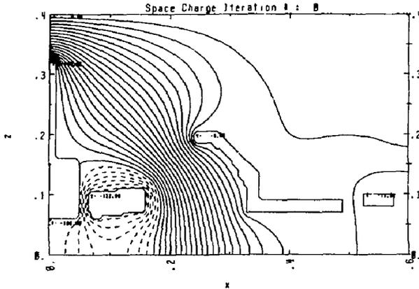
Figure 3: DART model of energy conversion system with second suppressor shown to the far right. The potential on the collector electrode is  $-5$  kilovolts and the potential on the second suppressor is  $-15$  kilovolts. These are the vacuum potential contours.
