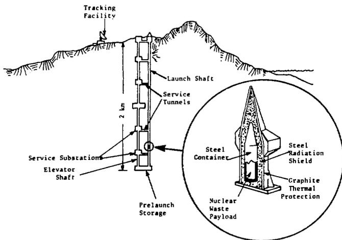
This space disposal concept involves the use of an electromagnetic launching shaft extending 2 km into the ground. Within it, a pulsed electric current would create a magnetic field and a wave of superheated gases, which would launch the waste from the earth at such a speed that it would eventually leave the solar system.
