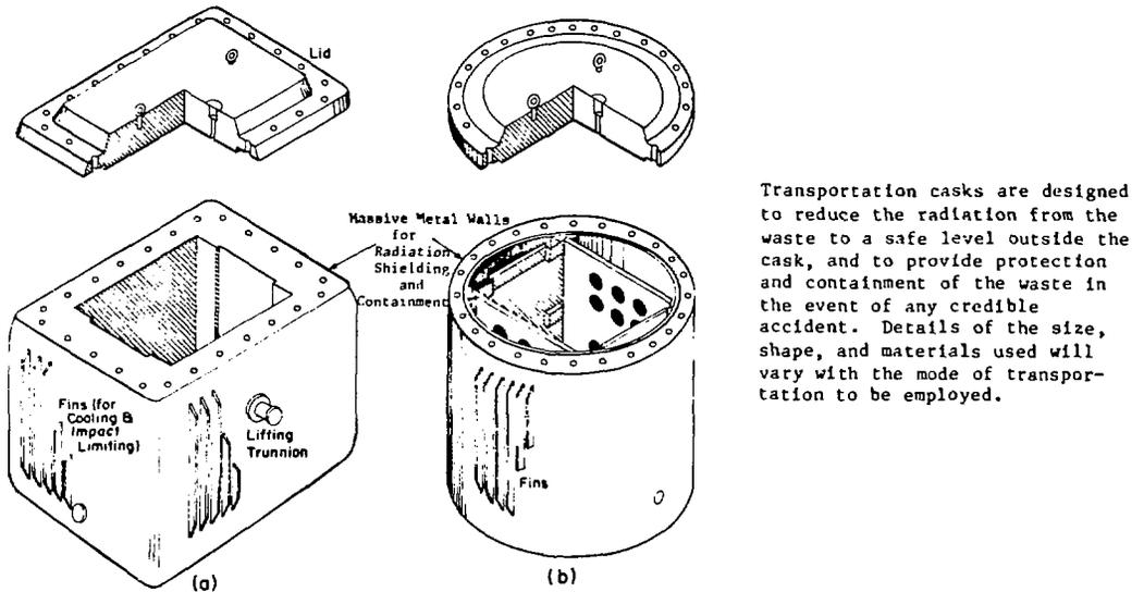
Transportation casks are designed to reduce the radiation from the waste to a safe level outside the cask, and to provide protection and containment of the waste in the event of any credible accident. Details of the size, shape, and materials used will vary with the mode of transportation to be employed.
