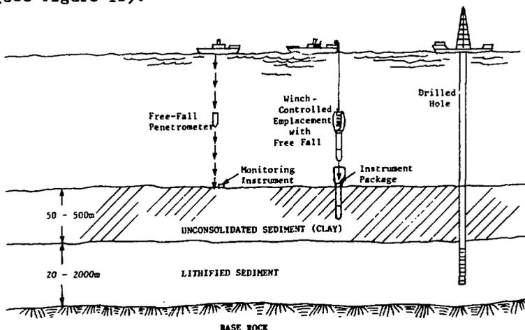
Nuclear fuel waste could be emplaced in the seabed by (1) encasing it in a penetrometer (a torpedo-shaped container) and dropping the penetrometer from a ship; (2) using a winch to control the fall of a penetrometer; or (3) drilling a hole in the sediments and placing the waste within it.
