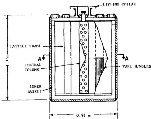
The reference container is an enclosed cylindrical vessel made of titanium. Each container would hold 72 bundles of used fuel stacked in two levels of 36 bundles each. The bundles would be immobilized in the container with a matrix of cast lead-antimony. The mass of a container of immobilized fuel would be about 8000 kg.
