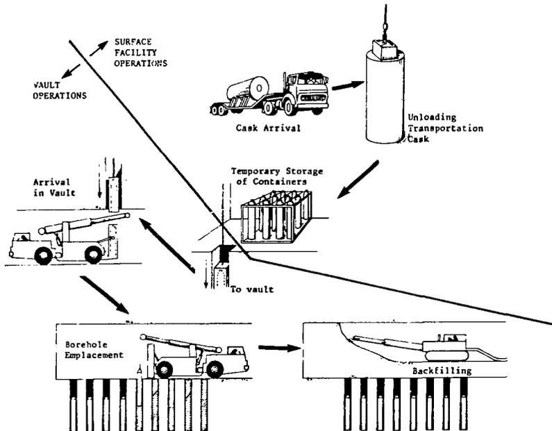
Containers of fuel recycle waste would be unloaded from the transportation cask, stored temporarily, and then lowered into the vault, where they would be emplaced in boreholes lined with buffer material. More buffer would be packed on top of the containers and the room would then be backfilled.
