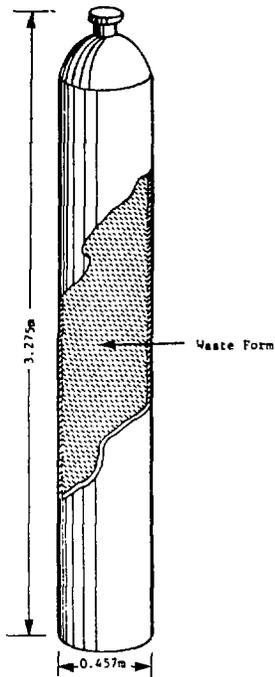
The reference container is a cylindrical vessel made of titanium. The mass of a container filled with the glass waste form would be 1675 kg.
