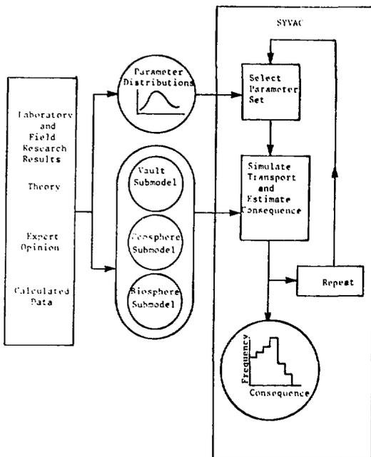
Laboratory and field research results, theory, expert opinion, and calculated data are used to develop the submodels and data used in SYVAC. The vault, geosphere, and biosphere submodels represent the release and transport of toxic substances. Some of the SYVAC input is in the form of probability distributions, from which single values are selected for each simulation. Many simulations are performed, and the results give a range of possible consequences.
