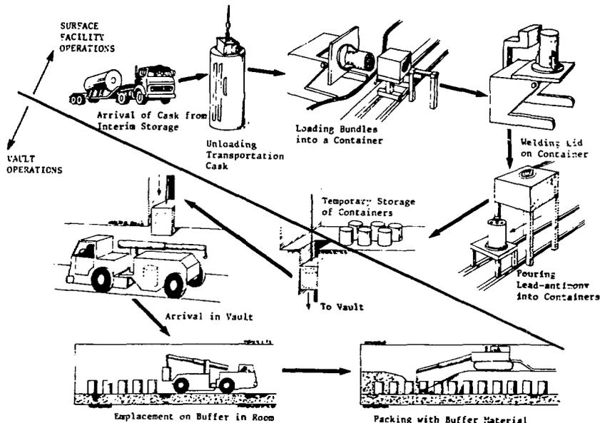
Used fuel bundles would be unloaded from the transportation cask, stored temporarily, and then immobilized in disposal containers. After a period of temporary storage, the containers of waste would be lowered into the vault, emplaced in a room on a bed of buffer material, and then surrounded with more buffer material. The room would then be backfilled.
