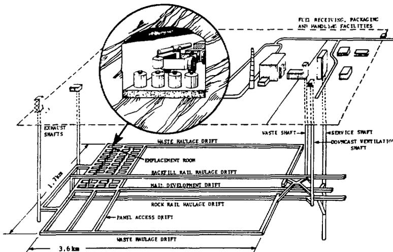
During vault construction, about  $9\,000\,000\text{ m}^3$  of rock would be excavated, half of which would be returned to the vault as part of the backfill. An area at the surface would be required for storage of rock and other materials. An additional area would be designated as an exclusion zone, so the total surface area required for the disposal centre would be about  $27\text{ km}^2$ . The area of the vault itself would be about  $7\text{ km}^2$ .
