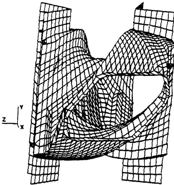
Fig. 3. MSC/NASTRAN model of the ATF vacuum vessel with port geometry.
