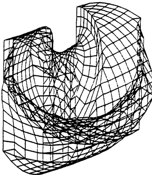
Fig. 2. Lockheed model of the ATF vacuum vessel, representing a 30° segment of the torus with no ports and with double helical troughs.
