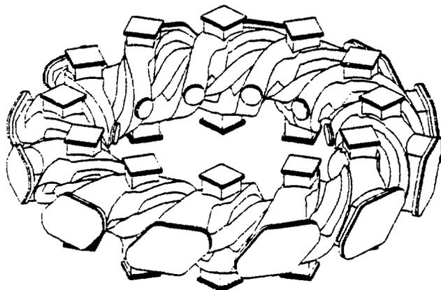
Fig. 1. Isometric diagram of the ATF vacuum vessel.
