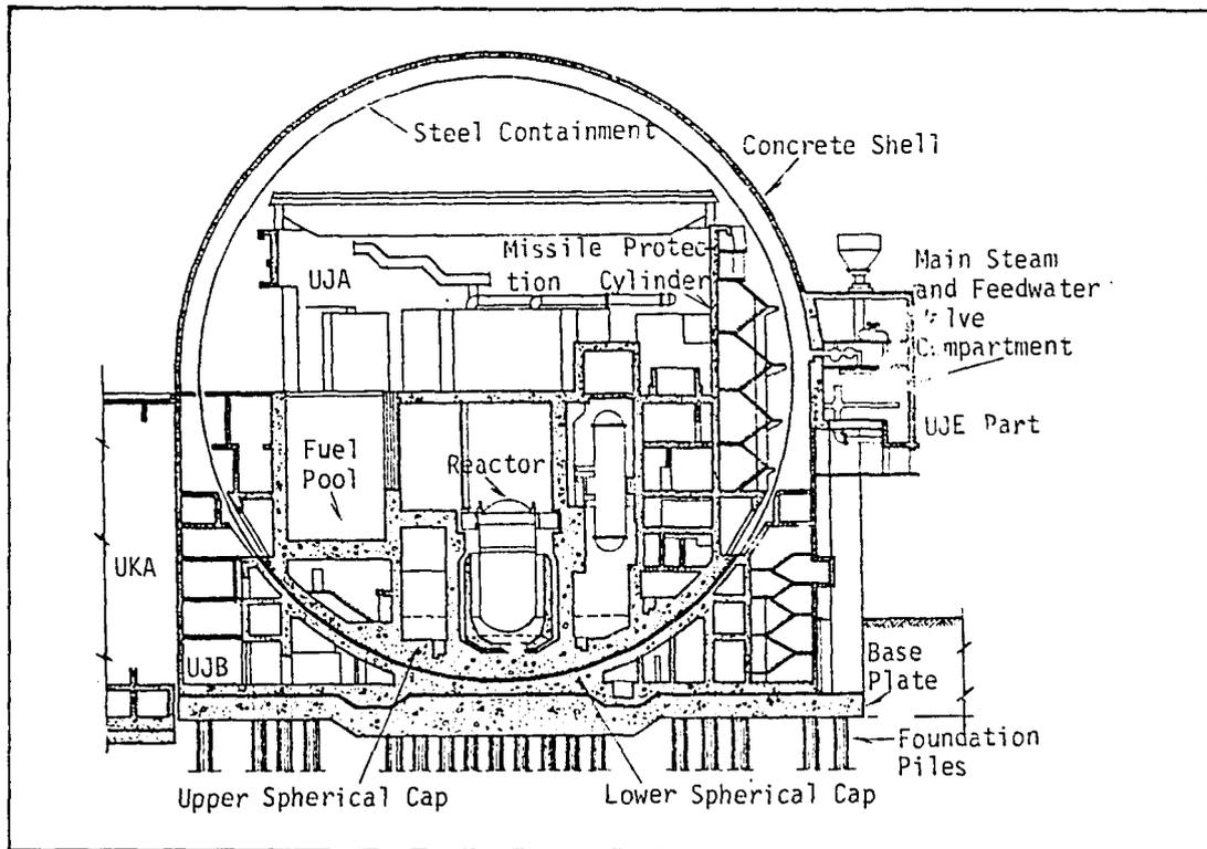
Fig. 1. General arrangement of the Reactor Building.
