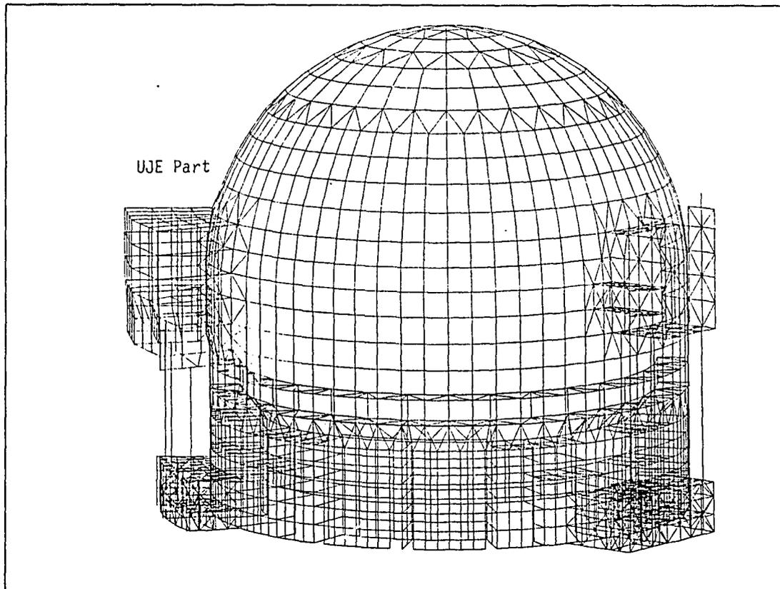
Fig. 2. Model for the external shell and the UJE Part
