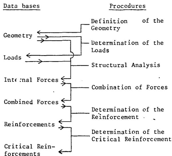
Figure 5. Organization of the design procedures and data bases.
