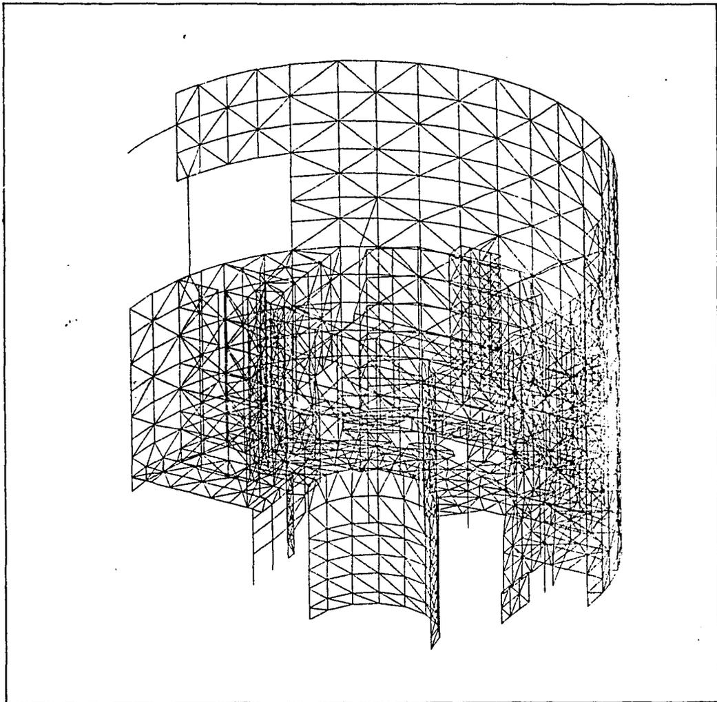
Fig. 4. Model for the analysis of the internal structures of the UJA part.
