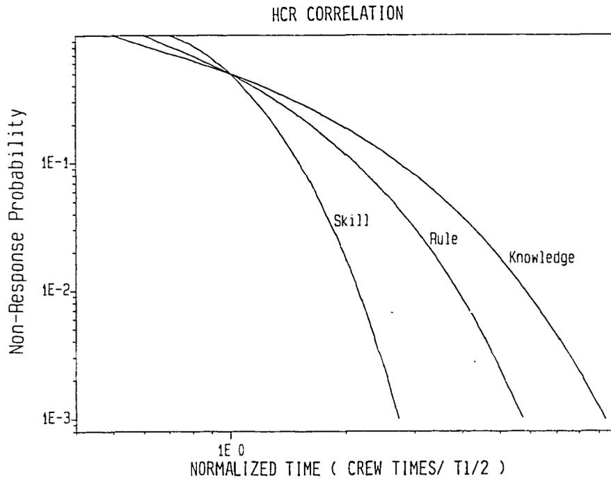
Fig. 2. Normalized Crew Non-Response Curves for Skill-, Rule-, Knowledge-based Cognitive Processing
