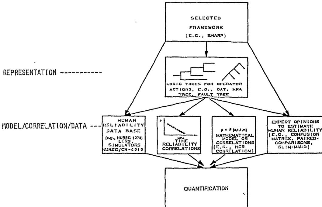
Fig. 1. Pathways for Quantification of Human Interactions
