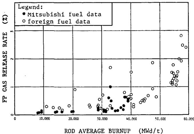
Fig. 5. FP Gas Release Rate
