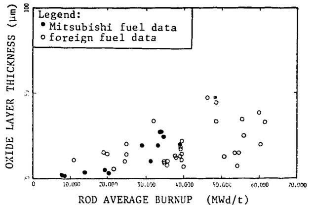
Fig. 6 Fuel Cladding Waterside Corrosion
