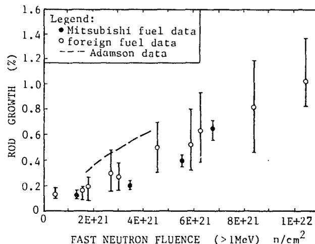
Fig. 3 Fuel Rod Irradiation Growth
