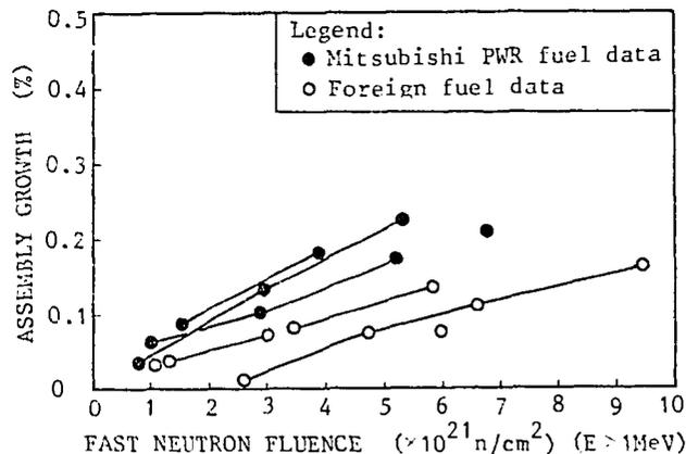
Fig. 2 Fuel Assembly Irradiation Growth
