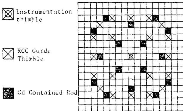
Fig. 10 Typical Gd Contained Rods Pattern (17 x 17)
