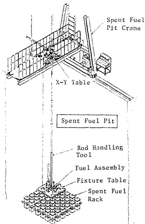
Fig. 15 Disassembling and Reconstitution Equipment for Fuel Assembly
