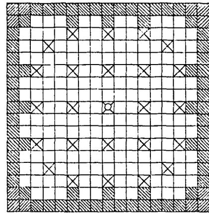
Fig. 12 Pu Enrichment Distribution in Mox Fuel Assembly (Example)
