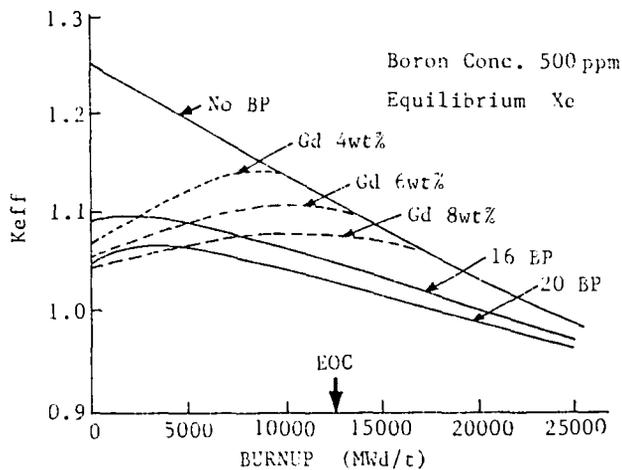
Fig. 11 Effective Multiplication Coefficient vs. Burnup (17 x 17, 16 Gd contained rods)
