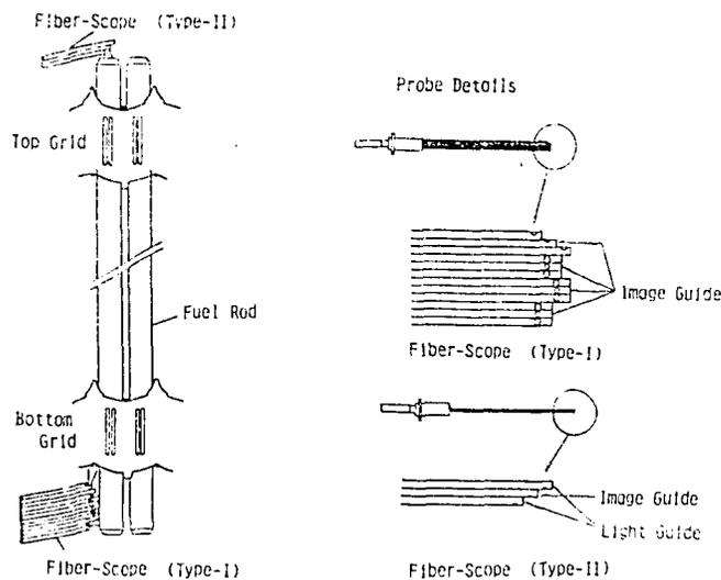
Fig. 14 View of Fuel Rod Surface Inspection with Fiber-Scope
