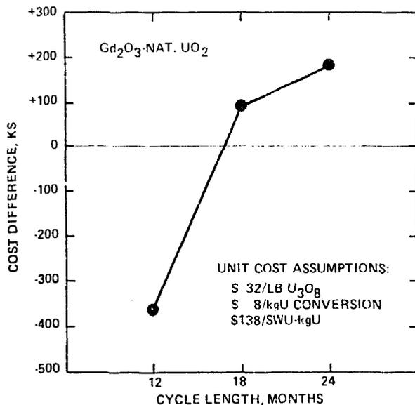
Fig. 4 Difference in Total Uranium Resource Costs (Ore, Conversion, Enrichment) Per Equilibrium Fuel Batch Relative to Reference Fuel Management Using  $B_4C-Al_2O_3$
