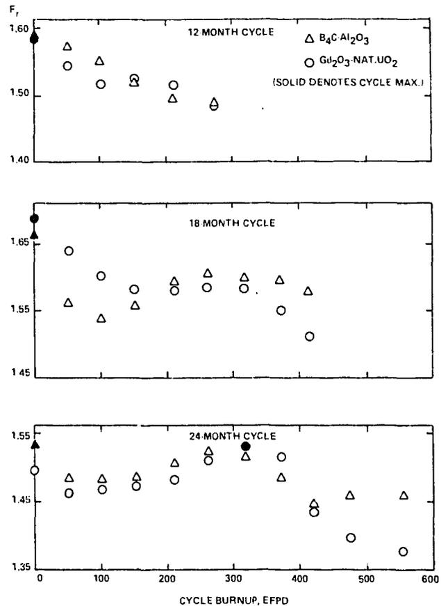
Fig. 3 Core Radial Peaking Factor ( $F_r$ ) vs. Cycle Burnup
