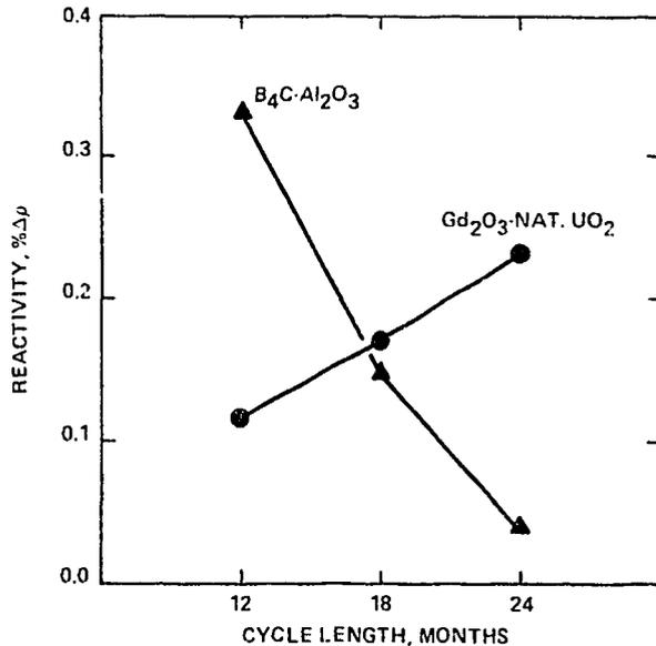
Fig. 2 Residual Core Reactivity Worth of Burnable Poisons in Equilibrium Fuel Cycles
