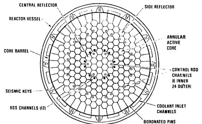
FIGURE 4. ANNULAR CORE AND CONTROL ROD LAYOUT
