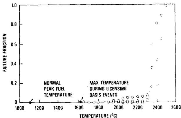
FIGURE 5. COATED FUEL PARTICLE INTEGRITY AT HIGH TEMPERATURES
