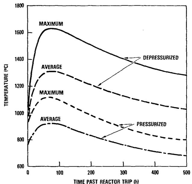
FIGURE 6. MHTGR TRANSIENTS DURING PRESSURIZED AND DEPRESSURIZED CONDUCTION COOLEDOWN
