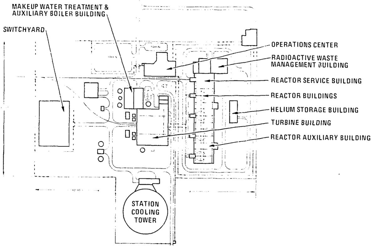
FIGURE 1. FOUR UNIT MHTGR PLANT LAYOUT
