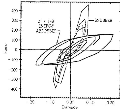
Fig. 4. Force-Displacement Behavior
