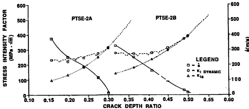
Fig. 6. Stress-intensity factor, crack-velocity, and static crack-arrest toughness versus crack-depth ratio for posttest elastodynamic analysis of PTSE-2.
