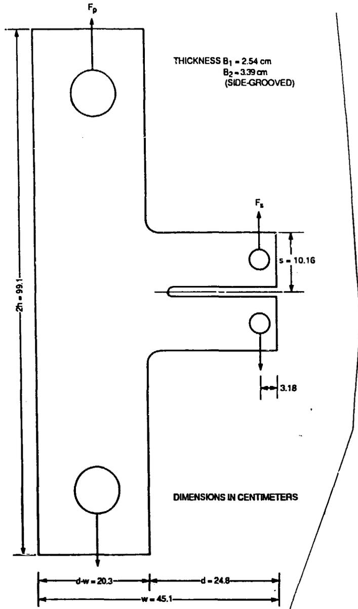
Fig. 8. Geometry and loading system of stub-panel crack-arrest specimen.
