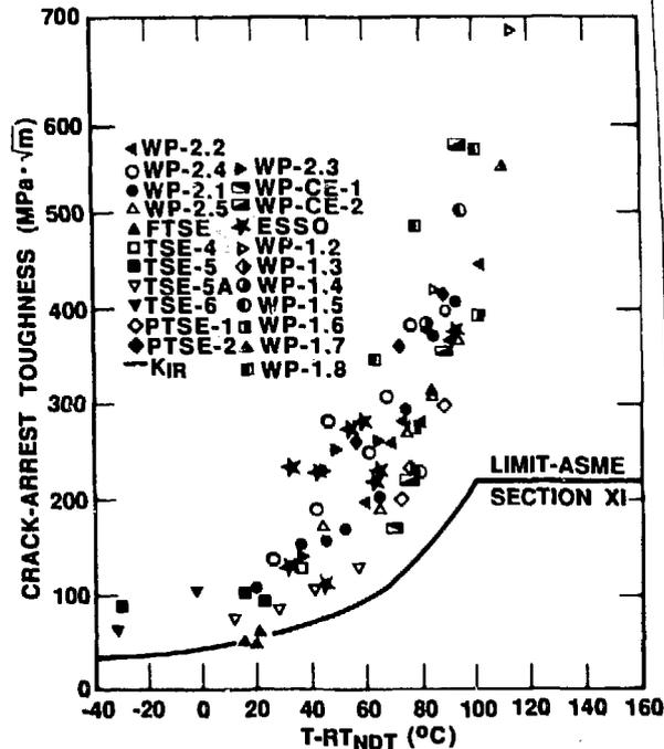
Fig. 7. High-temperature crack-arrest toughness data vs temperature ( $T - RT_{NDT}$ ) for wide-plate, PTS, and large-specimen tests.
