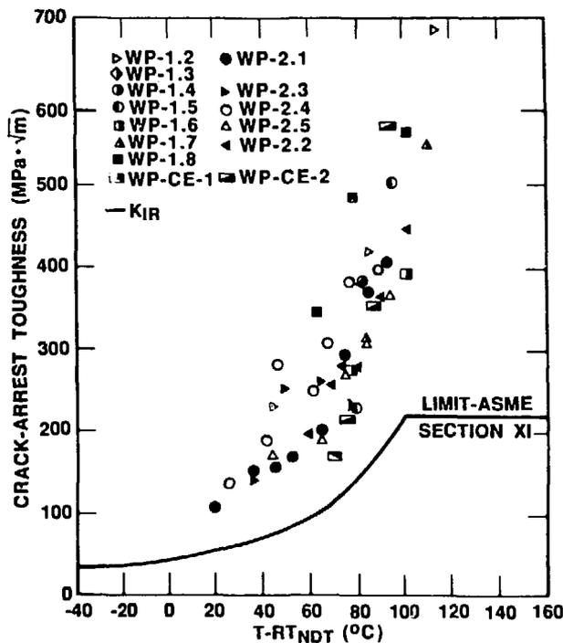
Fig. 2. Generation-mode (fixed load) crack-arrest toughness data versus temperature ( $T - RT_{NDT}$ ) for HSST wide-plate tests.
