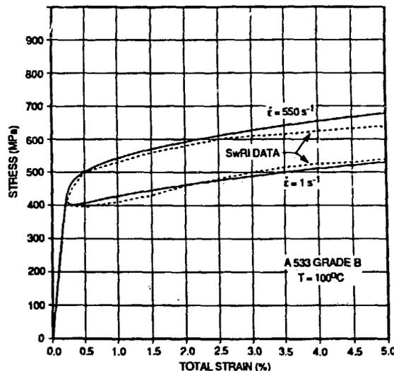
Fig. 10. Comparison of extended Robinson constitutive model predictions with measured stress-strain data for A533B steel at a temperature of  $100^\circ\text{C}$  and strain rates of  $1$  and  $550 \text{ s}^{-1}$ .
