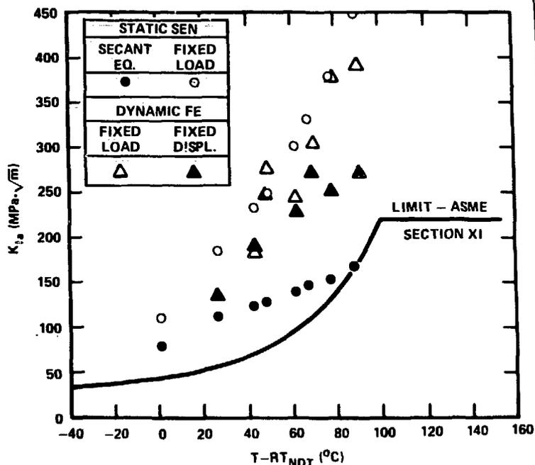
Fig. 3. Static and dynamic crack-arrest toughness determination vs temperature ( $T - RT_{NDT}$ ) for specimen WP-2.4.
