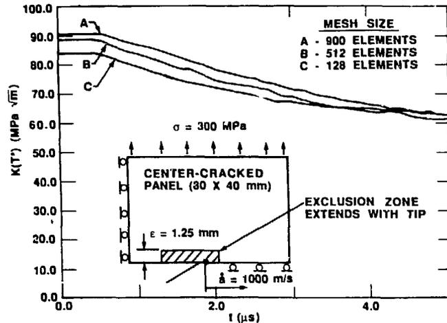
Fig. 15. Comparison of results  $[K_I(T^*) \text{ vs time}]$  from generation-mode viscoplastic-dynamic analyses of center-cracked panel for three mesh refinements and fixed exclusion zone ( $\epsilon = 1.25 \text{ mm}$ ).
