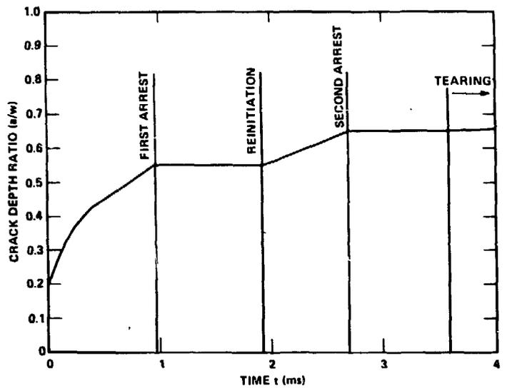
Fig. 12. Crack-depth history derived from strain-gage data for wide-plate test WP-1.2.
