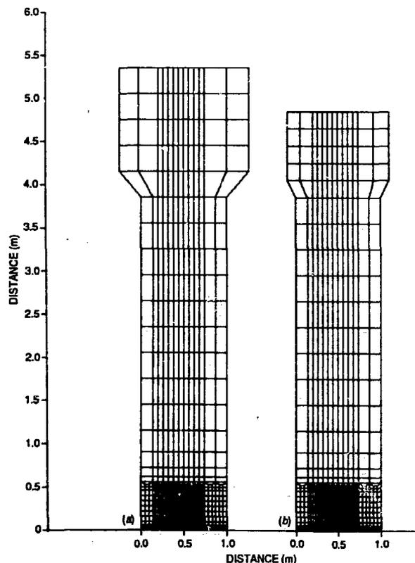
Fig. 11. Finite-element models used in dynamic analyses of tests WP-1.2 through WP-1.7: (a) model of WP-1.2 through WP-1.6, and (b) model of WP-1.7.
