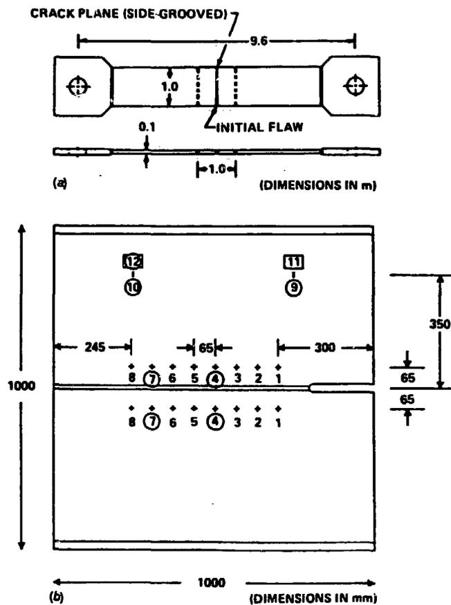
Fig. 1. Wide-plate assembly and crack-arrest specimen: (a) pull-plate assembly; (b) specimen with strain-gage locations.
