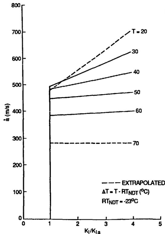
Fig. 4. Crack-tip velocity vs dynamic stress-intensity factor vs temperature inferred from A533B steel.
