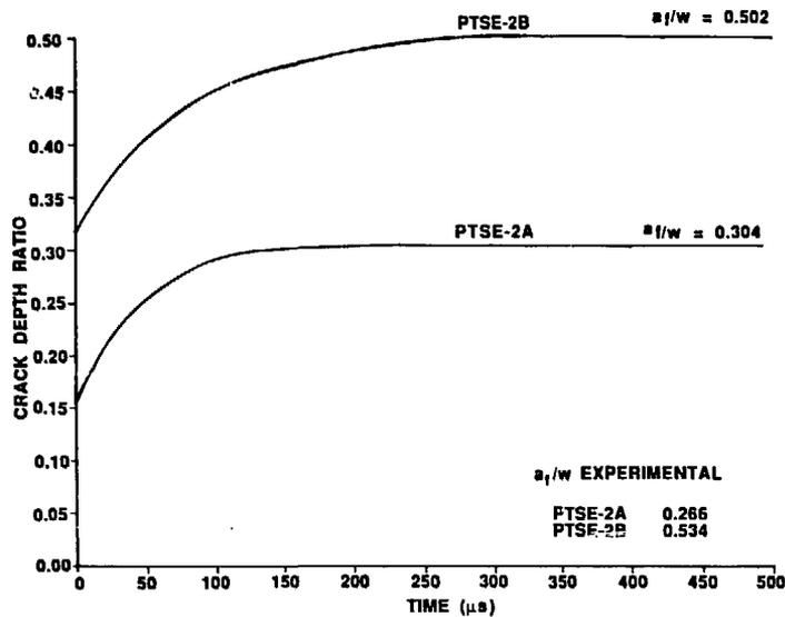
Fig. 5. Crack-depth ratio versus time for posttest elastodynamic analysis of PTSE-2.
