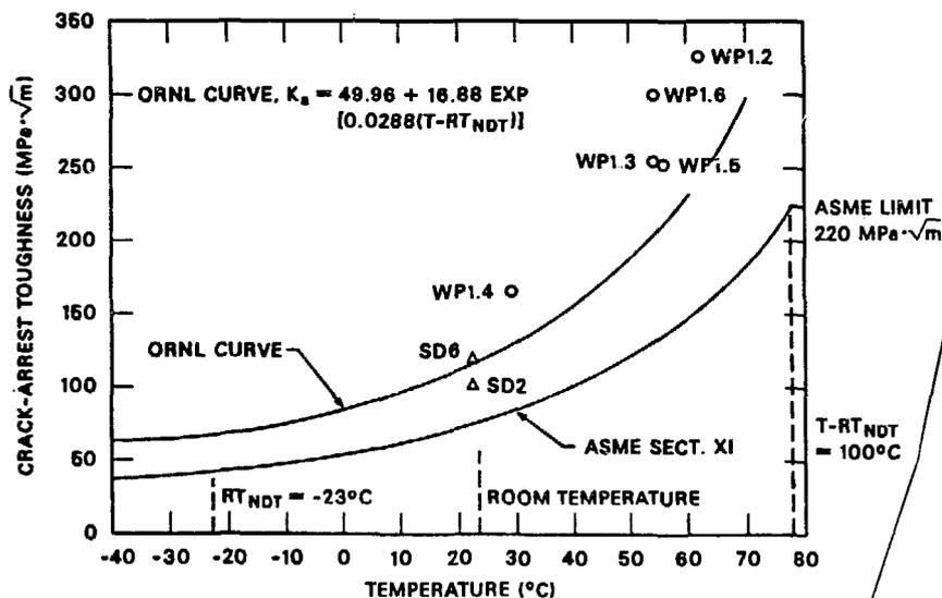
Fig. 9. Crack-arrest toughness data vs temperature for SwRI duplex specimen tests and HSST wide-plate tests.
