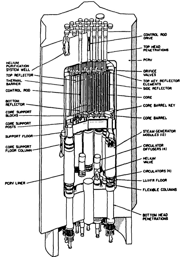
FIGURE 1 Fort St. Vrain Reactor Arrangement
