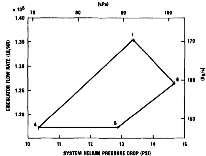
FIG. 13 MAIN CIRCULATOR OPERATING ENVELOPE AT 100% FW FLOW
