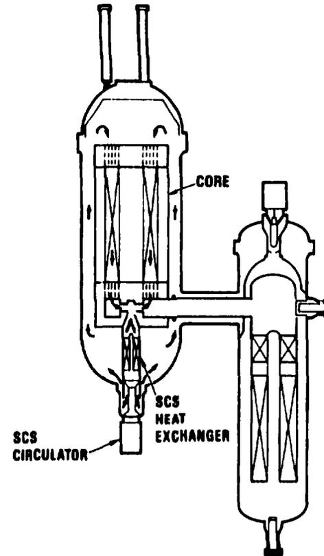
FIG. 6 PRIMARY COOLANT FLOW PATH DURING SYSTEM OPERATION
