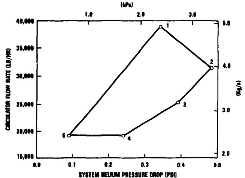
FIG. 15 MAIN CIRCULATOR OPERATING ENVELOPE DURING REFUELING
