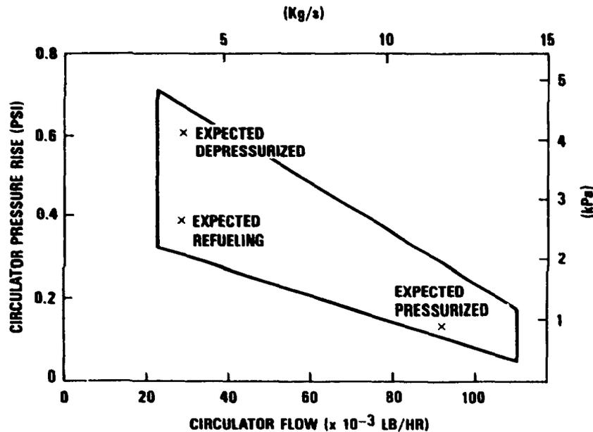
FIG. 17 SHUTDOWN CIRCULATOR OPERATING ENVELOPE
