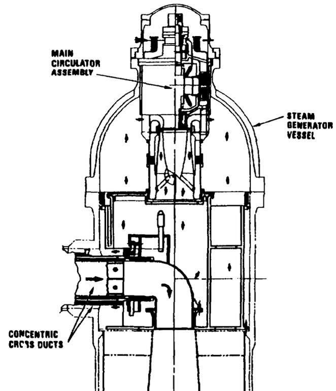
FIG. 12 MHTGR MAIN CIRCULATOR ARRANGEMENT
