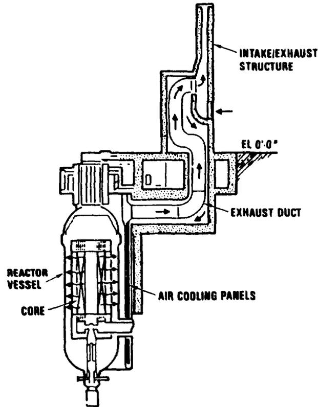
FIG. 7 RCCS (PASSIVE) DECAY HEAT REMOVAL
