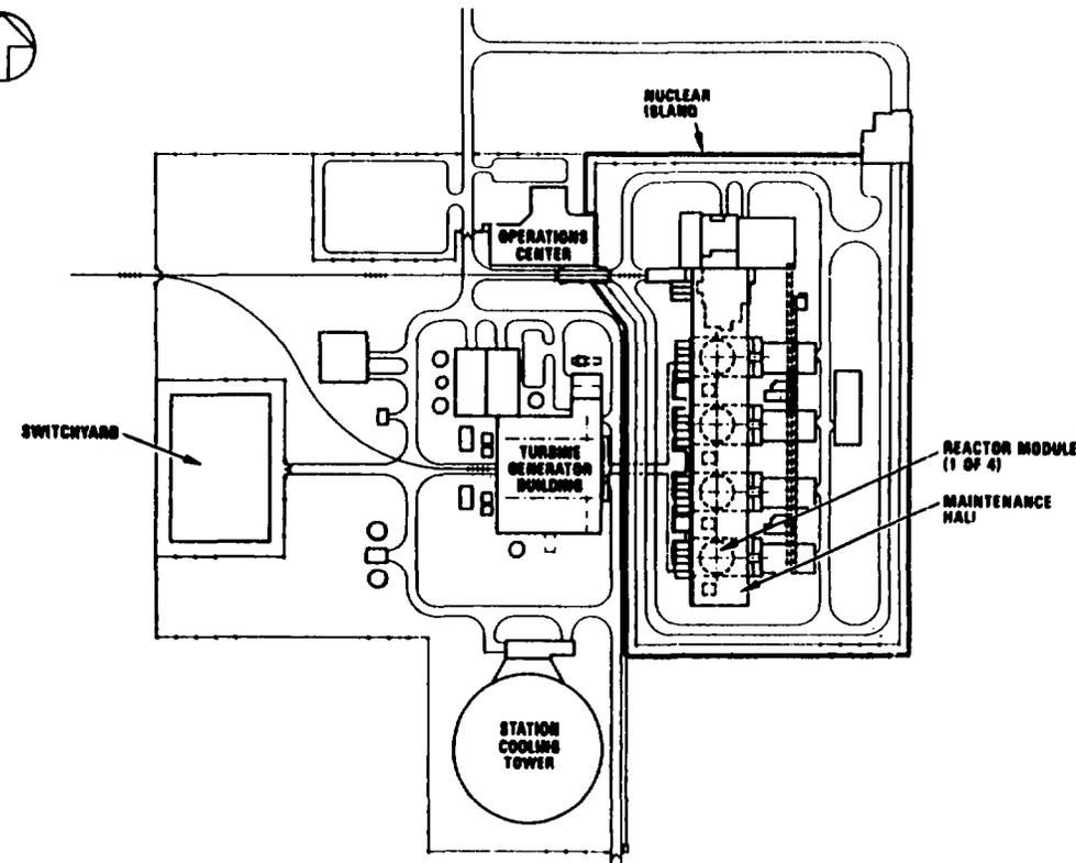
FIG. 1 MHTGR SITE PLOT PLAN
