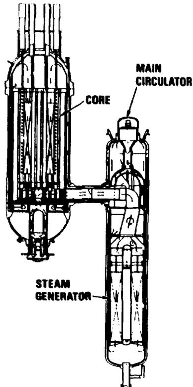
FIG. 5 PRIMARY COOLANT FLOW PATH DURING HEAT TRANSPORT SYSTEM OPERATION
