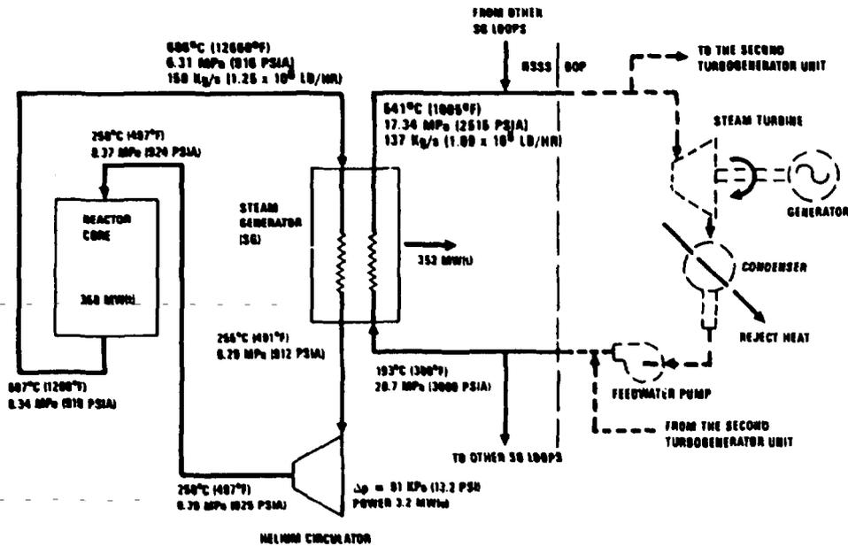
FIG. 2 HEAT BALANCE DIAGRAM FOR 350 MW(t) MODULE
