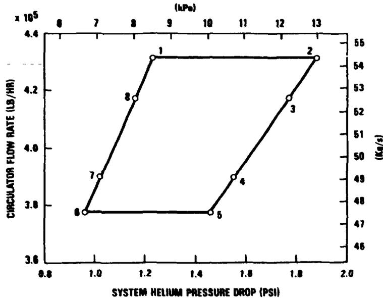
FIG. 14 MAIN CIRCULATOR OPERATING ENVELOPE AT 25% FW FLOW
