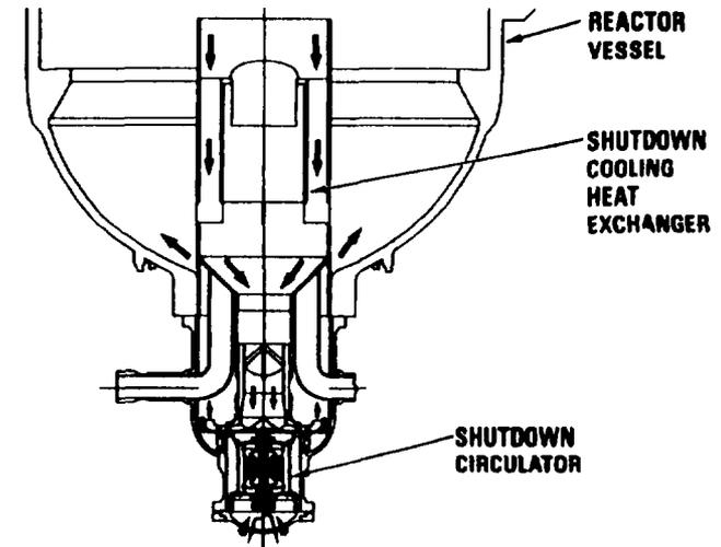
FIG. 16 SCS CIRCULATOR ARRANGEMENT
