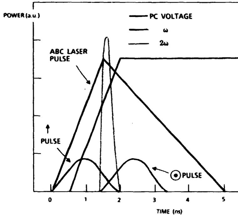
Fig. 2 Calculated time dependence of the  $2\omega$  short pulses as produced by the system represented in the previous figure
