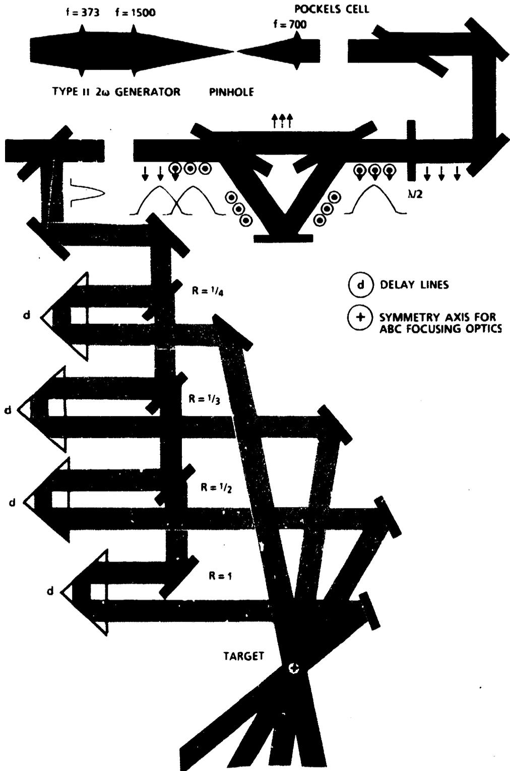
Fig. 1 The system used to generate four short light pulses at  $2\omega$  for optical diagnostics in the ABC experiment
