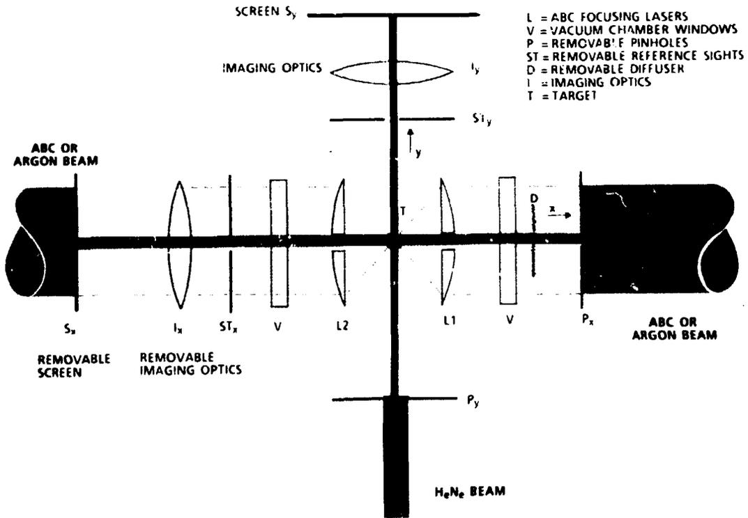
Fig. 10 Schematic view of the alignment optics
