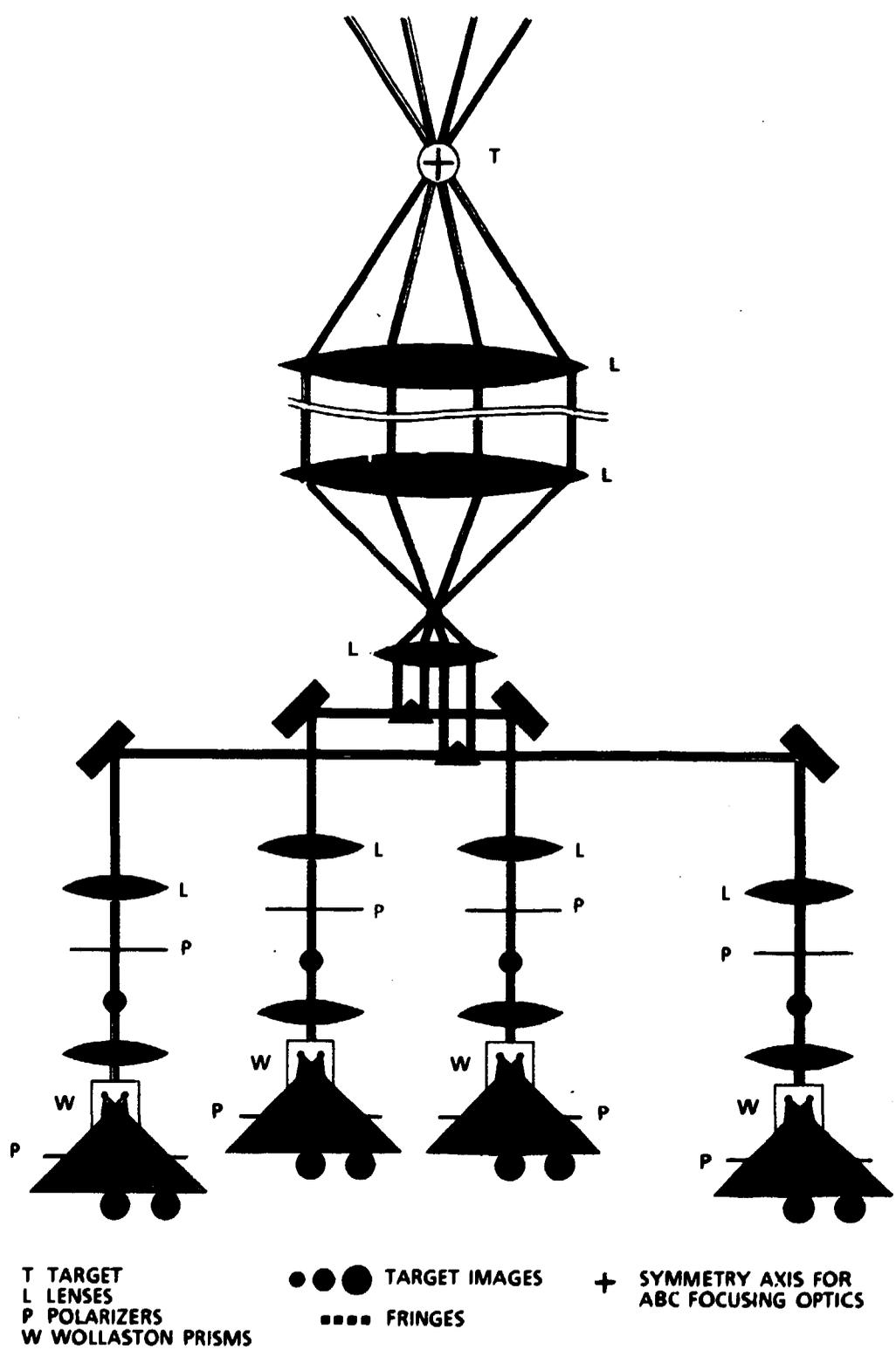
Fig. 4 The imaging system for the optical diagnostic
