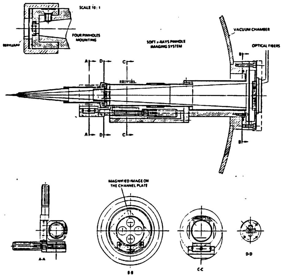
Fig. 7 The ABC pin-hole camera soft X-rays imaging system
