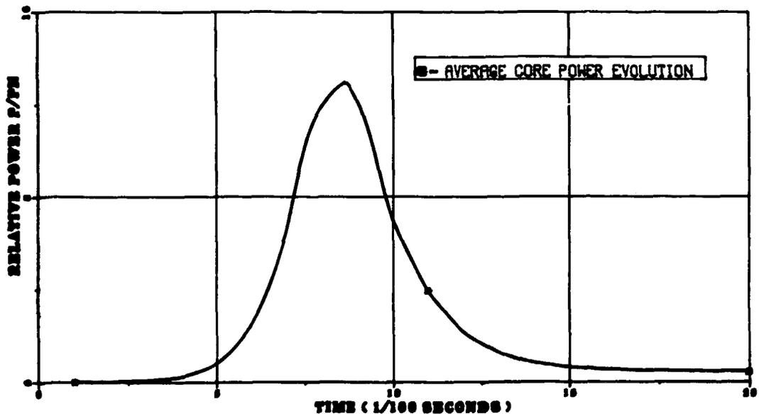
Fig. 5. Nuclear power for 1-D neutron kinetics 0-0.2s
