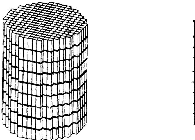
Fig. 1. Constitution of axial cross section libraries by 3-D - 1-D condensing.
