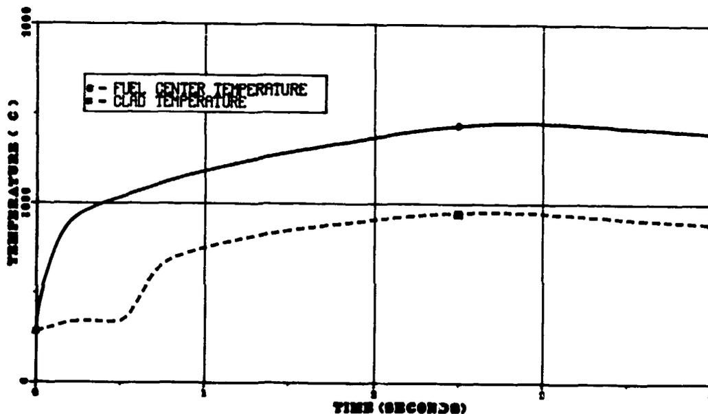
Fig. 6. Hot spot temperature versus time
