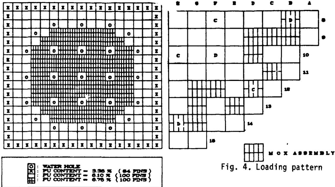
Fig. 3. Assembly zoning and plutonium distribution
