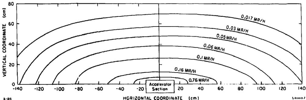
Fig. 16. Average x-ray dosage distribution around S-band (seven-cavity,  $2\pi/3$ -mode) accelerator section (300 MV/m surface field,  $2.5 \mu\text{sec}$ , 120 pps).
