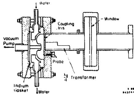
Fig. 4. Cross-sectional view of demountable C-band cavity.
