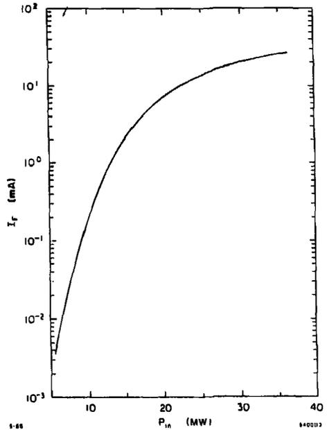
Fig. 14. Field emitted current transmitted through downstream window (right-hand side in Fig. 6) to Faraday cup, as a function of peak input power.
