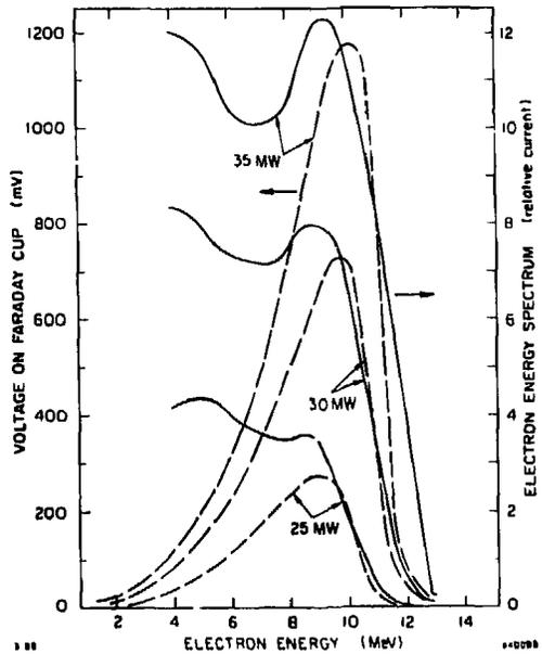
Fig. 15. Uncorrected (dashed lines) and corrected (continuous lines) electron energy spectra for various values of peak input power into S-band seven-cavity structure.
