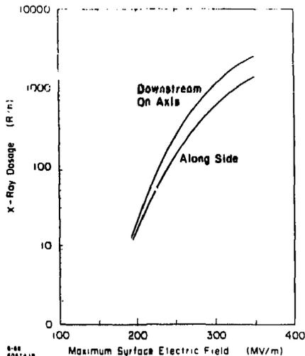
Fig. 17. Average x-ray dosage around S-band (two-cavity,  $\pi$ -mode) accelerator section ( $2.5 \mu\text{sec}$ , 60 pps) as a function of peak field.
