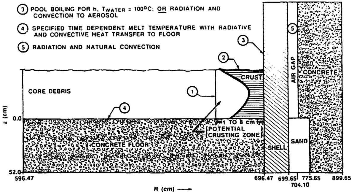
Fig. 1. Mark-1 Containment shell model for heatup analysis.
