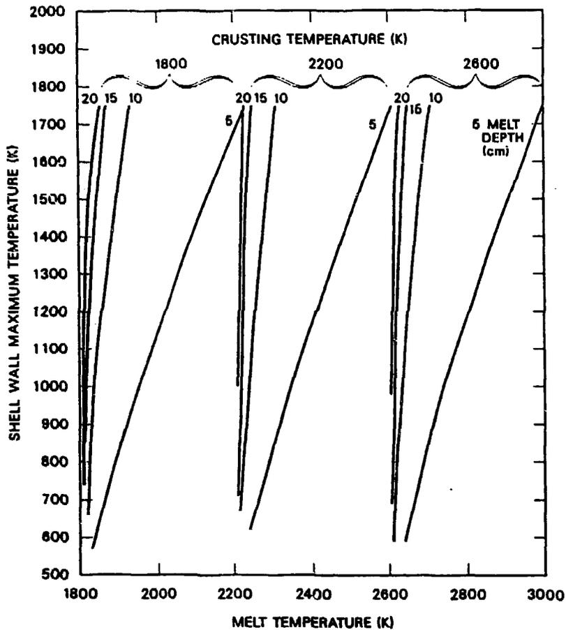
Fig. 9. Maximum shell temperature vs melt temperature as a function of crusting temperature and melt depth for a melt convective heat transfer coefficient of 5,000 (W/M<sup>2</sup>/K).
