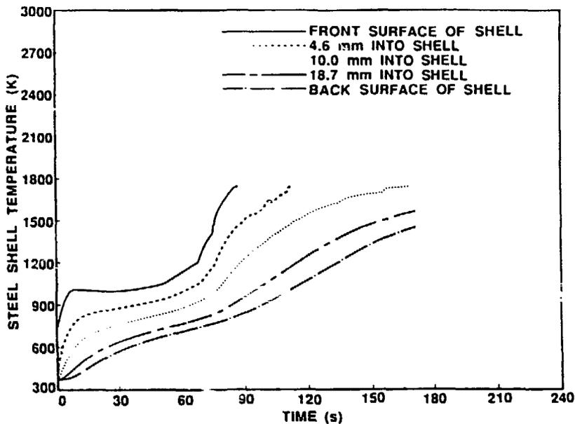
Fig. 4. Transient temperatures in containment shell (case 2).
