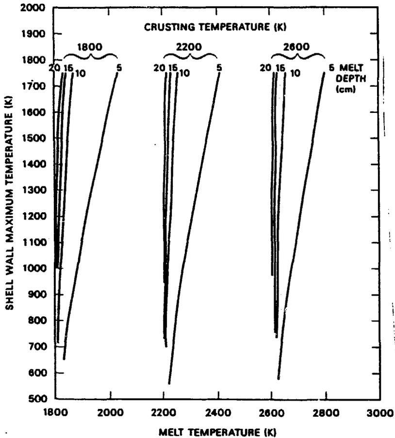
Fig. 8. Maximum shell temperature vs melt temperature as a function of crusting temperature and melt depth for a melt convective heat transfer coefficient of 10,000 ( $W/M^2-K$ ).
