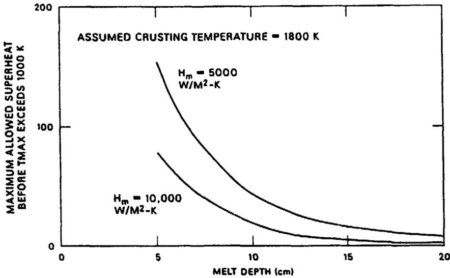
Fig. 10. Superheat (melt temperature – crusting temperature) above which the shell maximum temperature exceeds 1,000 K as a function of the melt depth and the melt-to-crust heat transfer coefficient.
