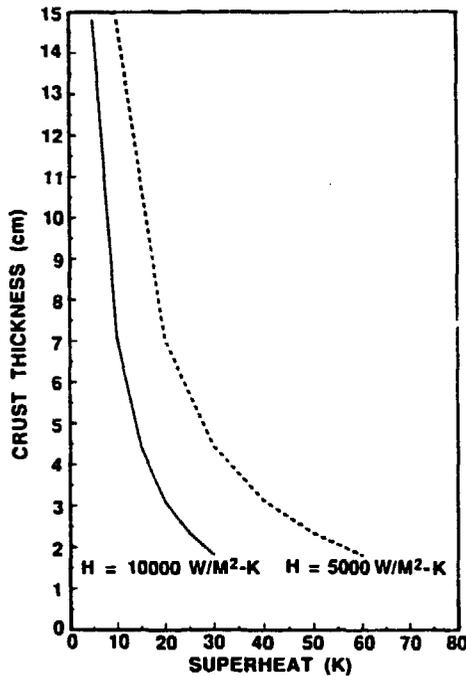
Fig. 11. Crust thickness vs superheat (melt temperature – crusting temperature), for a crusting temperature of 2,600 K, melt-to-crust heat transfer coefficients of 10,000 and 5,000 (W/M<sup>2</sup>-K), and melt depth of 15 cm.
