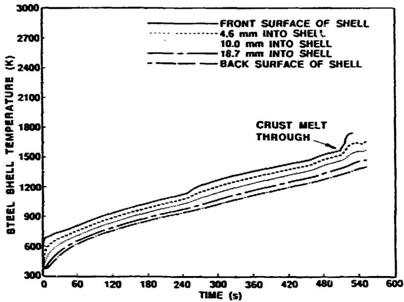
Fig. 5. Transient temperatures in containment shell (case 3).
