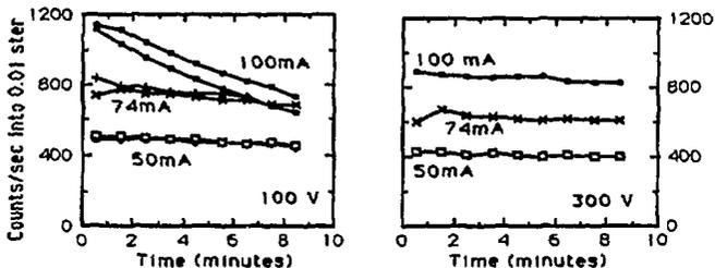
Fig. 6. Count rate vs time at high levels of cooling. Data taken at  $E=18\text{keV}$ ,  $n_e(\text{Ti})=1.3 \cdot 10^4\text{cm}^{-3}$  for  $V_A=100\text{V}$ ,  $V_A=300\text{V}$ . that ignore ion space charge cannot explain it. Also there is a noticeable decay ( $1/e$  lifetime = 18 min) at  $V_A=100\text{V}$  and  $I=100\text{mA}$ .
