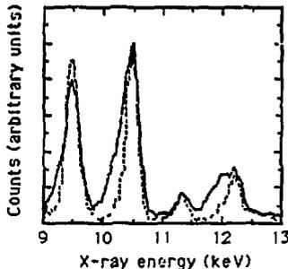
Fig.1.  $N=3 \rightarrow 2$  transition lines in near neon-like Au HCIs taken with a solid-state Ge detector.  $E=18\text{keV}$ ,  $I=100\text{mA}$ . Solid: no evaporative cooling,  $V_{\text{trap}}=80\text{V}$ . Dash: evaporative cooling (Ti ions),  $V_{\text{trap}}=40\text{V}$ . The narrower lines with cooling indicate a narrower charge state distribution.
