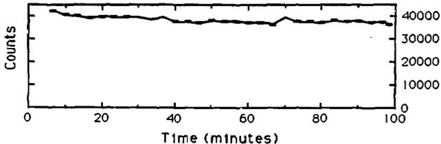
Fig.3. Count rate in  $n=3 \rightarrow 2$  transition lines vs. time. Gold is injected into the trap at 0 minutes. The estimated  $1/e$  trap lifetime is about 4 hrs. Ti shutter is always open.
