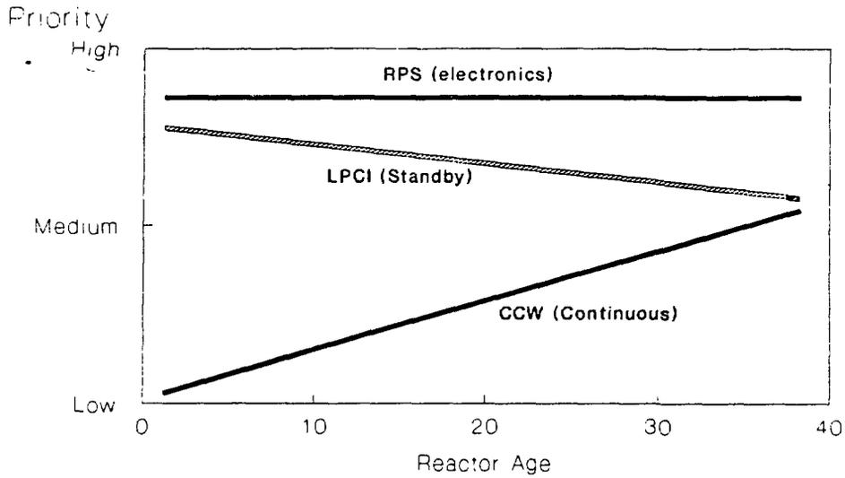
Figure 2 Potential Prioritization of System Inspections Based on NPAR Input
