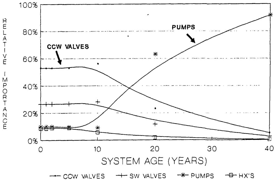
Figure 3 Inspection Importance of Components Within a System
