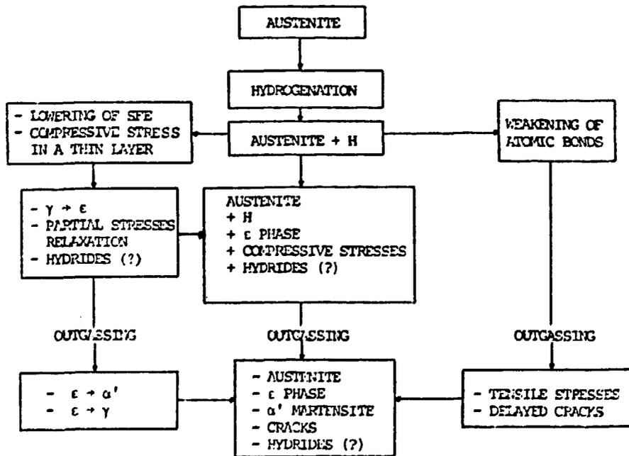
Figure 12 Schematic diagram of the phenomena occurring during hydrogenation and outgassing of an unstable austenitic stainless steel
