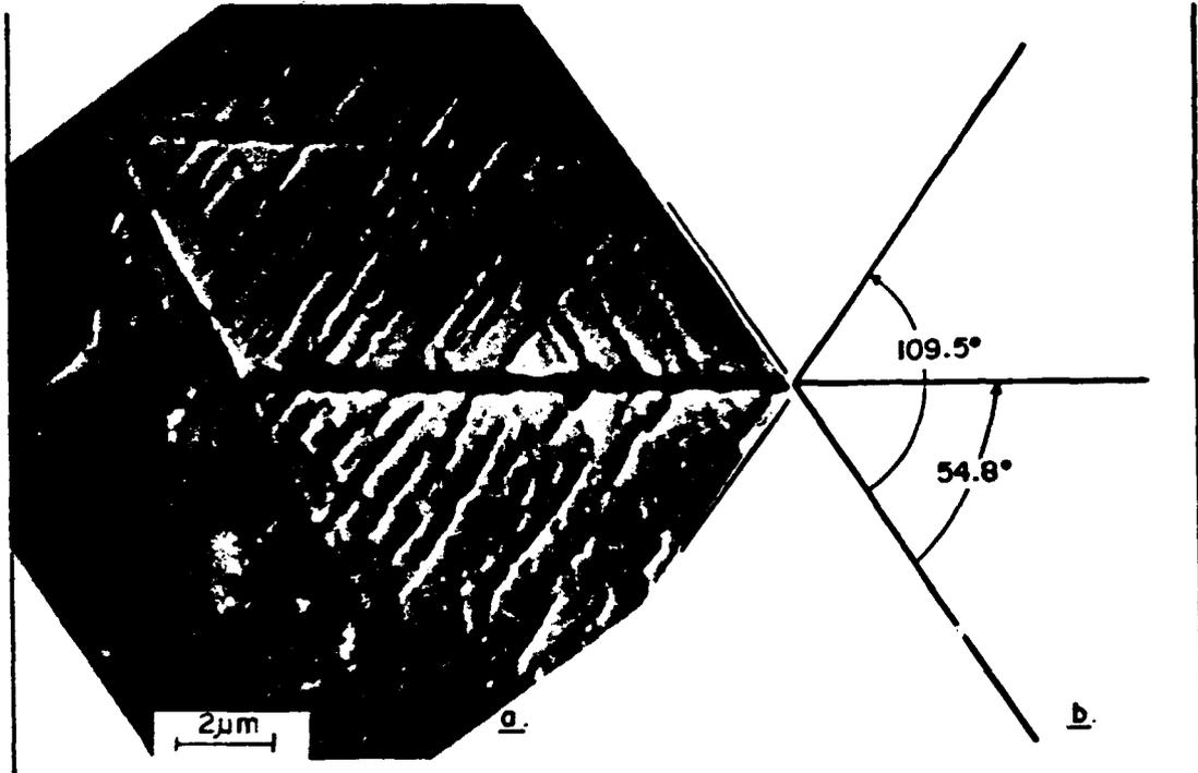
Figure 2 - a. SEM Micrograph of sample charged at  $2000 \text{ A/m}^2$  for 2 h.  $\epsilon$  phase at a twin. Etched with aqua regia. b. Angles between traces of planes  $(111)_\gamma$  ( $\epsilon$  phase) and the crack (ref. 4)
