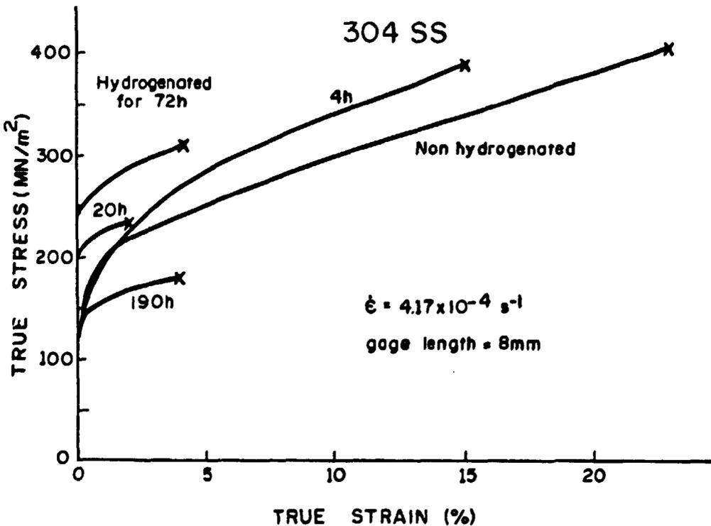
Figure 6 True stress - true strain curves for sheet specimens annealed and hydrogenated with 2000A/m<sup>2</sup> for the specified times.
