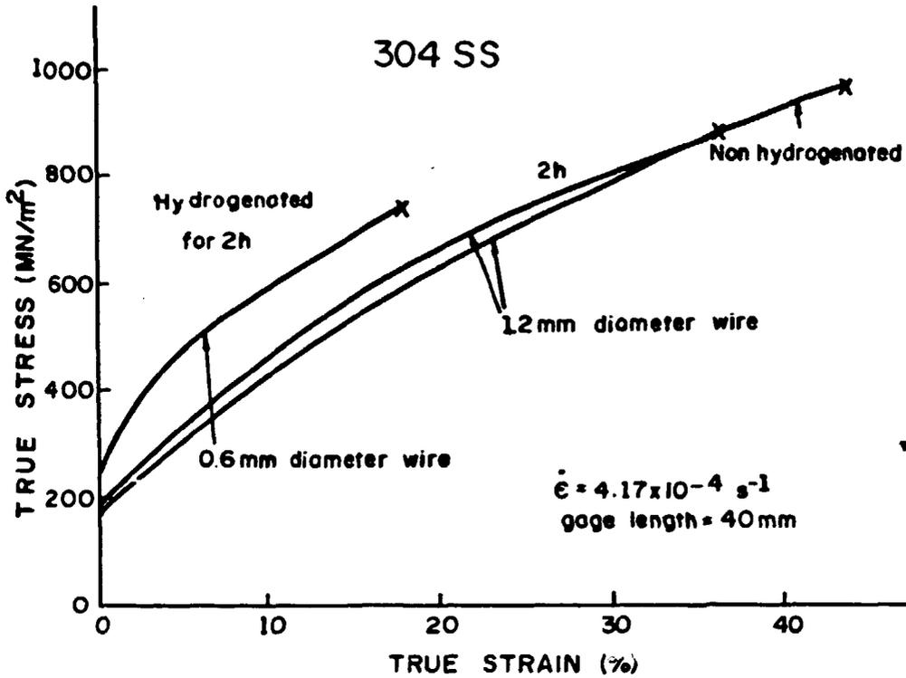
Figure 5 True stress - True strain curves for wire specimens annealed and hydrogenated with 1000A/m<sup>2</sup> for the specified times.
