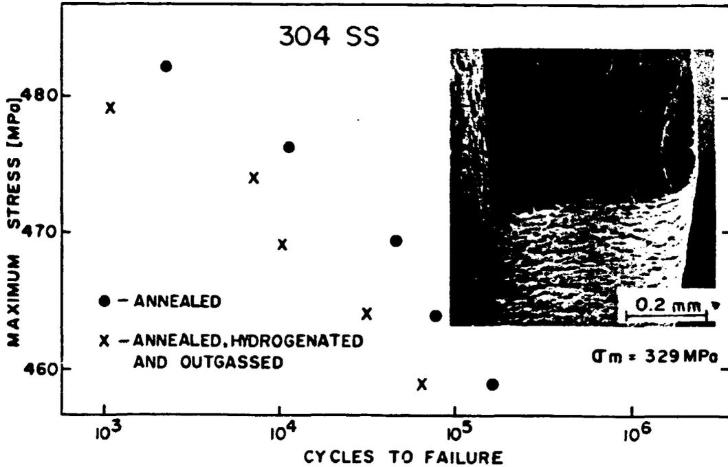
Figure 11 Fatigue life of annealed and hydrogenated samples. Insert shows typical lateral surface and fracture morphology appearance after testing
