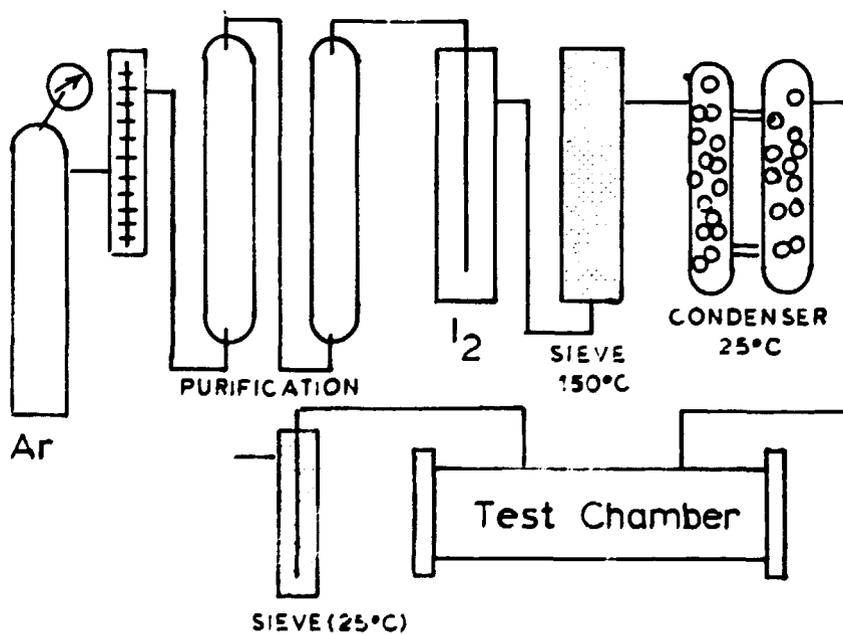
Figure 1 Diagram of the flowing gas (Ar + 40Pa I<sub>2</sub>) system
