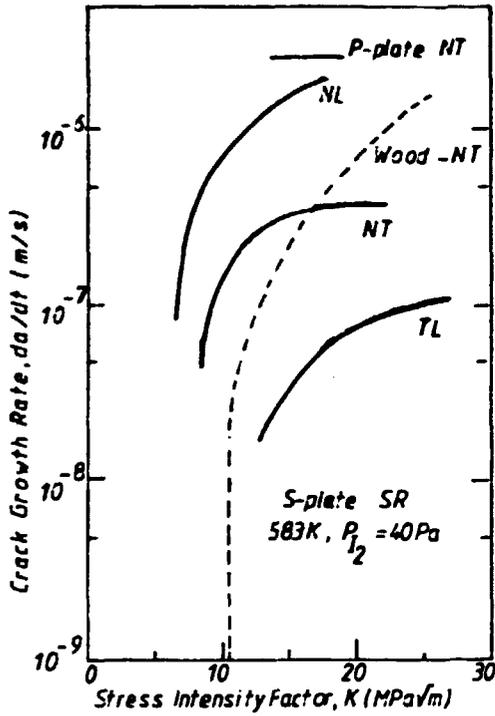
Figure 2 da/dt vs K behavior at 583K
