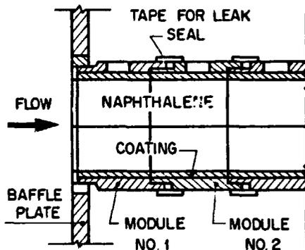
Figure 2. The test section
