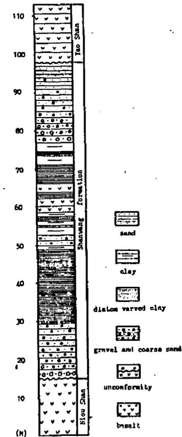
Fig.1. Columnar section of Shanwang area.
