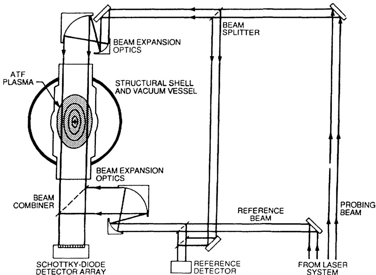
Fig. 1. Schematic of the 15-channel FIR interferometer system on ATF.
