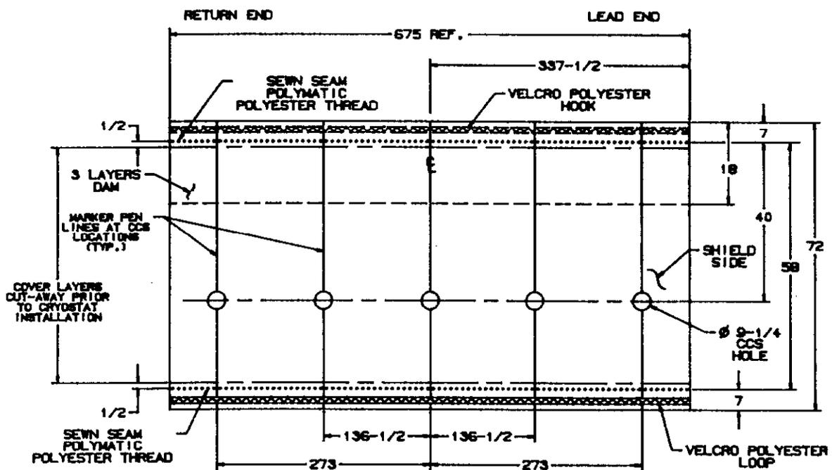
Fig. 3. SSC Dipole Magnet 80K Inner Blanket
