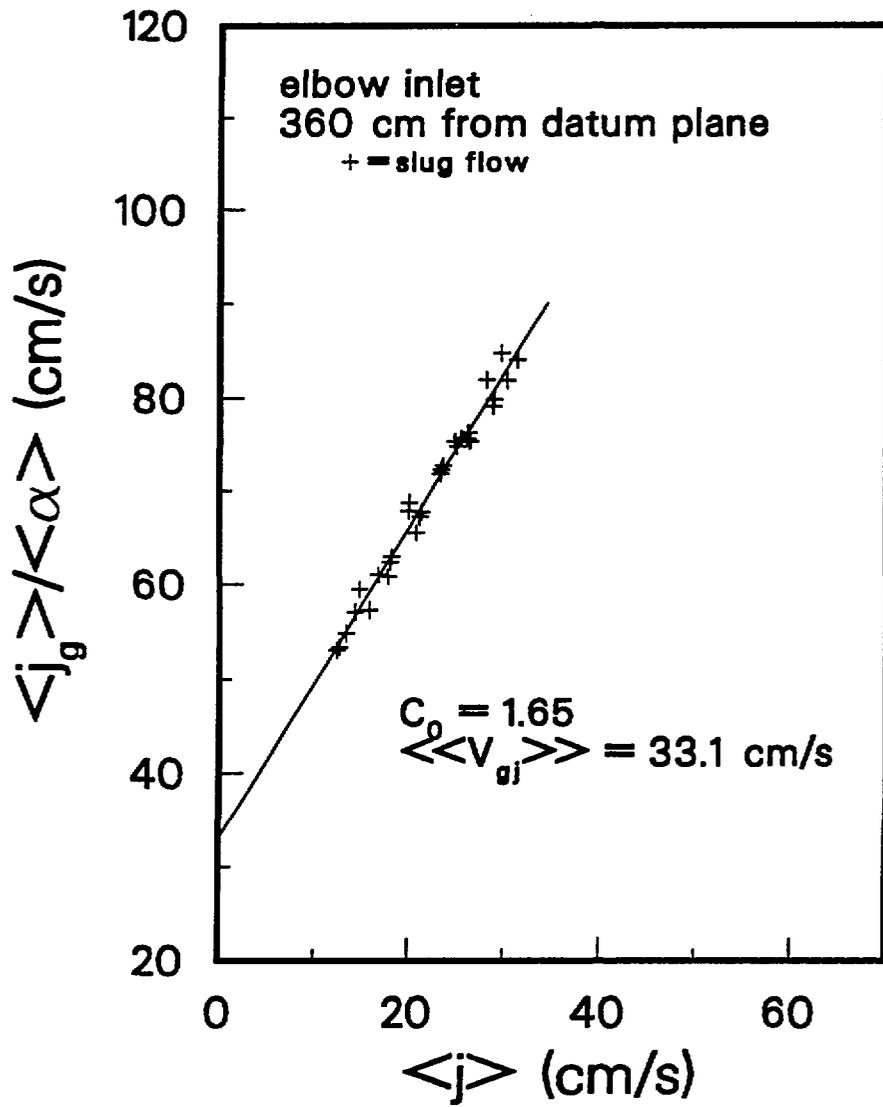
Fig. 17. -  $\langle j_g \rangle / \langle \alpha \rangle$  vs.  $\langle j \rangle$ . Elbow Inlet, 360 cm from Datum Plane.
