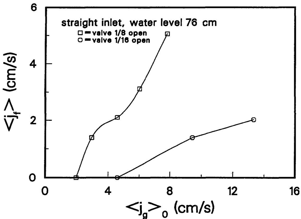
Fig. 6. - Induced Liquid Volumetric Flux vs. Gas Volumetric Flux. Straight Inlet, Separator Water Level 76 cm.
