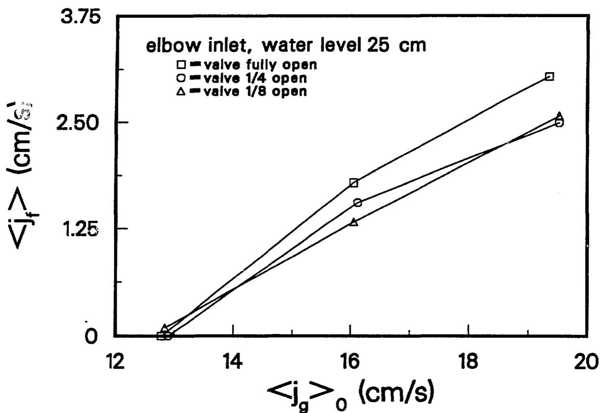
Fig. 7. - Induced Liquid Volumetric Flux vs. Gas Volumetric Flux. Elbow Inlet, Separator Water Level 25 cm.
