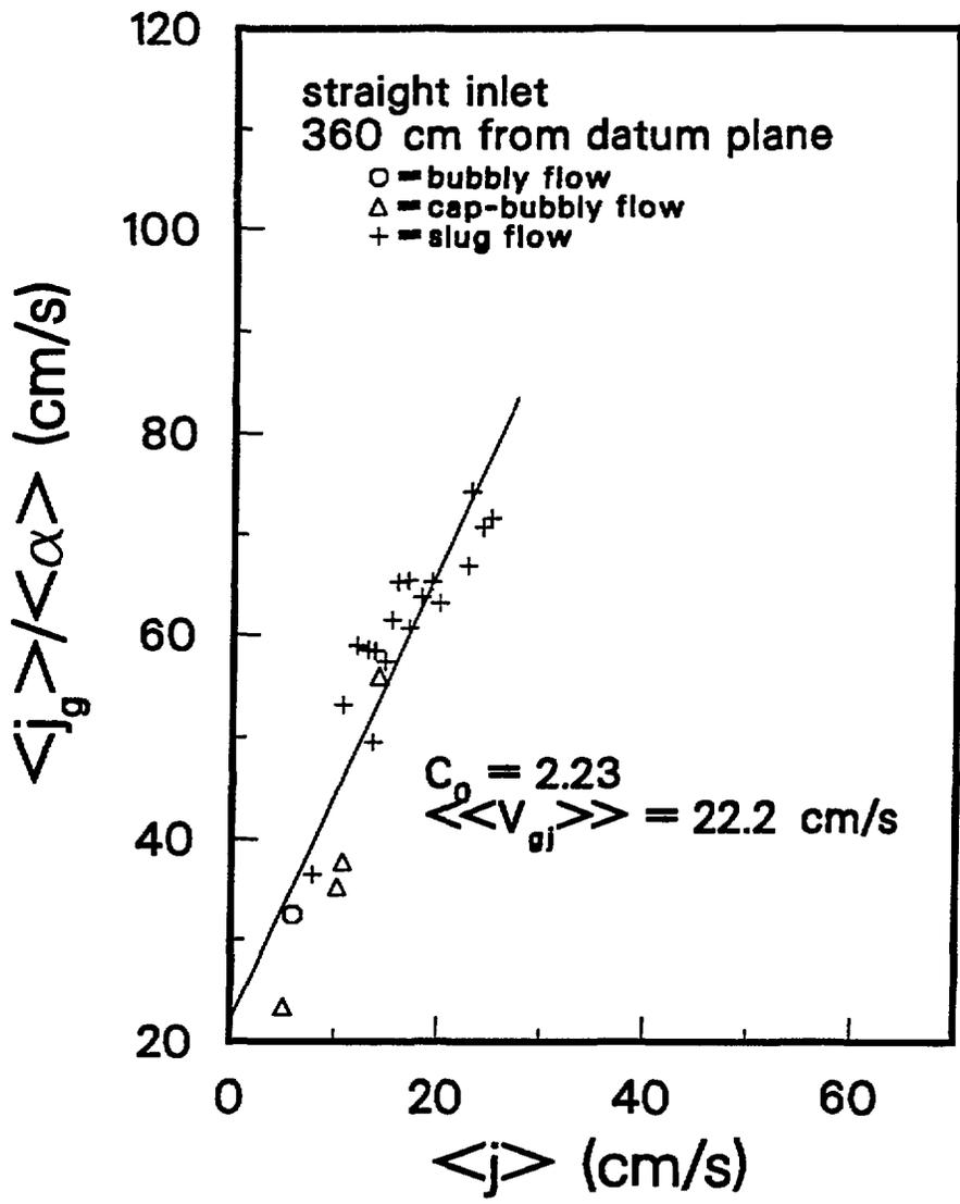
Fig. 14. -  $\langle j_g \rangle / \langle \alpha \rangle$  vs.  $\langle j \rangle$ . Straight Inlet, 360 cm from Datum Plane.
