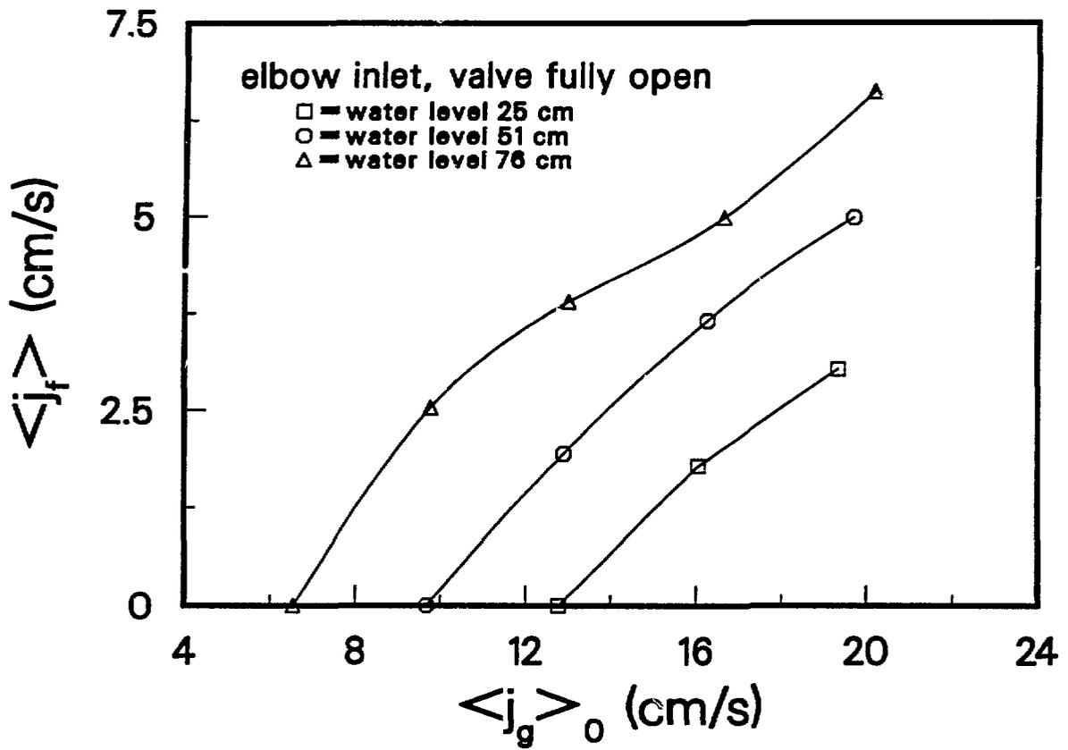
Fig. 4. - Induced Liquid Volumetric Flux vs. Gas Volumetric Flux. Elbow Inlet, Friction-Loss Control Valve Fully Open.
