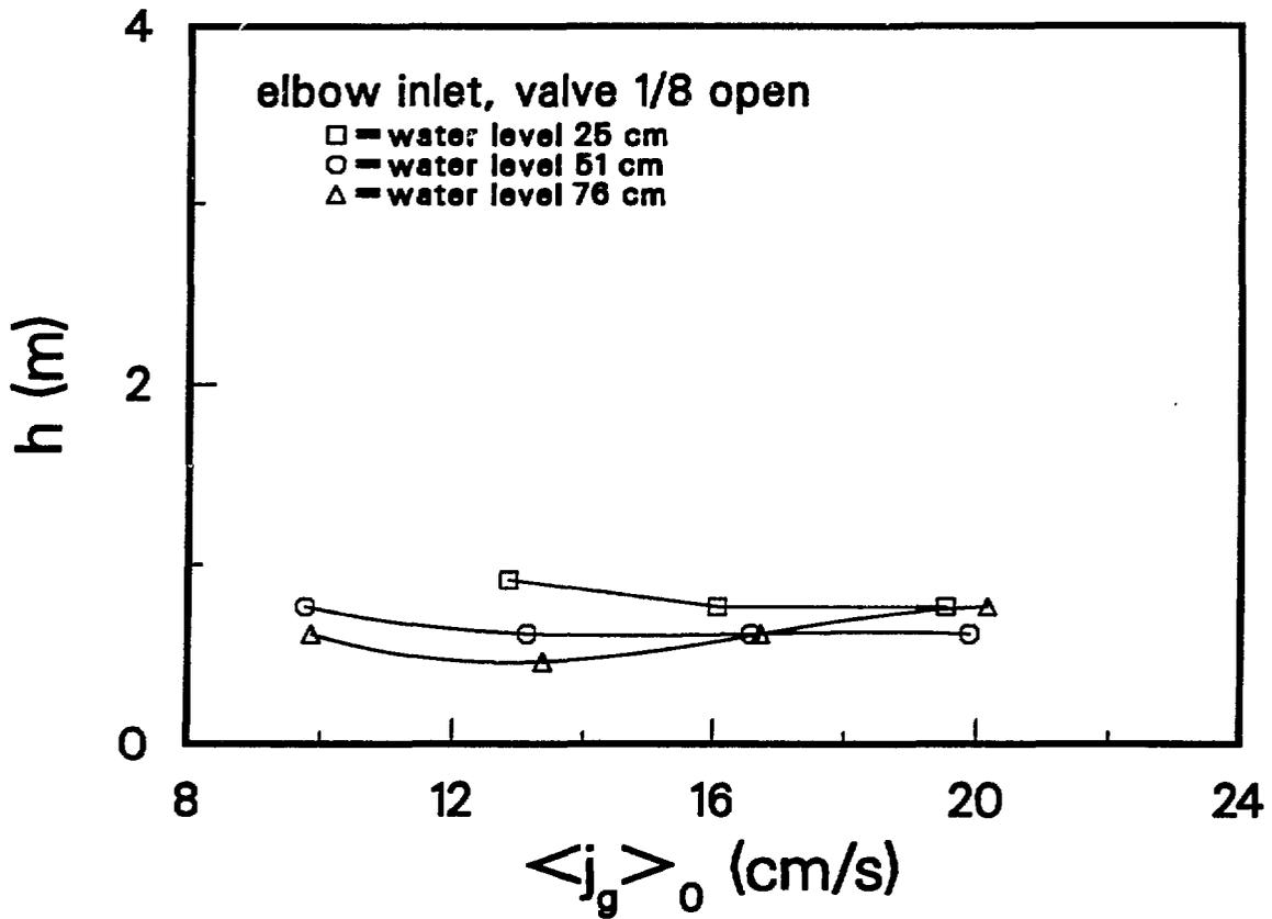
Fig. 9. - Location of Flow-Pattern Transition from Cap-Bubbly Flow to Slug Flow vs. Gas Volumetric Flux. Elbow Inlet, Friction-Loss Control Valve 1/8 Open.
