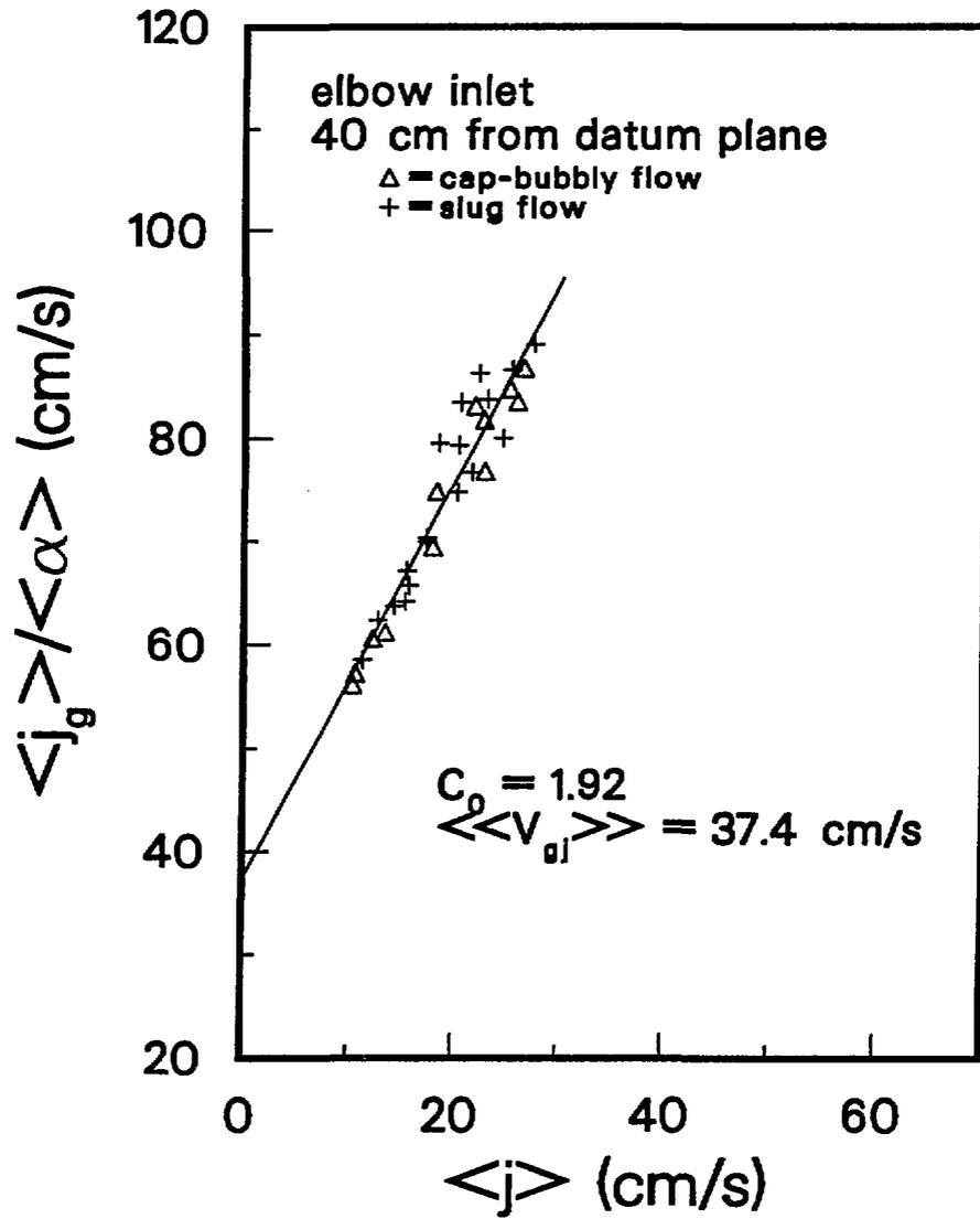
Fig. 15. -  $\langle j_g \rangle / \langle \alpha \rangle$  vs.  $\langle j \rangle$ . Elbow Inlet, 40 cm from Datum Plane.
