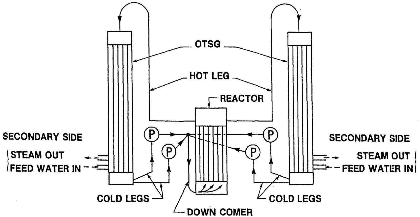
Fig. 1. - Schematic of Babcock and Wilcox Nuclear Reactor System.
