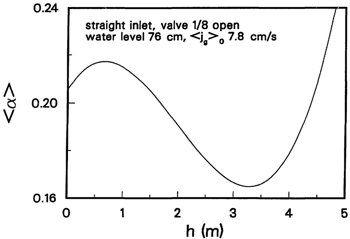
Fig. 11. - Void Fraction as a Function of Length Along the Riser Section. Straight Inlet, Friction-Loss Control Valve 1/8 Open, Separator Water Level 76 cm.
