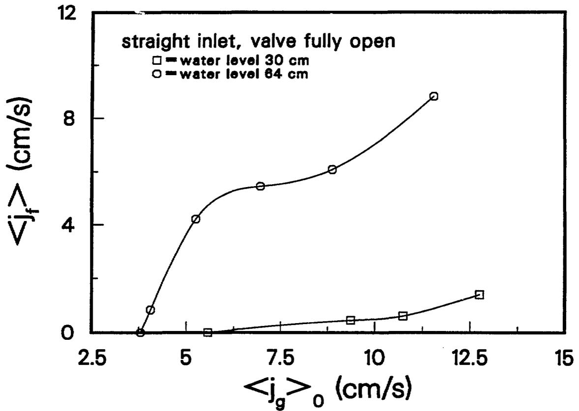
Fig. 3. - Induced Liquid Volumetric Flux vs. Gas Volumetric Flux. Straight Inlet, Friction-Loss Control Valve Fully Open.
