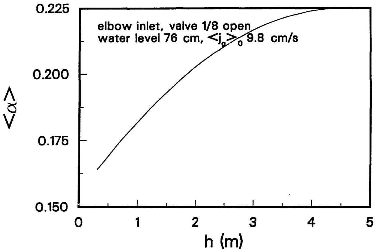
Fig. 12. - Void Fraction as a Function of Length Along the Riser Section. Elbow Inlet, Friction-Loss Control Valve 1/8 Open, Separator Water Level 76 cm.
