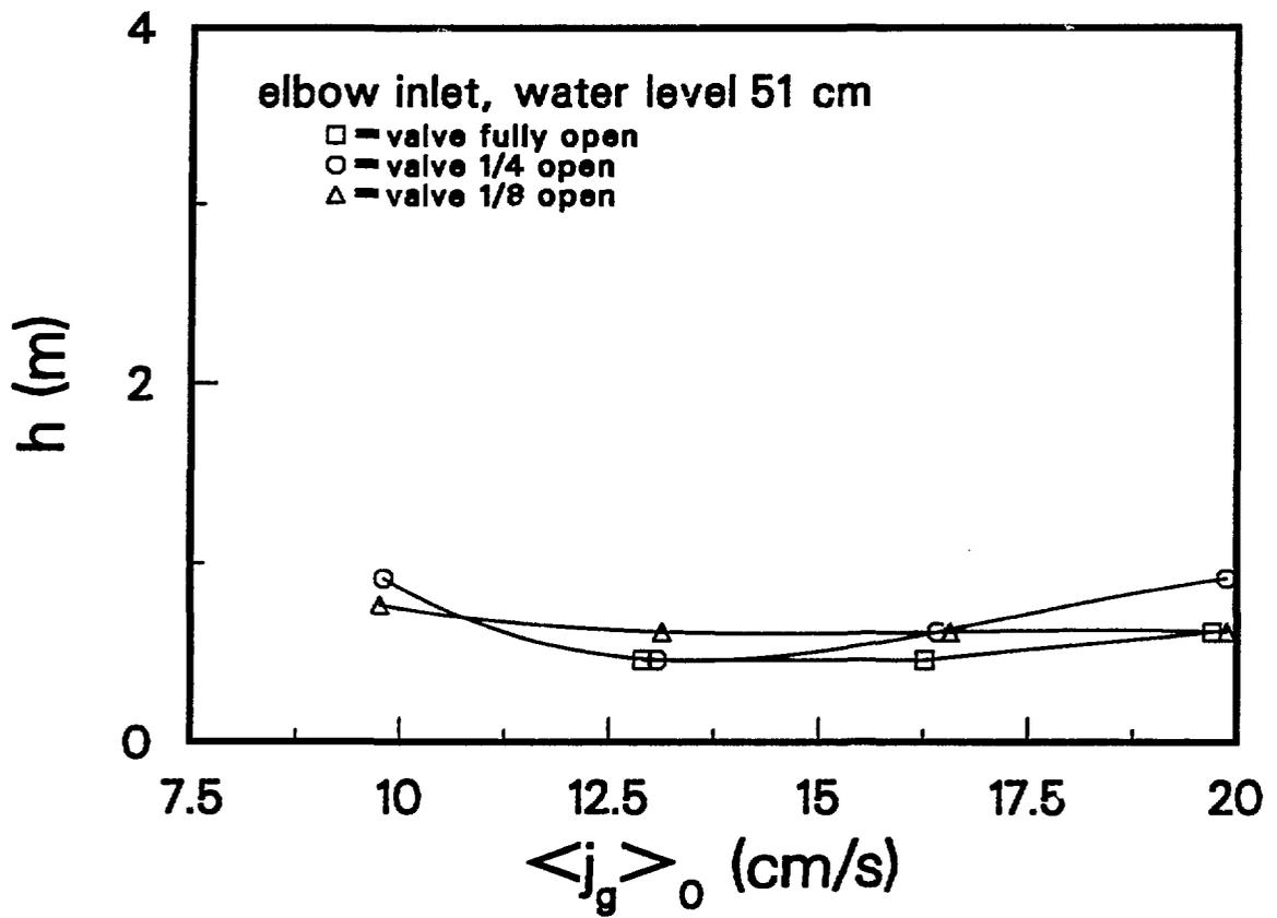
Fig. 10. - Location of Flow-Pattern Transition from Cap-Bubbly Flow to Slug Flow vs. Gas Volumetric Flux. Elbow Inlet, Separator Water Level 51 cm.
