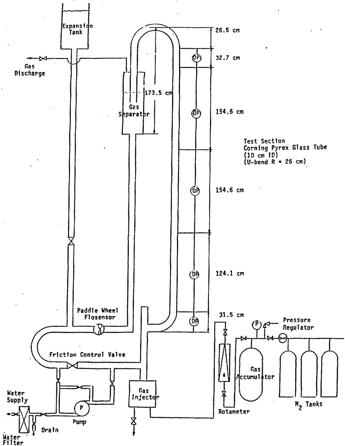
Fig. 2. - Schematic of the Experimental Setup.
