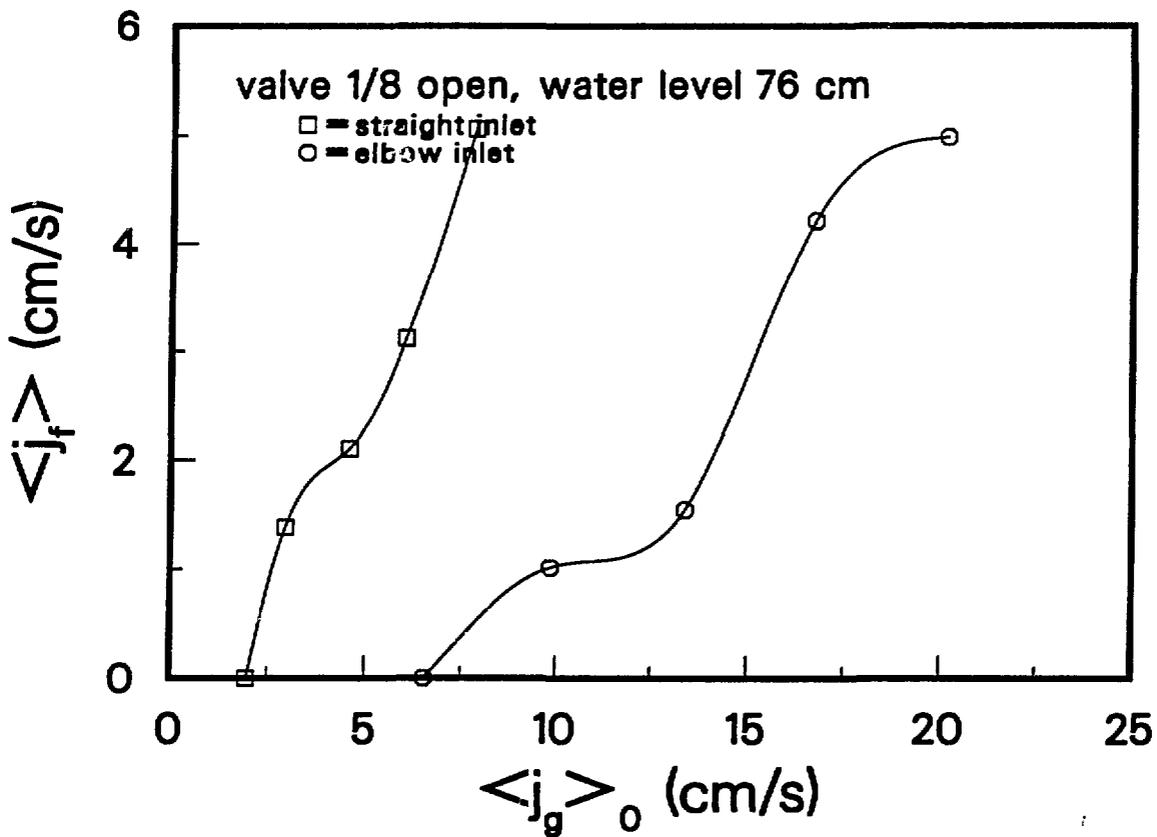
Fig. 8. - Induced Liquid Volumetric Flux vs. Gas Volumetric Flux. Friction-Loss Control Valve 1/8 Open, Separator Water Level 76 cm.
