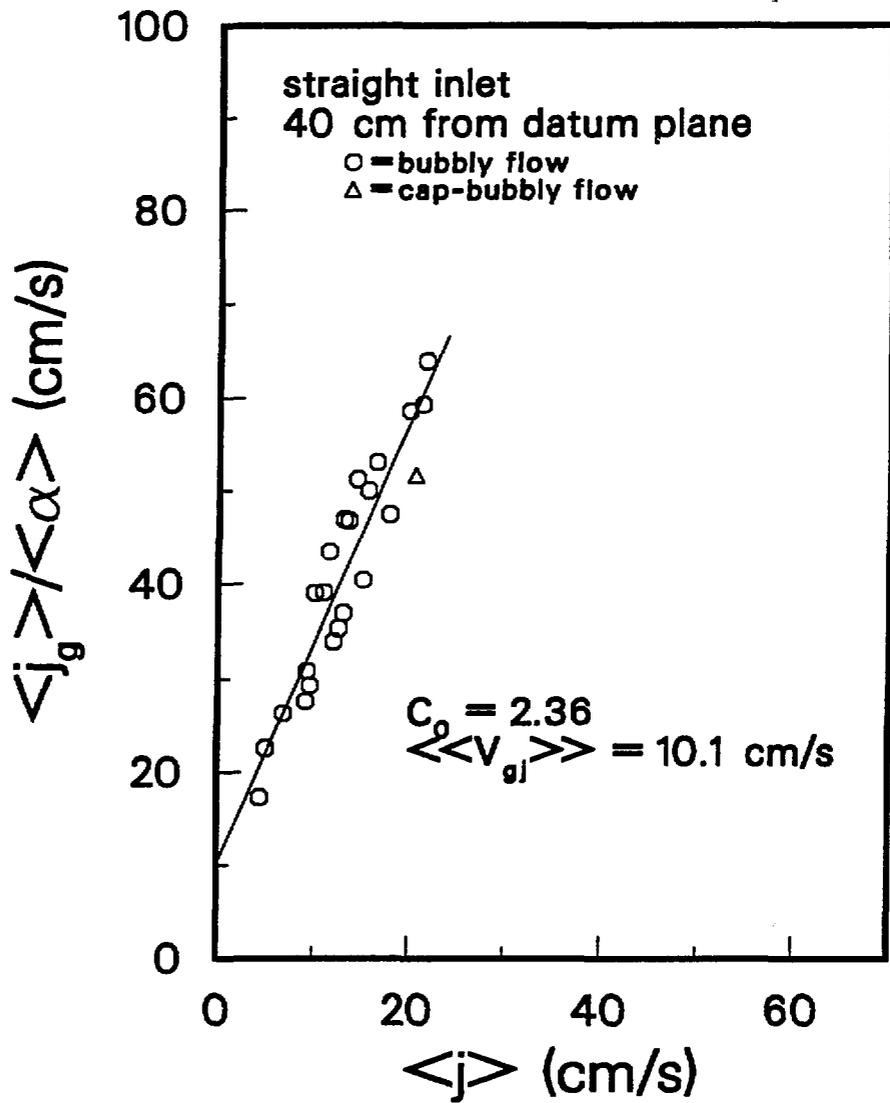
Fig. 13. -  $\langle j_g \rangle / \langle \alpha \rangle$  vs.  $\langle j \rangle$ . Straight Inlet, 40 cm from Datum Plane.
