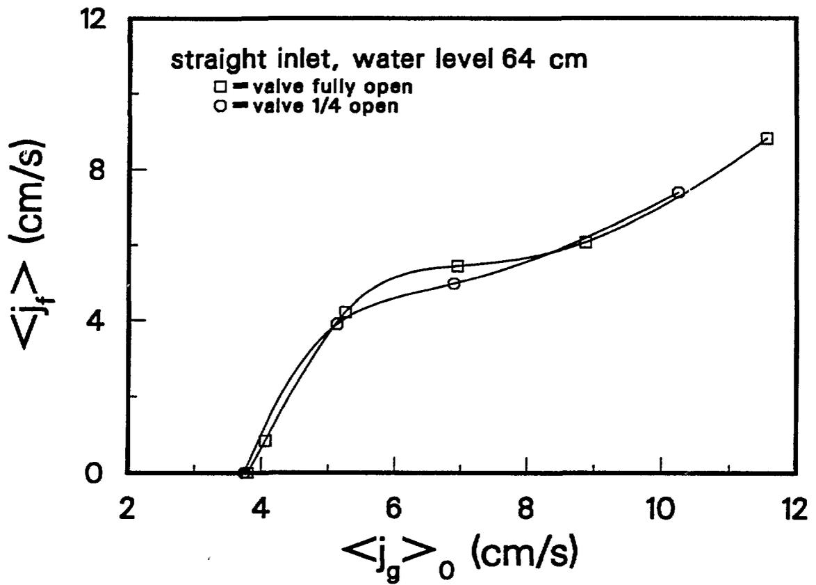
Fig. 5. - Induced Liquid Volumetric Flux vs. Gas Volumetric Flux.
