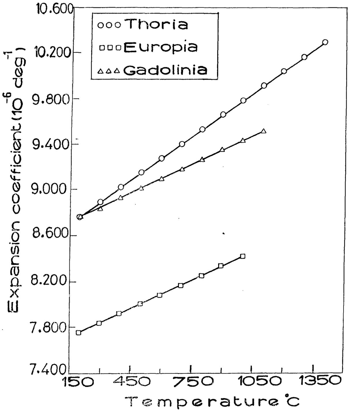
Fig.9 Measured expansion coefficient of thoria, europia, and gadolinia as a function of temperature
