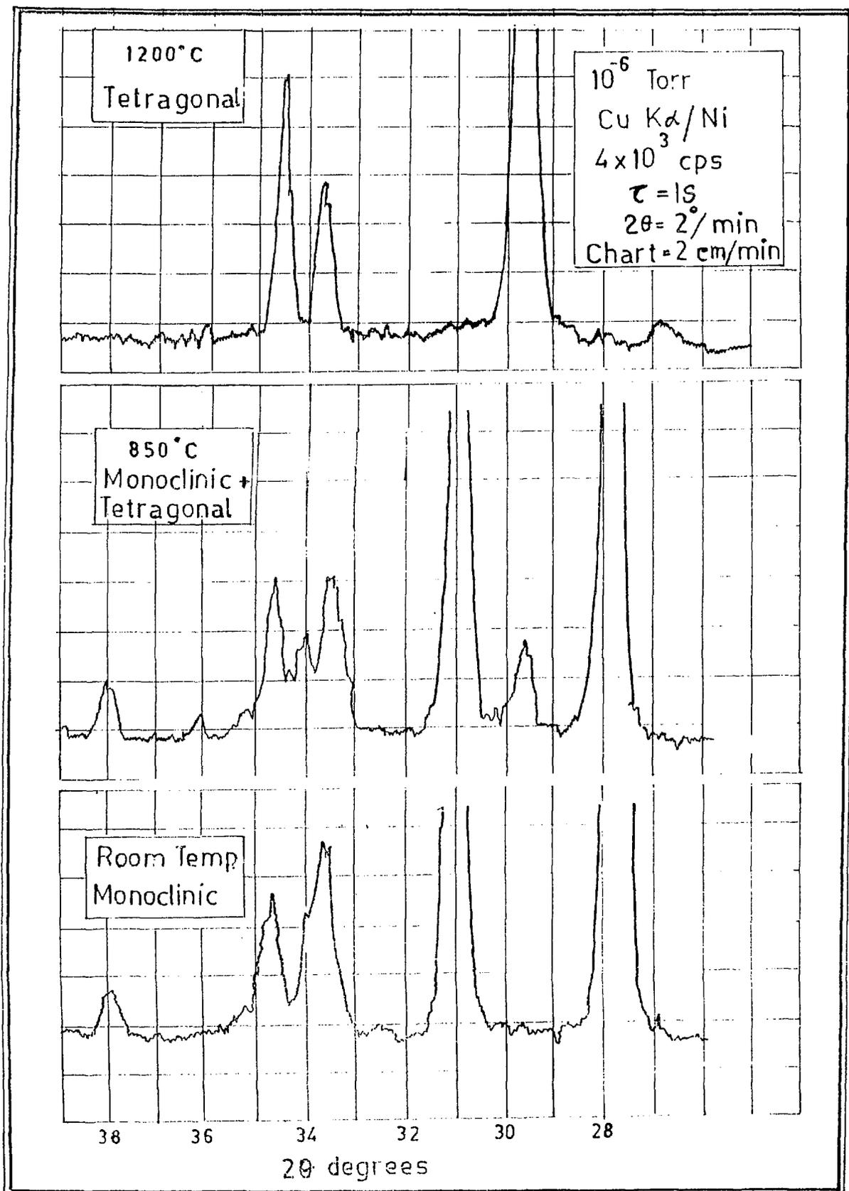
Fig.5 Diffraction pattern of zirconia before, during and after phase transformation
