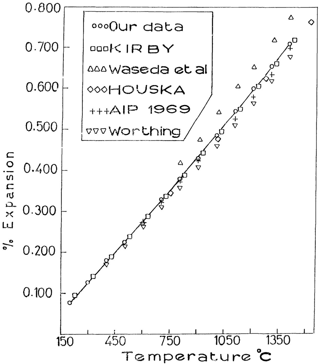
Fig.7 Measured % expansion of tungsten versus temperature as compared with the reported values
