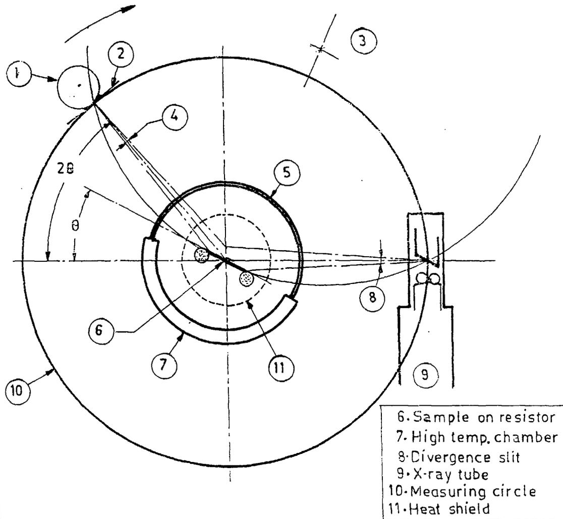
Fig.1 X-ray diffraction geometry incorporating the high temperature attachment.
