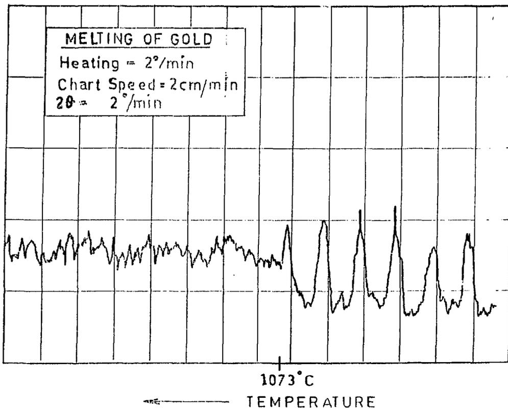
Fig.4 A diffraction peak of gold at the temperature of melting
