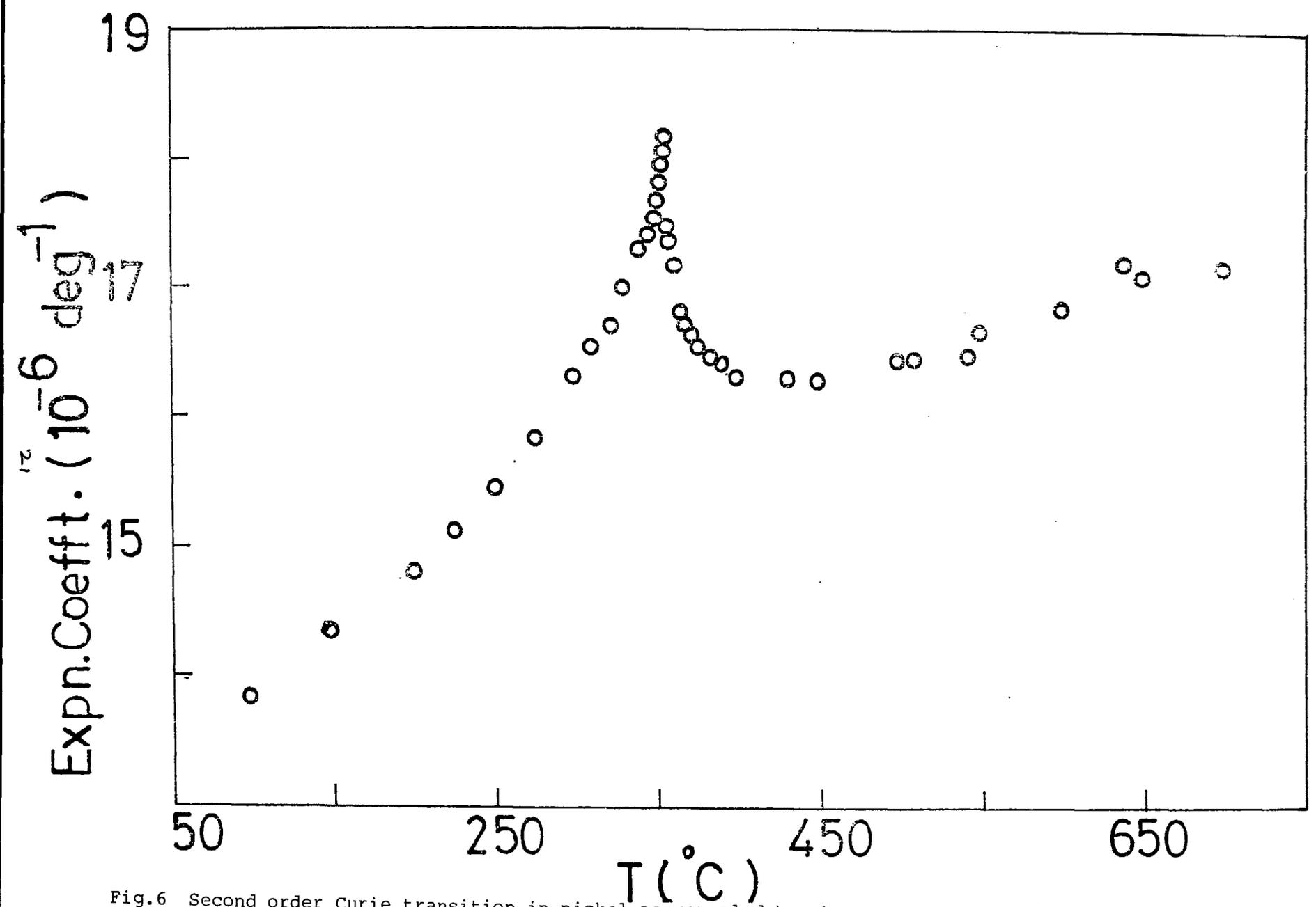
Fig.6 Second order Curie transition in nickel as revealed by the anomalous variation of thermal expansion coefficient with temperature
