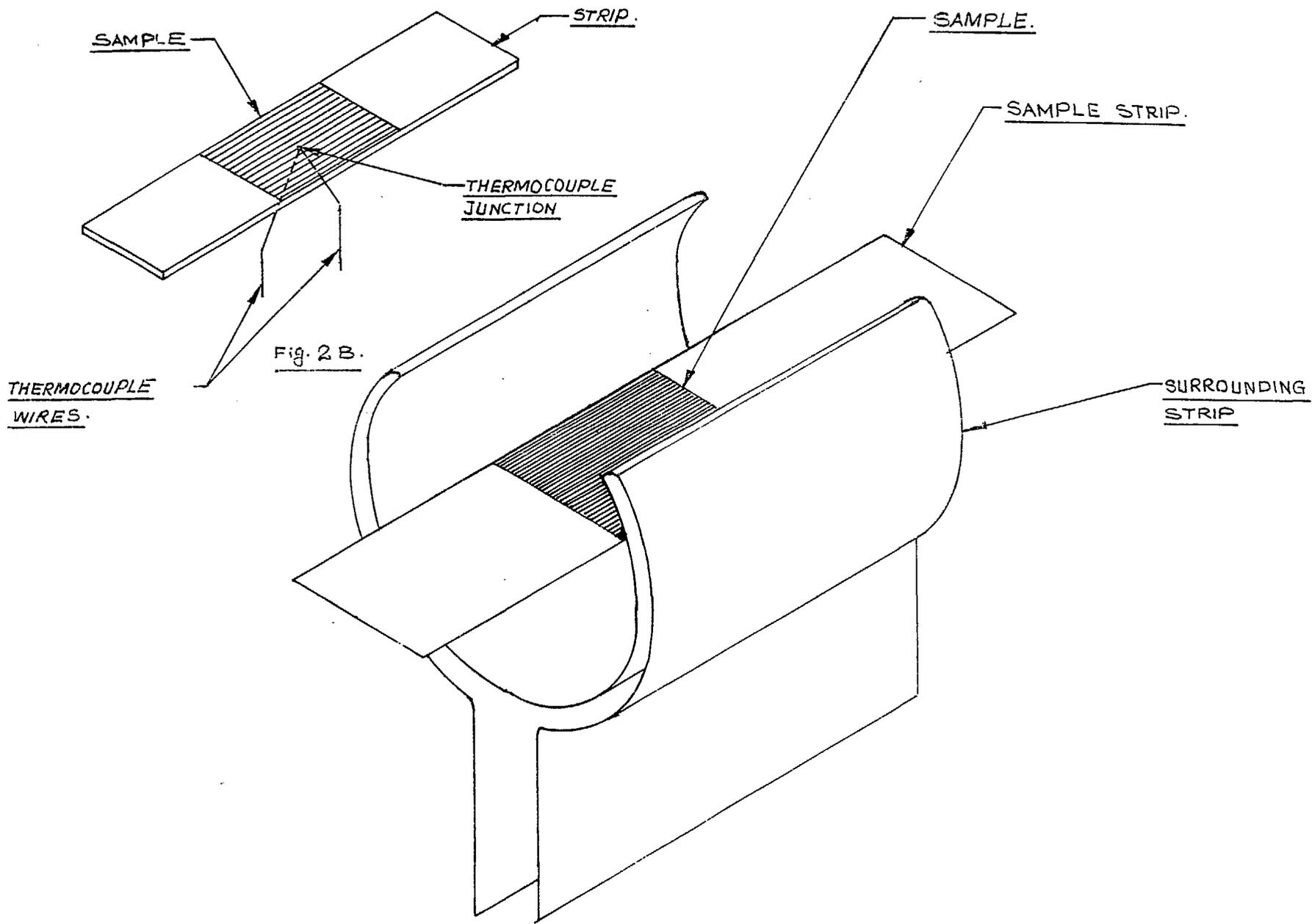
Fig.2 The arrangement of sample strip and surrounding heaters
