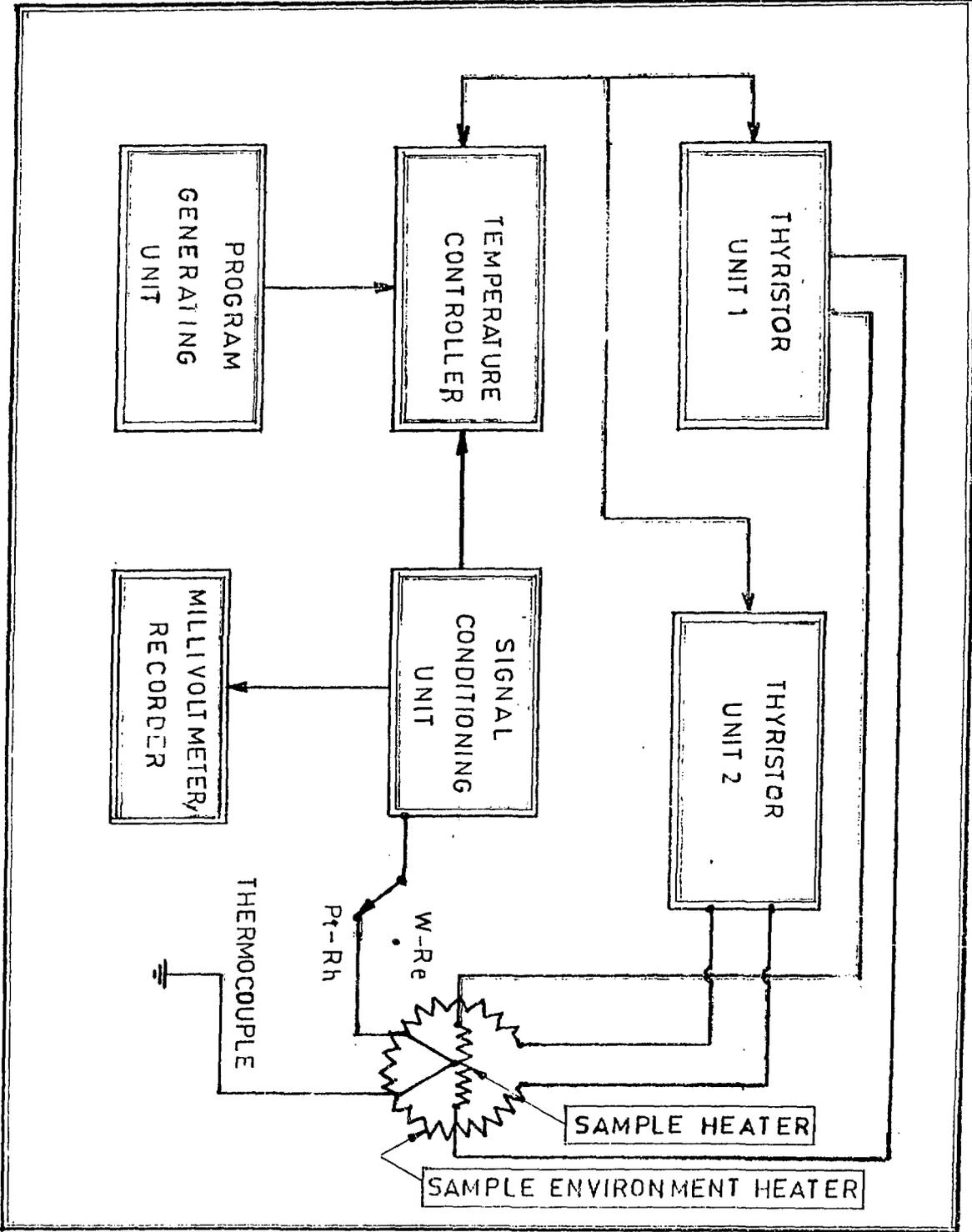
Fig. 3 Schematics of the temperature controller unit
