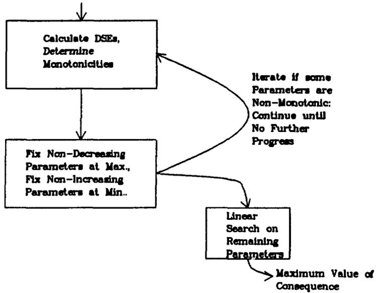
FIGURE 5: Procedure to Determine Maximum Value of Consequence
