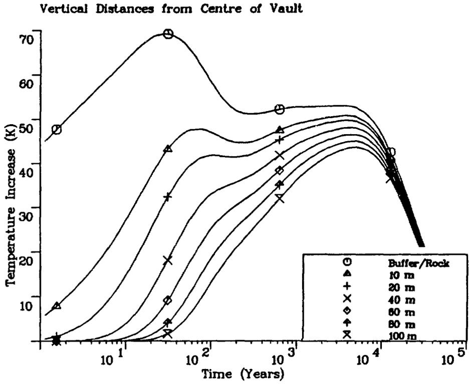
FIGURE 1: Temperature Profiles above Centre of the Vault
