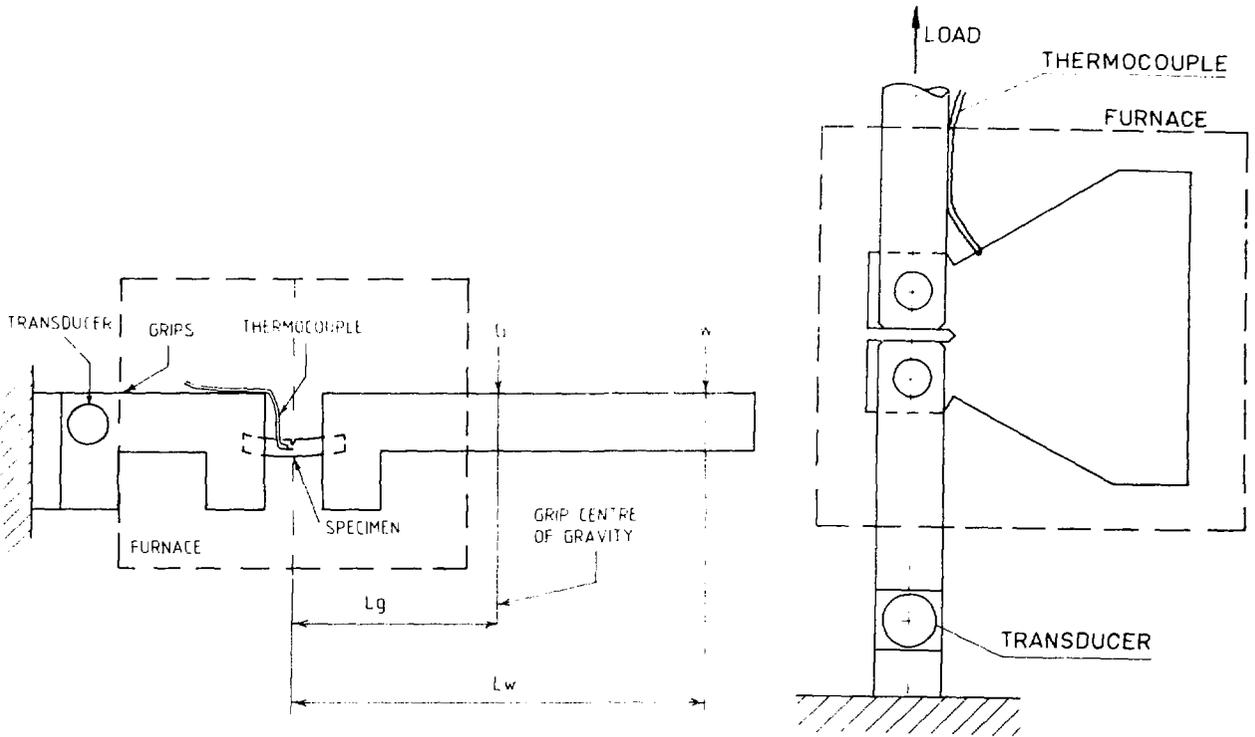
Figure 1: Schematic diagram of test set-ups in DHC testing using cantilever beam (left) and double cantilever beam specimens (right).
