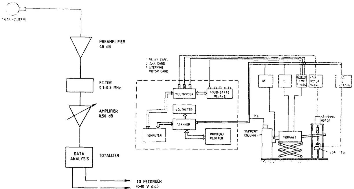
Figure 4: Schematic Diagram of the AE apparatus and the computerized DHC Rig.
