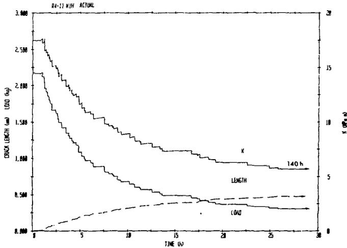
Figure 6: Measurement of the threshold stress intensity factor using AE to control the applied load. Every time the crack extended 0.005 mm, the load was reduced by 2% until cracking stopped. The corresponding  $K_I$  of  $5.7 \text{ MPa}\sqrt{\text{m}}$  is the threshold stress intensity factor.
