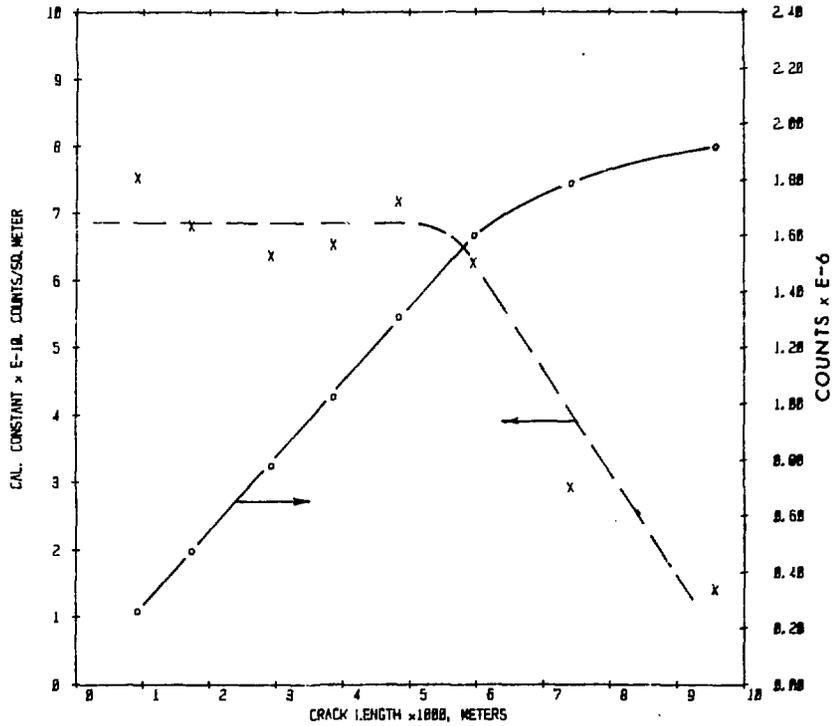
Figure 3: Calibration constant and cumulative counts as a function of crack length from Table 1.
