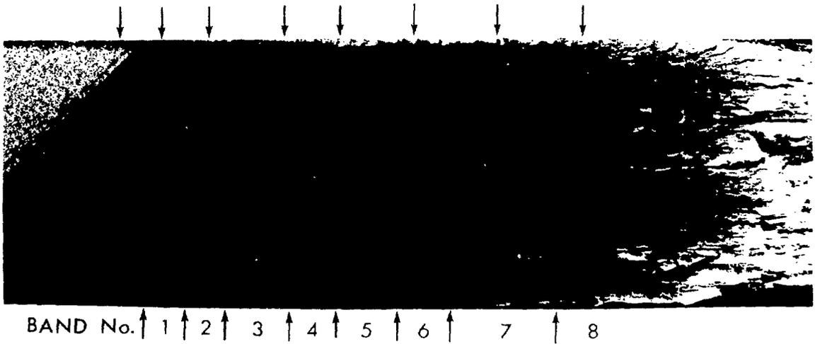
Figure 2: Fracture surface of a Zr-2.5 Nb double cantilever beam specimen after a series of eight, nominally identical crack velocity tests at 475 K and  $K_I$  of 15 MPa/ $\sqrt{m}$ .
