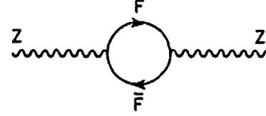
Fig. 5. Contributions of  $\mathcal{O}(G_F m_i^2)$  to the  $Z$  boson propagator
