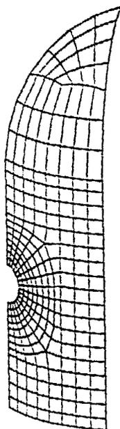
Figure 1. Three-Dimensional Containment Model (PRENEP)
