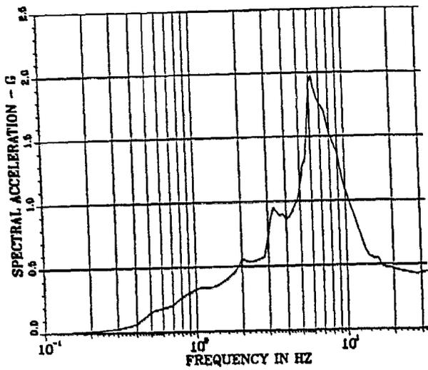
Fig. 7. Calculated Floor Spectrum
