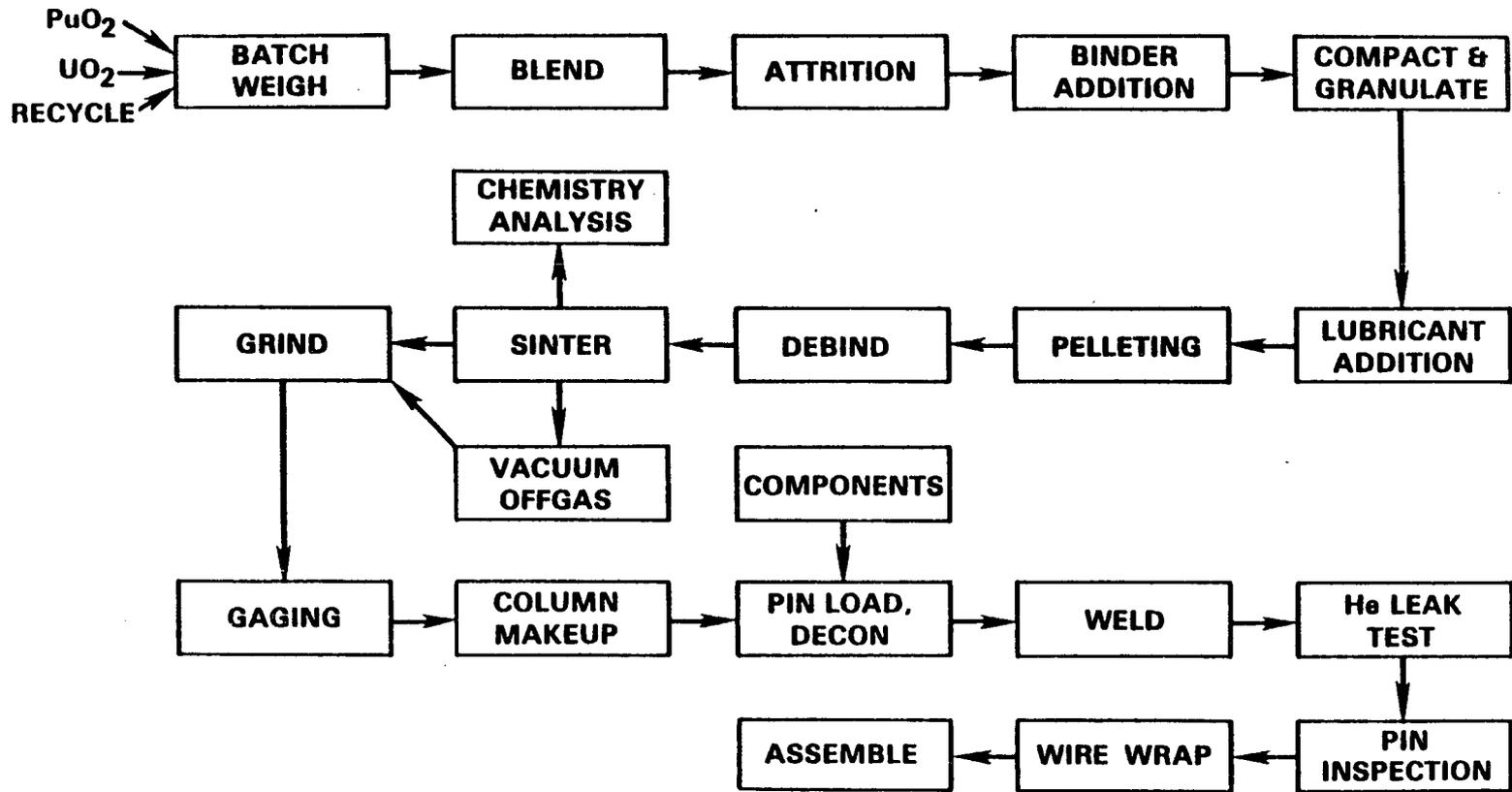
Figure 1: SAF Process Flow Diagram
