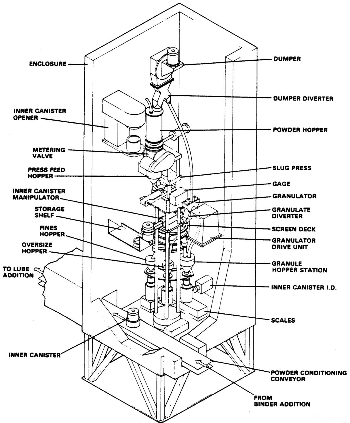
Figure 4: Compaction and Granulation
