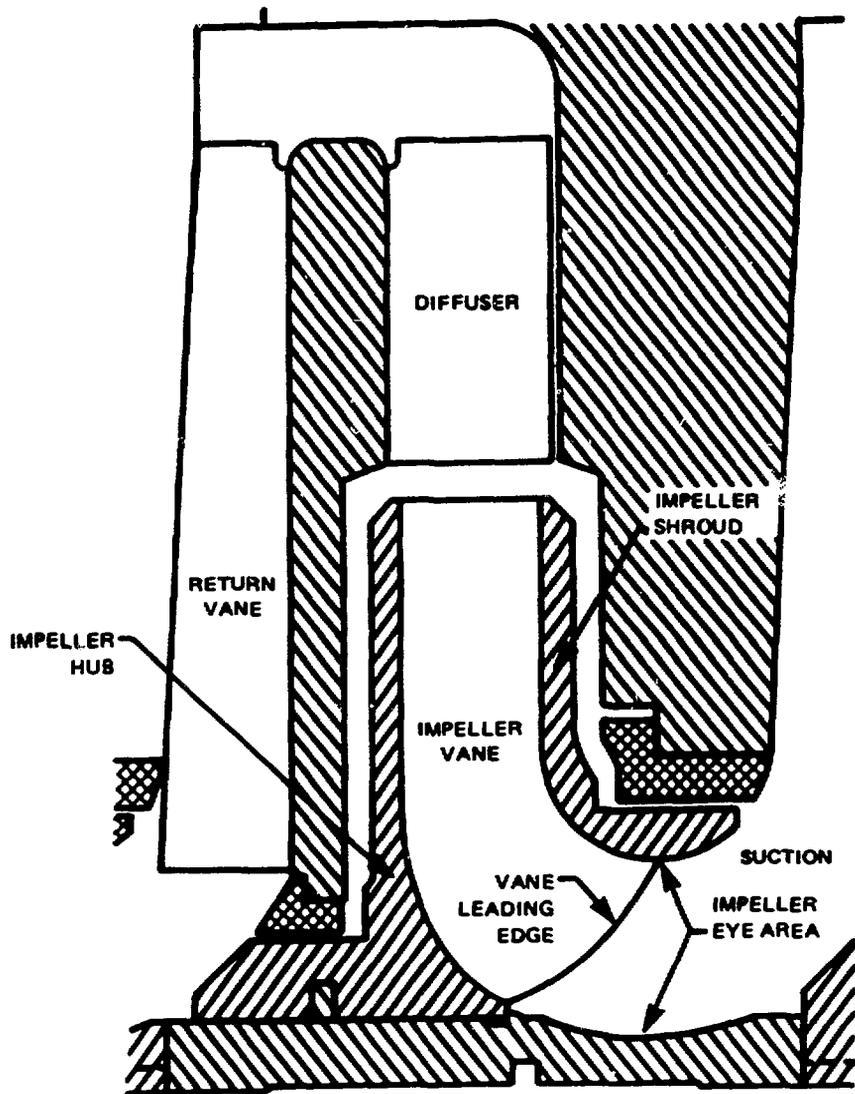
Fig. 1. Pump stage terminology (diffuser-type discharge chamber).
