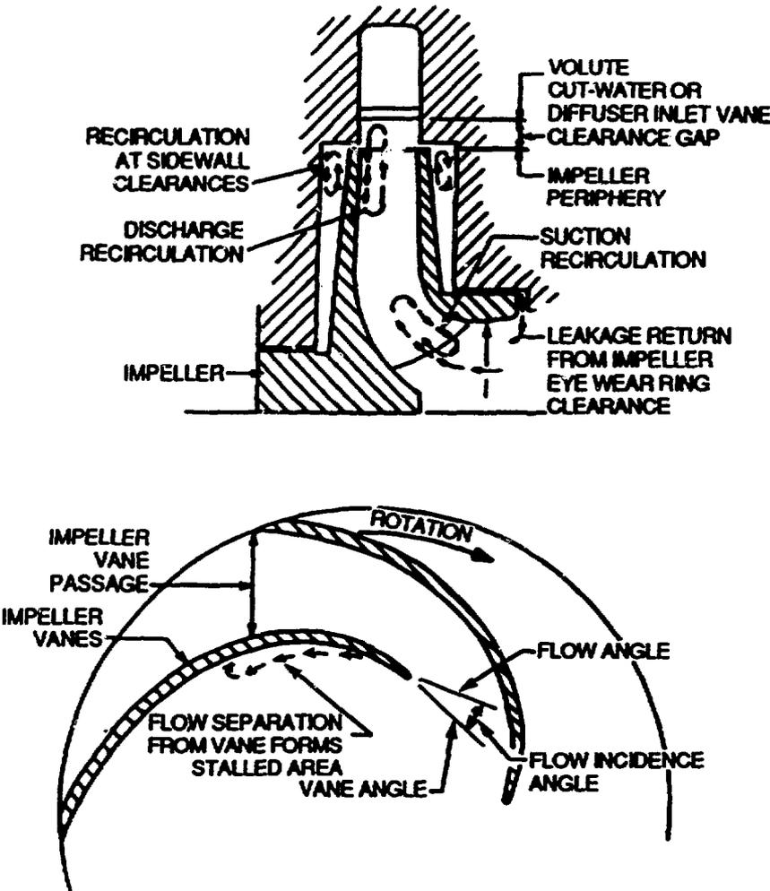
Fig. 2. Hydraulic instability flow phenomena. Redrawn with permission after Ref. 7.
