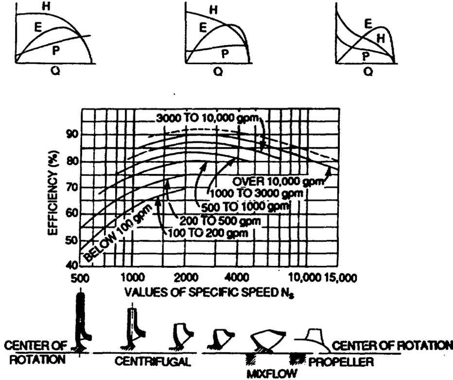
Fig. 3. Approximate relative impeller shapes and performance characteristic variations with specific speed. Reprinted with permission from McGraw-Hill, Ref. 12.
