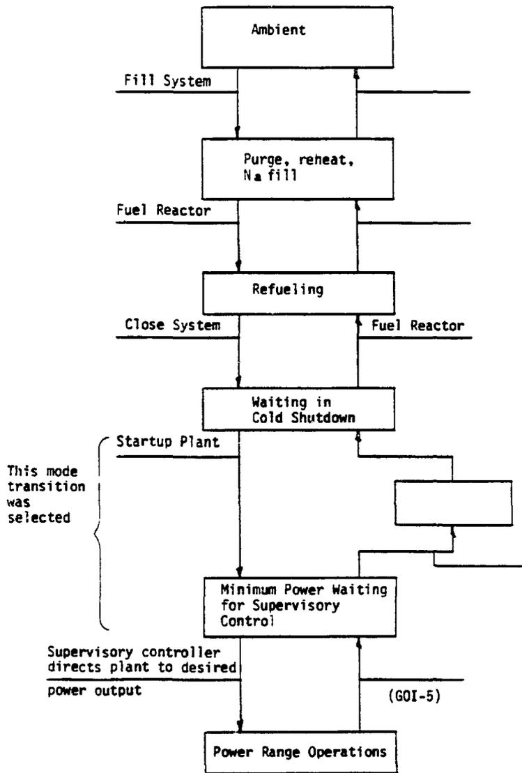
Fig. 6. Overall state-transition model of EBR-II. Note: many transitions have been omitted since this figure represents a framework for illustration only.
