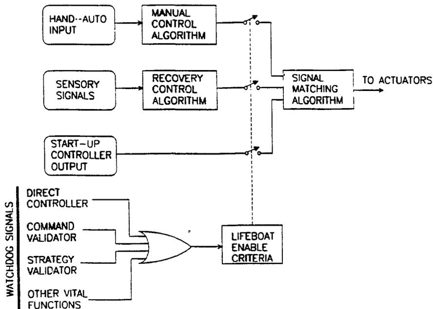
Fig. 3. Simplified diagram of lifeboat controller.
