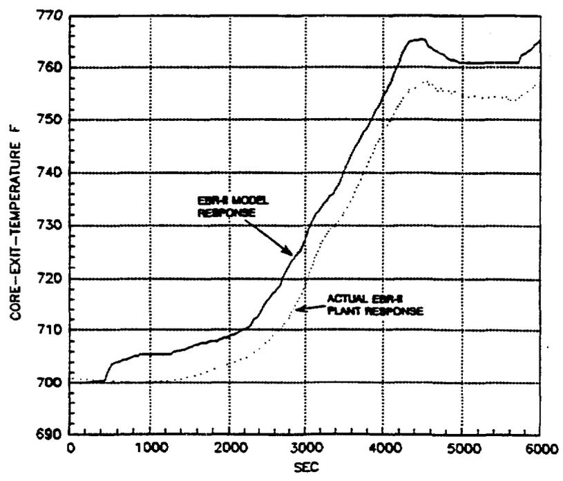
Fig. 5. Core-exit temperature during start-up.
