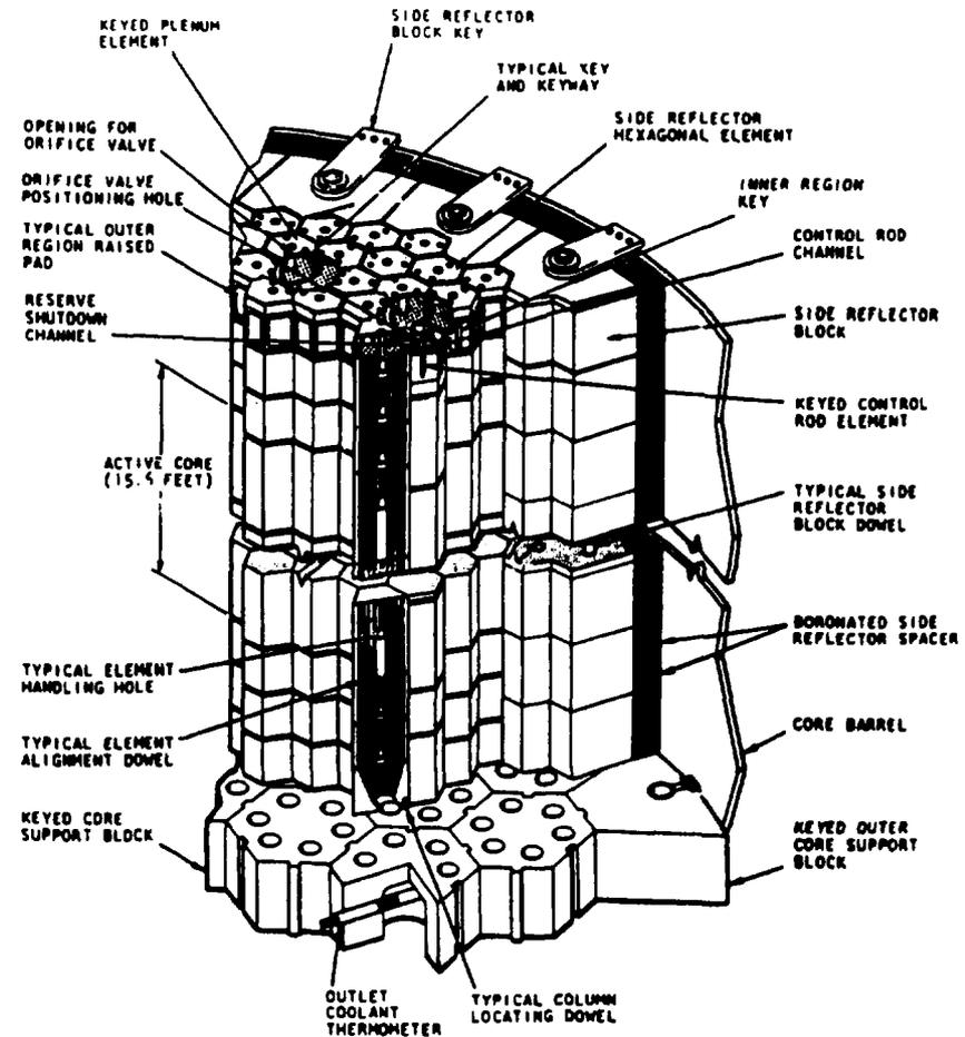
FIGURE 4-Cross Section of Reactor, Showing Representative Column Of Fuel Elements
