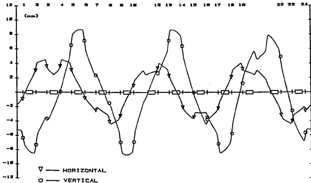
FIG. 16 - Difference orbit with magnetic correctors.
