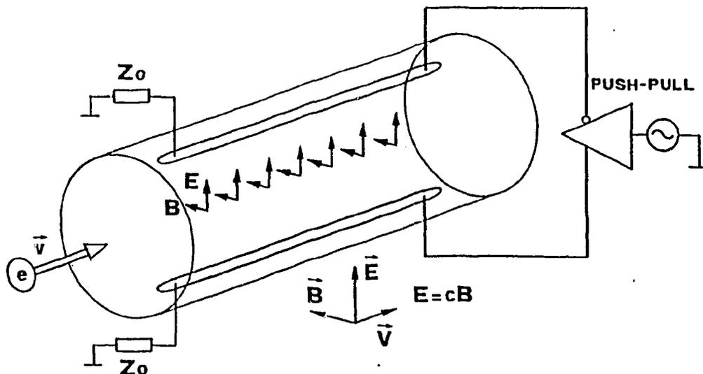
FIG. 10 - Strip line kicker. If the beam and the voltage wave enter the strip-line from opposite directions, the magnetic and electric force add-up and give a deflection. If the voltage wave and the beam velocity are in the same direction the two forces cancel and there is not net deflection.
