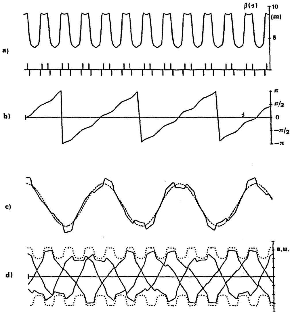
FIG. 1 - a) Example of horizontal betatron function  $\beta(s)$  in Adone (periodicity 12). The ticks mark the position of focusing and defocusing quadrupoles. - b) The betatron phase advance  $\mu(s)$ . - c) Betatron oscillation (solid line) and its smooth approximation (dashed line). - d) Plot of several betatron oscillations with different values of the reference phase  $\phi_0$ . The dotted line is the envelope of the betatron oscillations around the machine.
