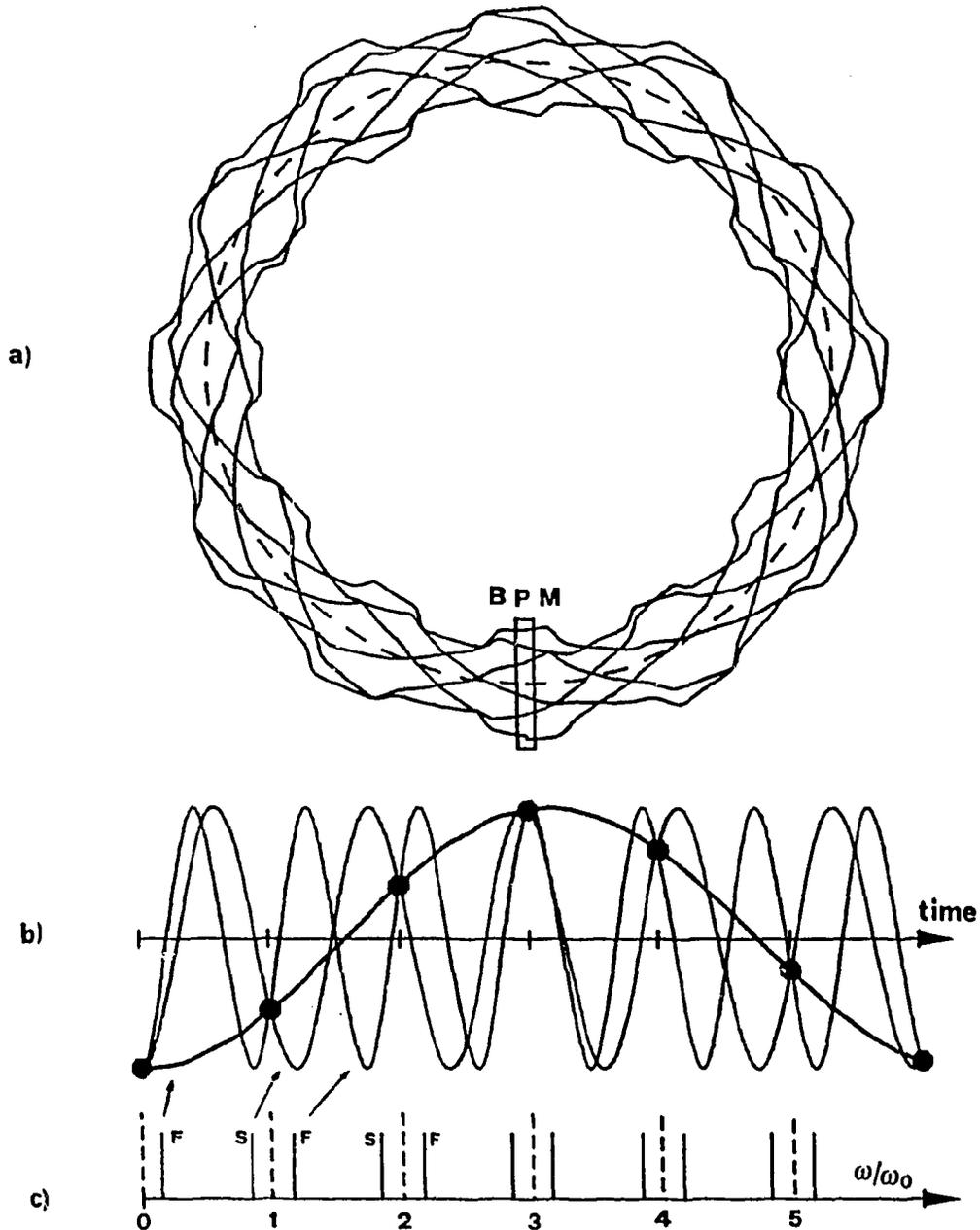
FIG. 3 - a) Betatron motion (exaggerated) of a single particle, traced over 7 successive passages across a BPM. The betatron tune is  $Q = 3.2$ . - b) Heavy dots mark the beam position vs. time. The superposed sinusoidal waveforms are the first few betatron modes fitting the beam position. - c) Spectrum analyzer representation of the waveforms. The dashed lines are the harmonics of revolution frequency, the solid lines labeled F are the fast waves and those labeled S are the slow waves.
