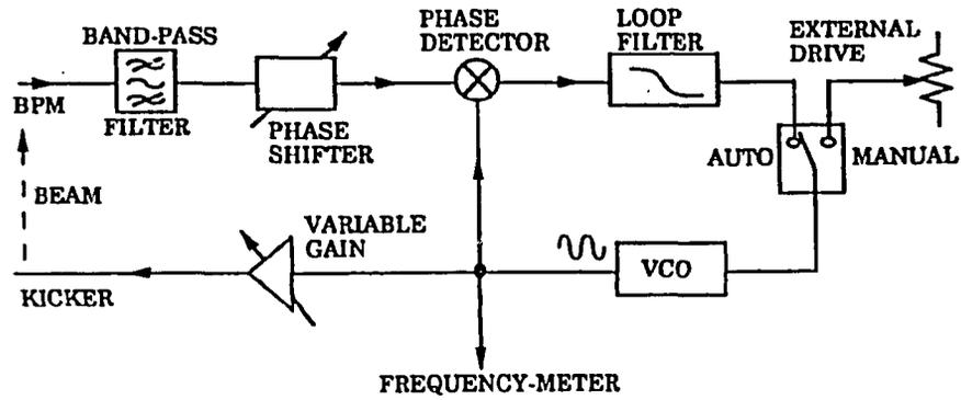
FIG. 15 - Tune measurement with a Phase Locked Loop.
