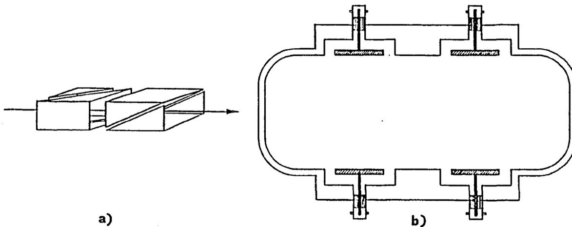
FIG. 6 - *Electrostatic Beam Position Monitors: a) Split electrodes, b) Buttons.*
