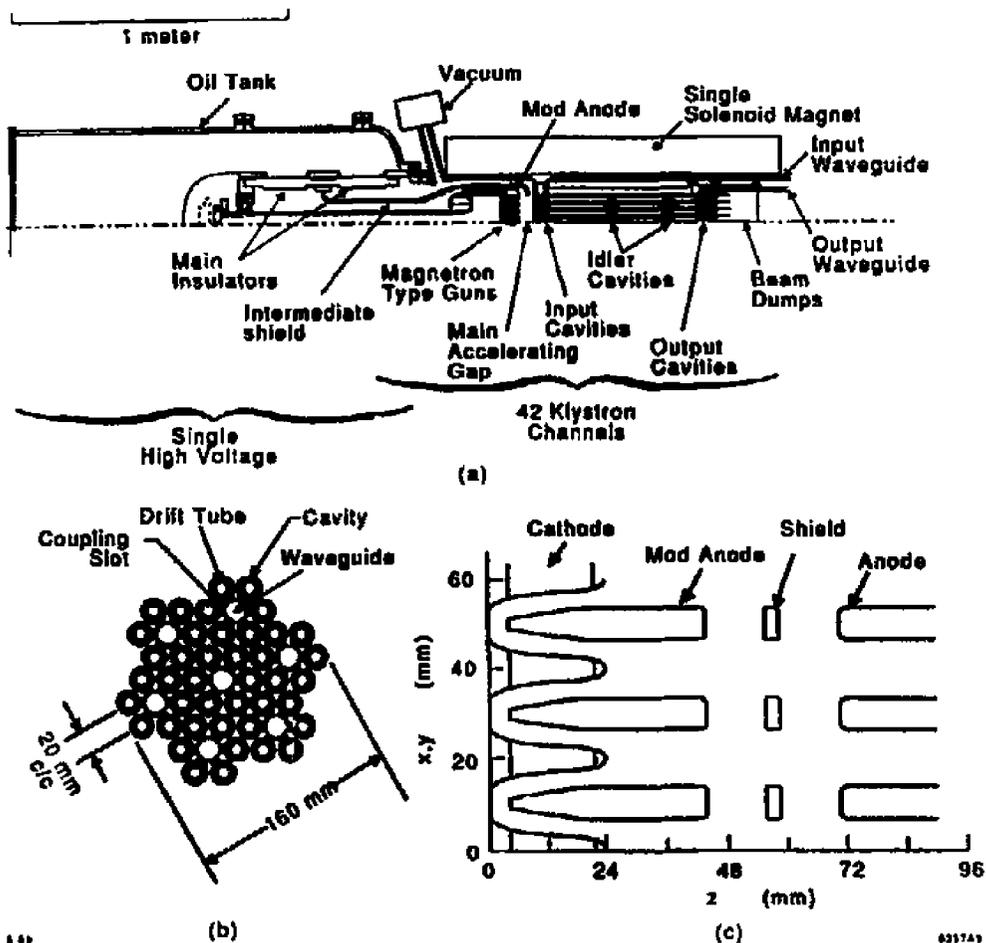
**FIGURE 1** Conceptual design of an immersed field cluster klystron: (a) longitudinal cross section of complete tube including high voltage tank (SLAC lasertron design); (b) possible cross section of 42 individual klystron cavities; (c) enlarged view of three magnetron-type guns.
