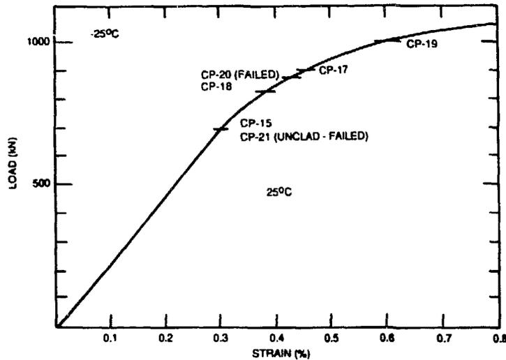
Fig. 4. Point on load vs surface strain curve at which the six plates were tested in the arrest mode. Note that all plates whose designations appear above the curve were tested at  $-25^{\circ}\text{C}$ , while those below the curve were tested at  $25^{\circ}\text{C}$ .
