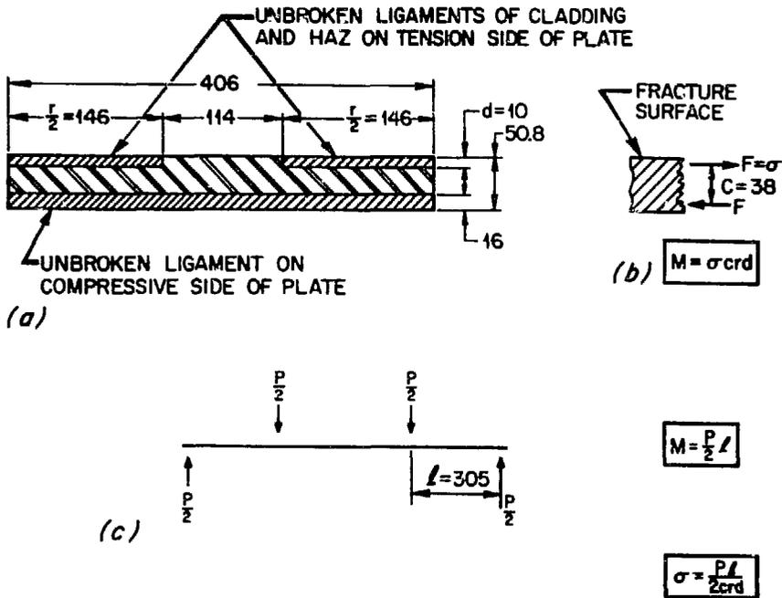
Fig. 8. Analysis of stresses required to rupture the four plates CP-16, CP-17, CP-18, AND CP-19. (a) Idealized, typical remaining ligaments. (b) Forces acting on the fracture surface. (c) Forces and pertinent dimensions of the four-point bend load train.
