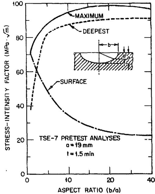
Fig. 1. Variation of the stress intensity factor  $K_I$  for an elliptic flaw as a function of the aspect ratio of the major to minor axes ( $b/a$ ). Source: R. D. Cheverton et al., *Pressure Vessel Fracture Studies Pertaining to the PWR Thermal-Shock Issue: Experiment TSE-7*, NUREG/CR-4304 (ORNL-6177), Oak Ridge National Laboratory, 1985.
