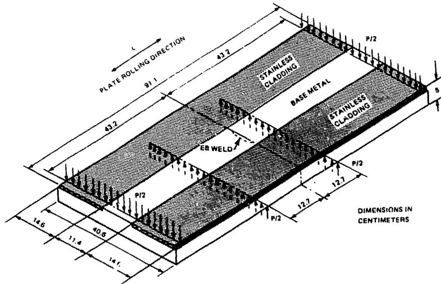
Fig. 3. Clad plate specimen with electron-beam weld tested in four-point bending.
