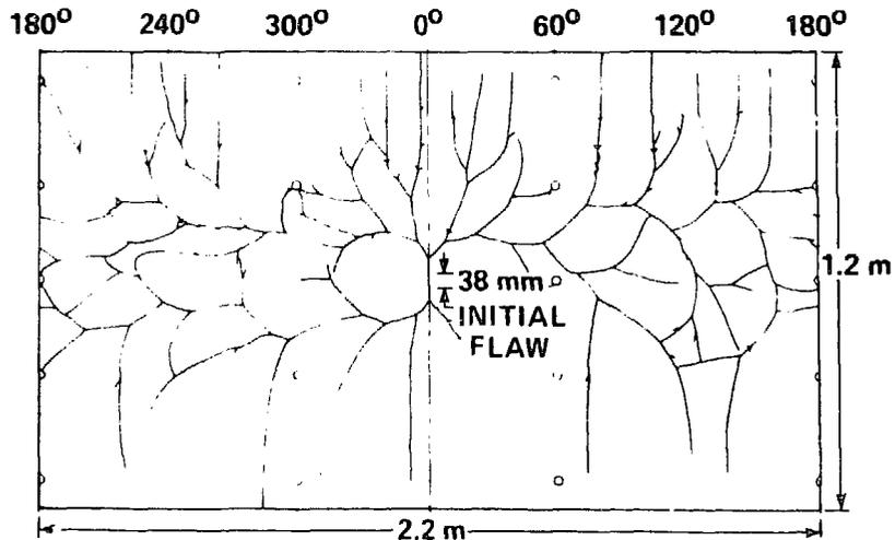
Fig. 2. Developed view of inner surface of the TSE-7 cylinder in which the 19-mm-radius, semicircular flaw propagated on the surface to become a long flaw during the test. Source: R. D. Cheverton et al., *Pressure Vessel Fracture Studies Pertaining to the PWR Thermal-Shock Issue: Experiment TSE-7*, NUREG/CR-4304 (ORNL-6177), Oak Ridge National Laboratory, 1985.
