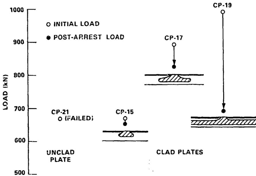
Fig. 5. Initiation loads, post-arrest loads, and corresponding crack lengths for the four plates tested at room temperature.
