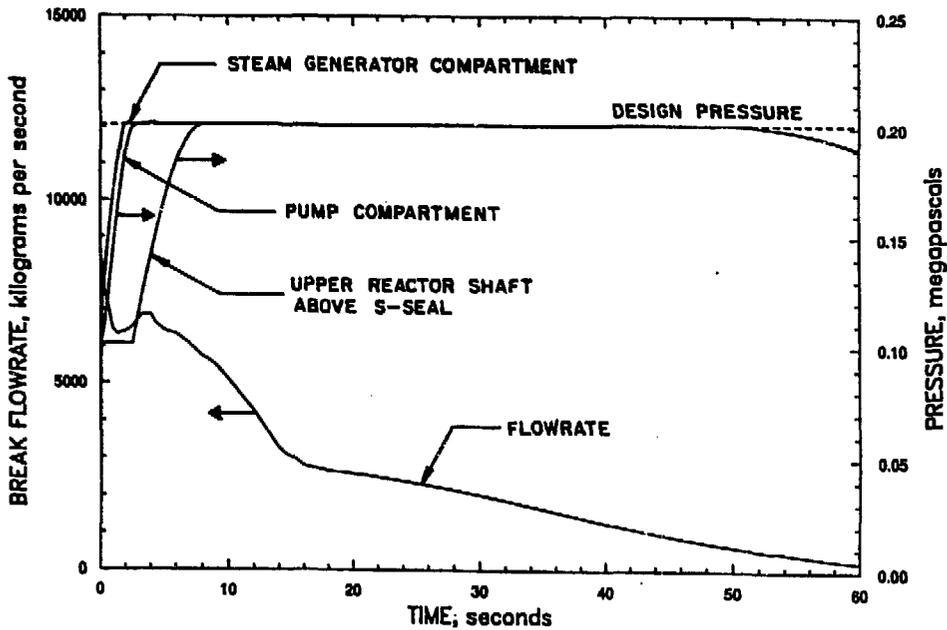
Figure 2. Pressure Loading of VVER-440 Model V230 Accident Localization Volume Following a Primary Coolant Outlet Pipe Break.
