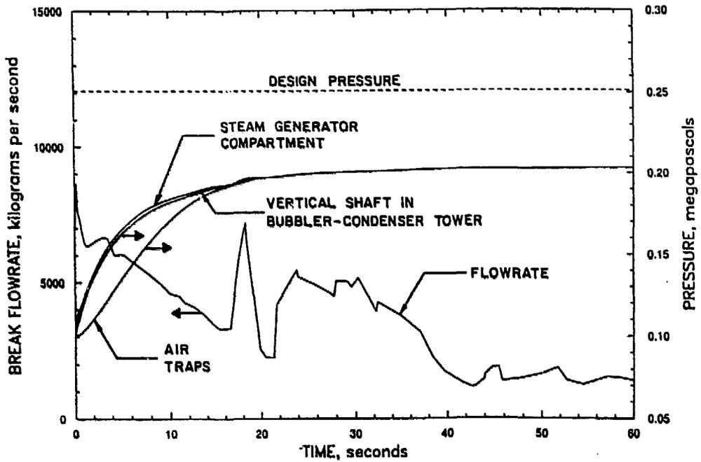
Figure 3. Calculated Pressure Loading of VVER-440 Model V213 Accident Localization Volume Following a Primary Coolant Outlet Pipe Break.
