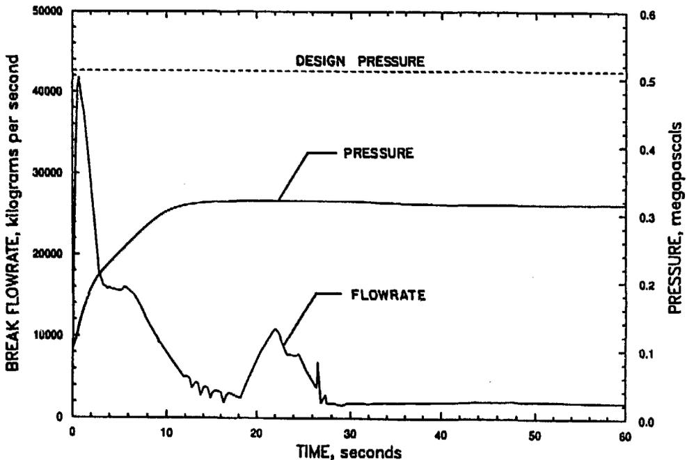
Figure 4. Calculated Pressure Loading of VVER-1000 Model V320 Containment Following a Primary Coolant Inlet Pipe Break.
