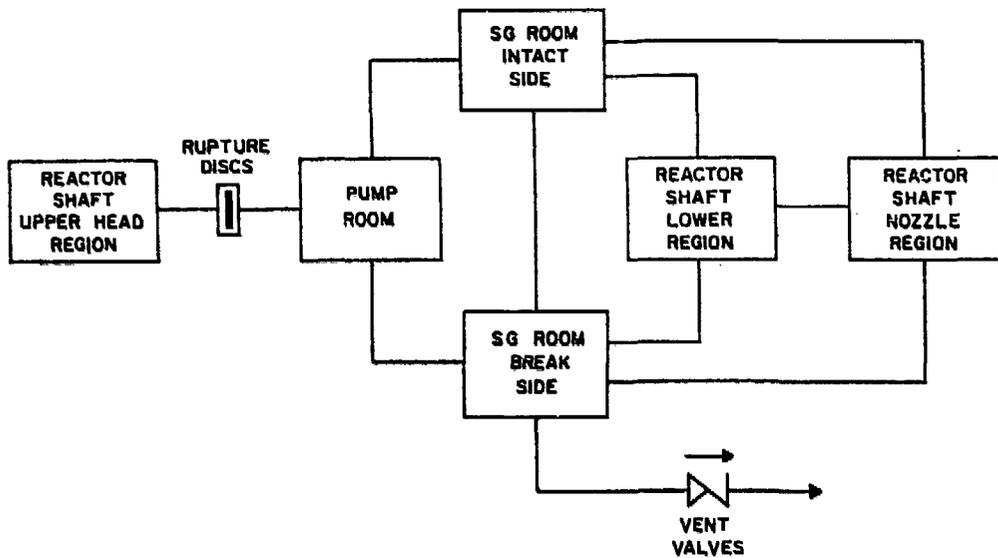
Figure 1. Multicompartment Representation of the VVER-440 Model V230 Accident Localization System.
