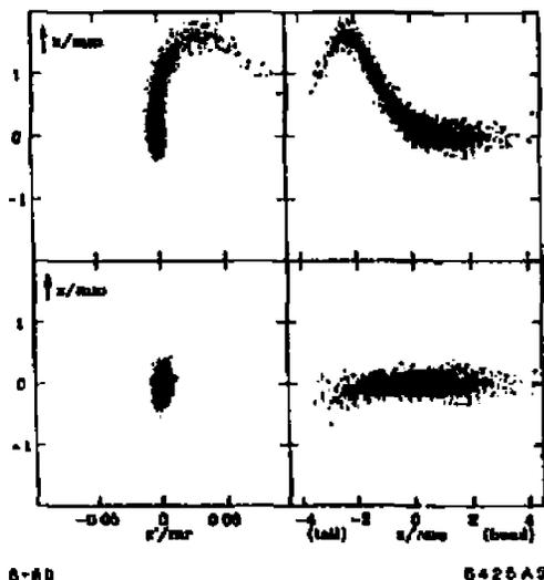
FIGURE 3 The effect of wake field driven emittance growth without (upper two boxes) and with (lower two boxes) BNS damping. The left-hand boxes show the projection in transverse phase space, while the right-hand boxes show the transverse projection along the bunch.
