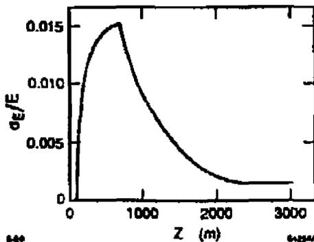
**FIGURE 2** Induced energy spread profile along the linear accelerator for BNS damping at intensities up to  $2.5 \times 10^{10}$  per bunch.
