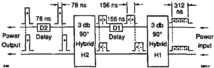
**FIGURE 8** Schematic of a two-stage binary pulse compression system is showing the relative phase during the pulse and the length of the required delay lines.
