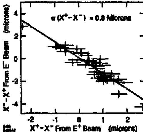
FIGURE 7 Correlation plot showing the pulse-to-pulse jitter in centering of the two beams. The spread of points along the heavy line indicates true beam jitter, while the spread around the line is caused by electronic noise in the pickup system.
