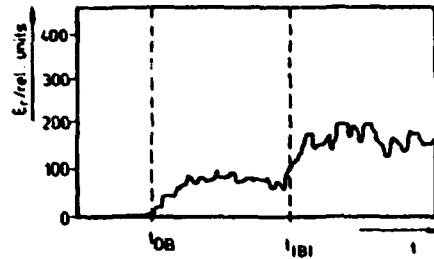
Fig. 9. Measure of burst's energy derived from the r.m.s.-signal ( t_{0B} and t_{1B} being the time of onset of boiling and of increasing the boiling intensity, respectively)
