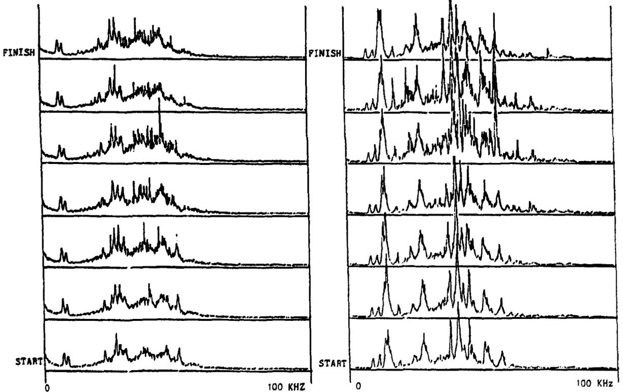
FIGURE 11: Signal Spectrum Development from Start of BOR 60 Tape II to finish of record
