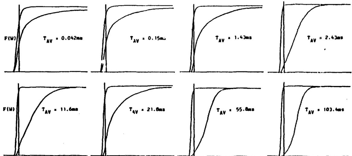
FIGURE 14: Transducer P2 (BOR 60 Tape II) with 4th order differentiation: Cumulative feature PDFs showing decision boundary  $W_1$  for minimum (S.M).
