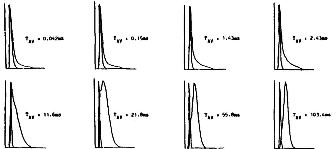
FIGURE 13: Pressure transducer P2 (BOR 60 Tape II) with 4th order differentiation: Separation of flow (a) and boiling (b) feature PDFs with increased averaging time.
