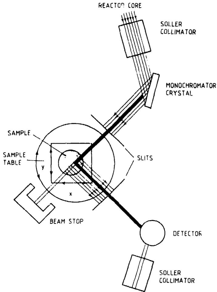
Figure 1: Schematic of residual strain measurement using slits to define a small beam.
