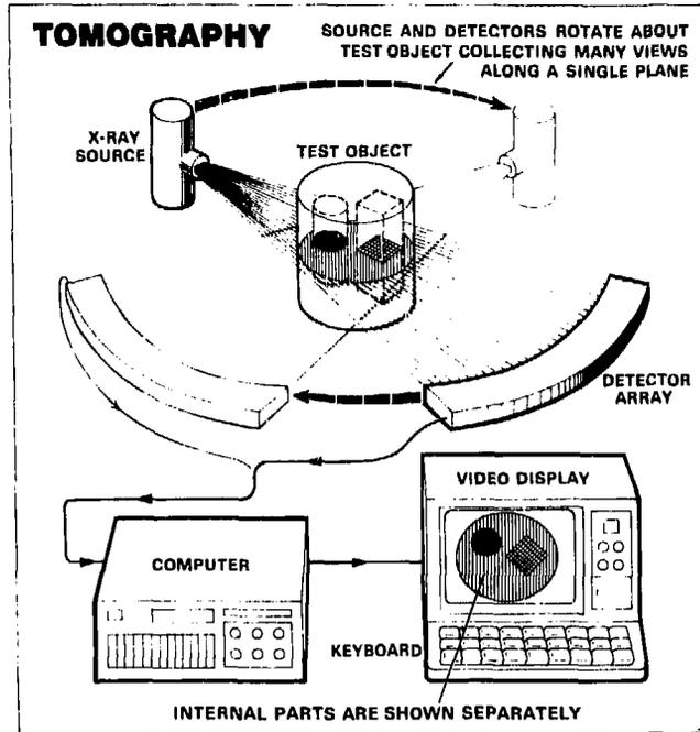
Figure 3: A CT scanner measures X-ray (or gamma-ray) attenuation in a single plane of an object from many different views. The data are stored in computer memory. The computer then reconstructs an image that is a map of X-ray attenuation, which is related to density, and shows the internal features of the cross section in their correct spatial configuration.
