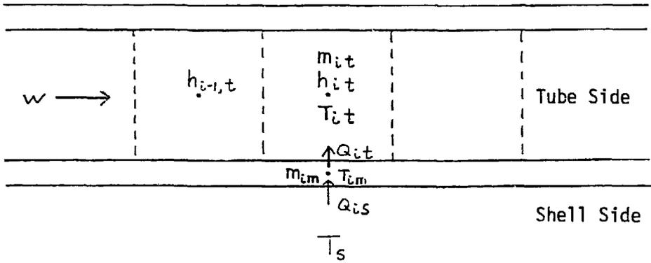
Fig. 2. Tube Side Nodalization
