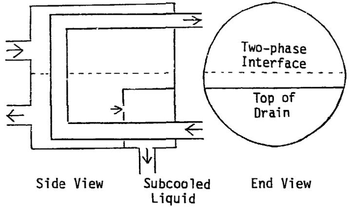
Fig. 1f. Drain Cooler
