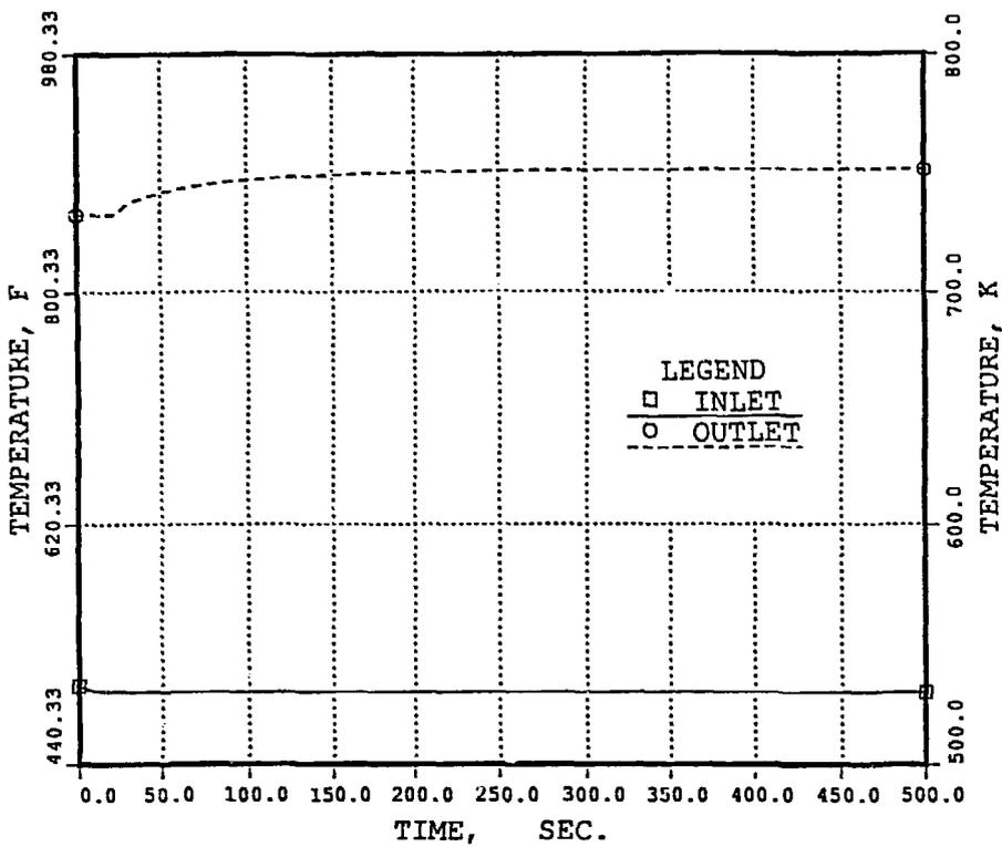
Fig. 4c. Steam Generator Water Temperatures at the Inlet and Outlet
