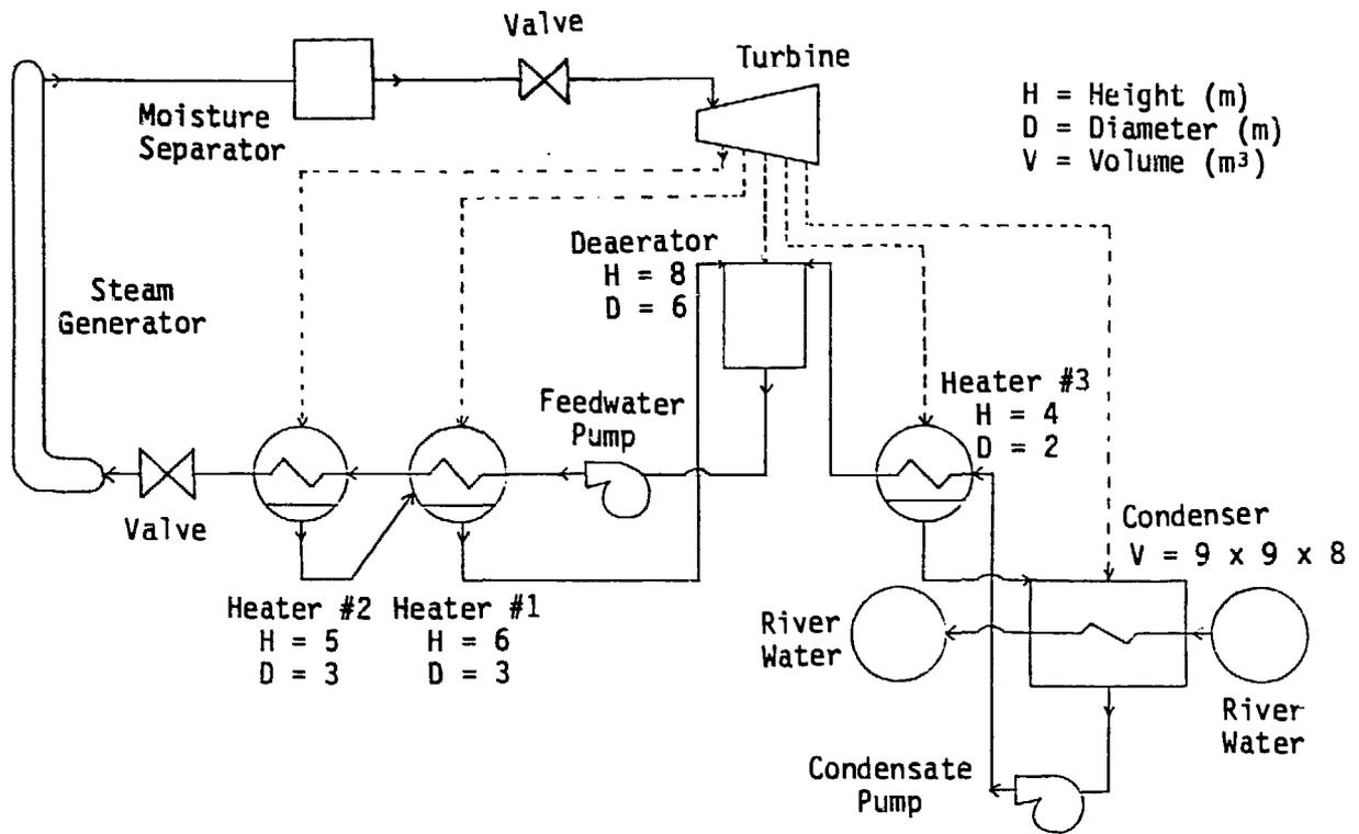
Fig. 3a. Integrated Test Problem Configuration
