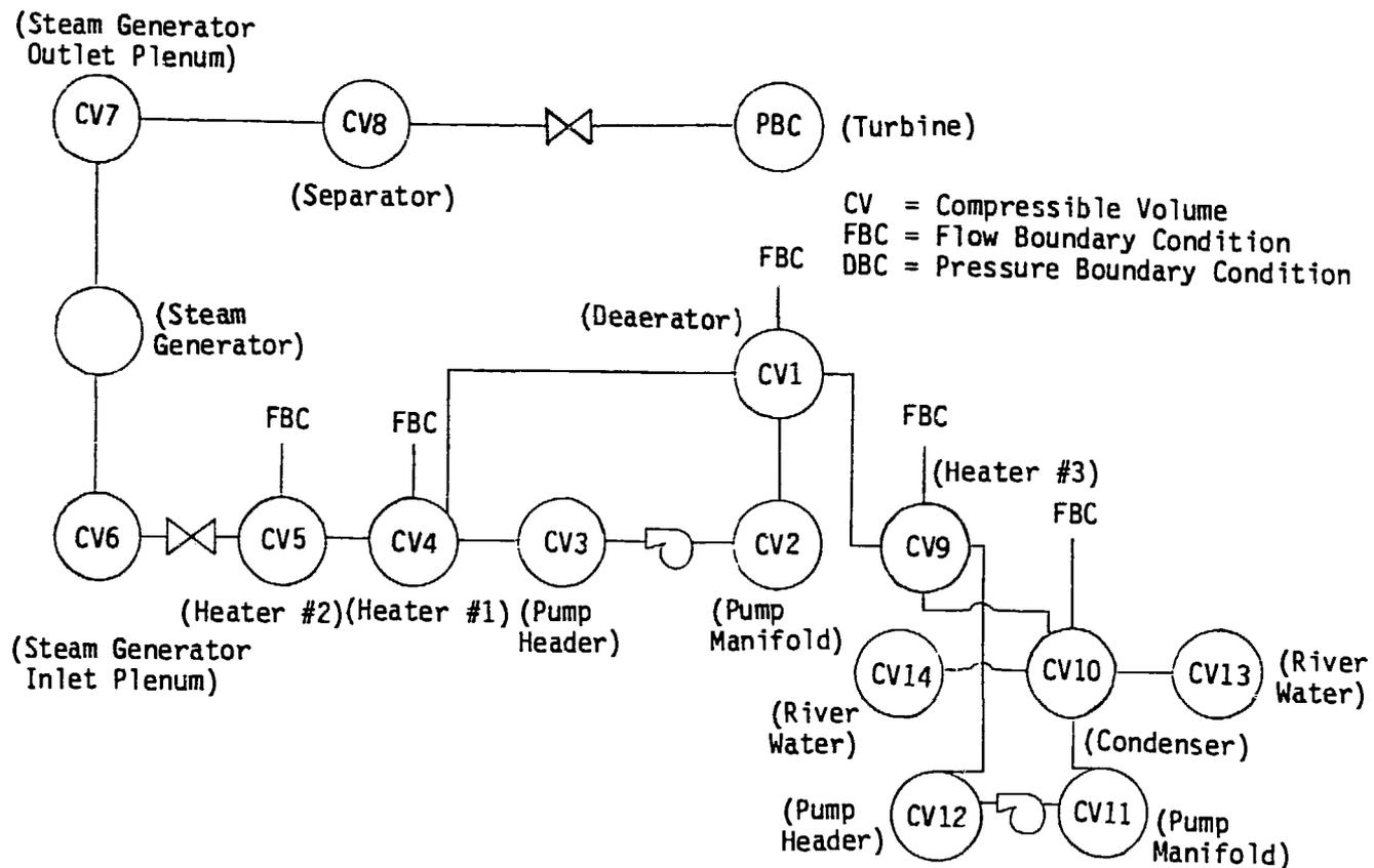
Fig. 3b. Discretization of the Test Problem
