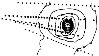
Figure 7. Temperature distribution on a plane perpendicular to the heater at its midpoint.
