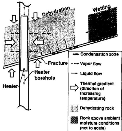
Figure 1. Schematic representation of a probable hydrologic scenario in partially saturated welded tuff subjected to a thermal load.
