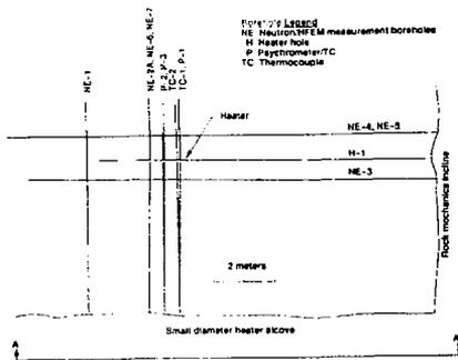
Figure 3. Plan view of the as-built borehole layout. The locations of the Rock Mechanics Incline and the Small Diameter Heater Alcove are shown for reference.
