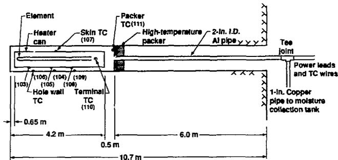
Figure 11. Moisture collection system and thermocouples in the heater borehole.
