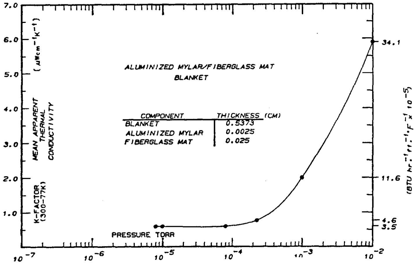
Fig. 4 Thermal conductivity vs. pressure for the insulation package used in SSC dipoles.
