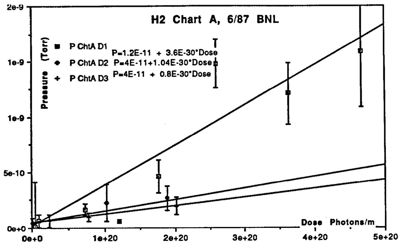
**Fig. 6** The Hydrogen desorption signal as a function of photon dose for three successive runs, with warmup to 20 to 70K in between. Note the strong increase with accumulated dose, and the slope reduction on successive runs.
