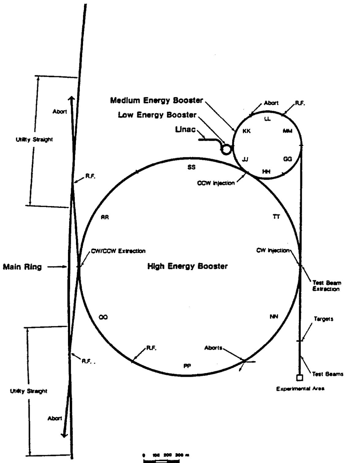
**Fig. 3** The injector system to the Supercollider. Starting with a source injecting protons into the Linac, the energy is raised by three successive booster synchrotrons to the 2 TeV injection energy (the 1986 design report, this picture, still suggests a 1 TeV injection energy).
