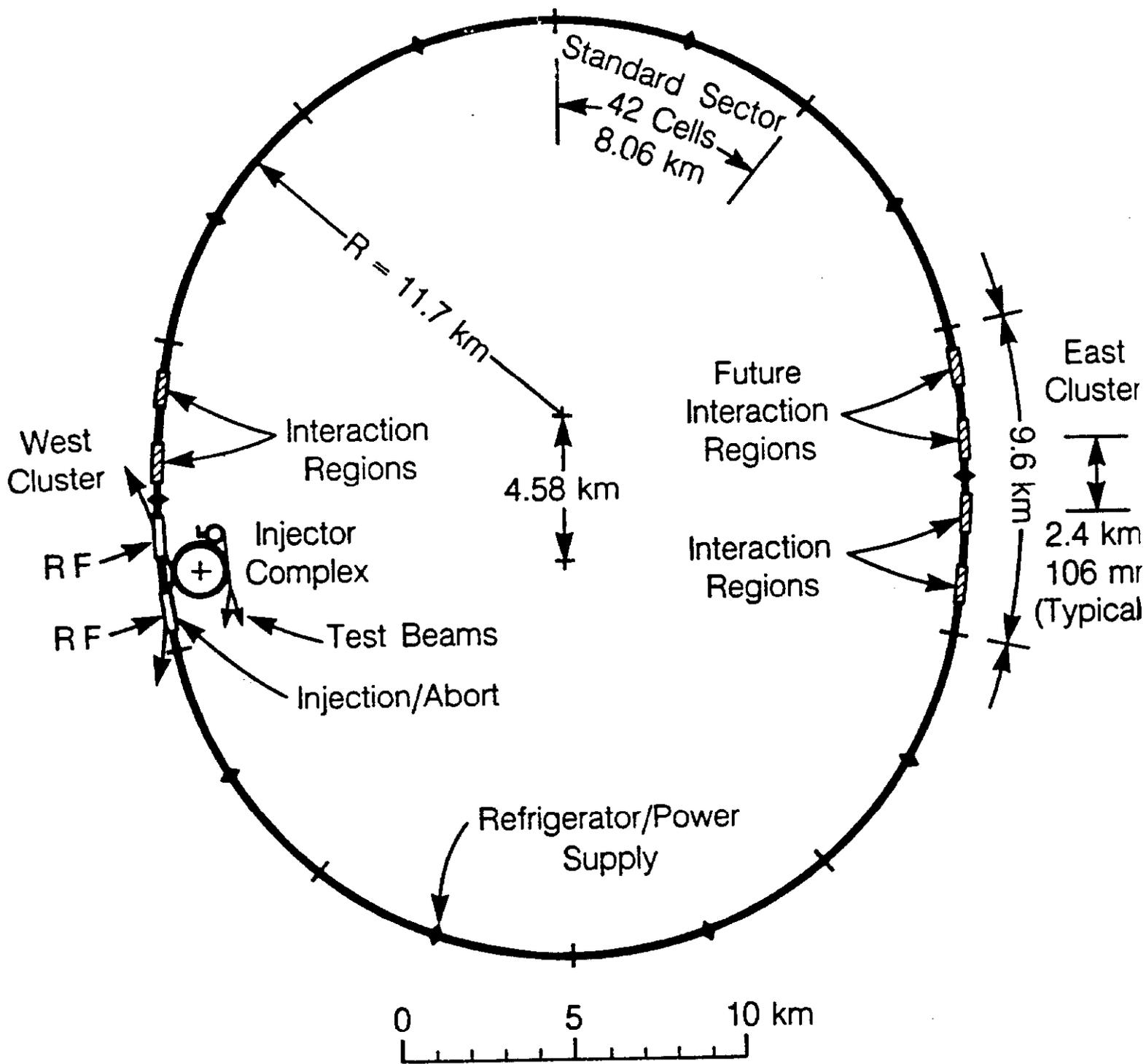
**Fig. 1 SSC Collider ring layout. The cluster regions provide space for experiments. The injector complex is shown near the west cluster. There are 10 refrigeration and power units around the ring (black diamonds).**
