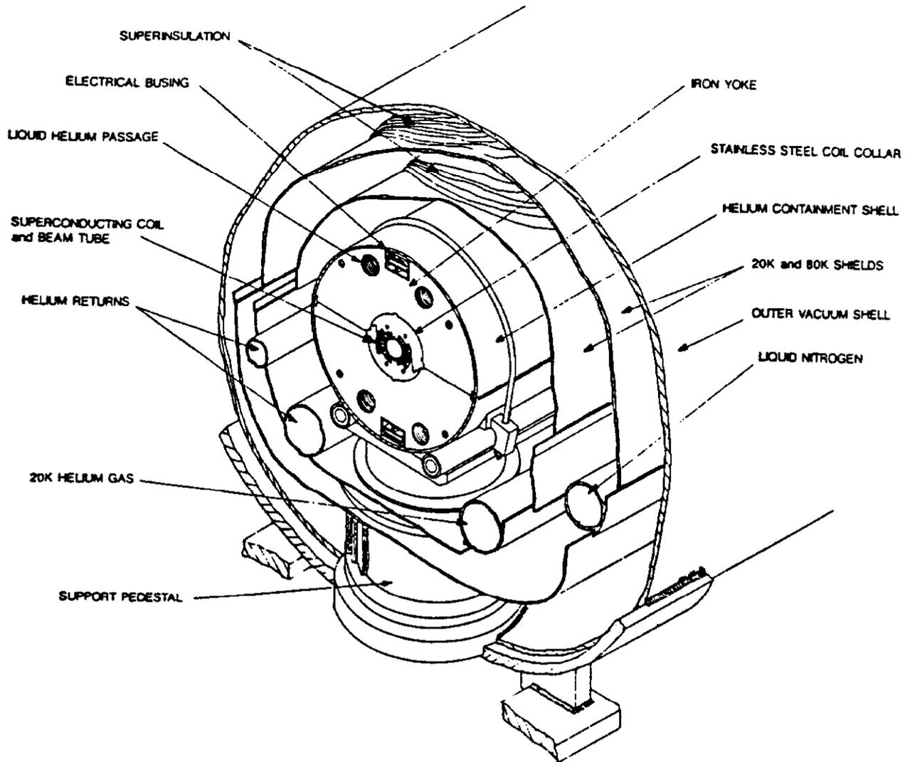
**Fig. 7 Isometric cutaway perspective drawing of the 6.6 Tesla SSC dipole magnet, showing all interconnect pipes.**
