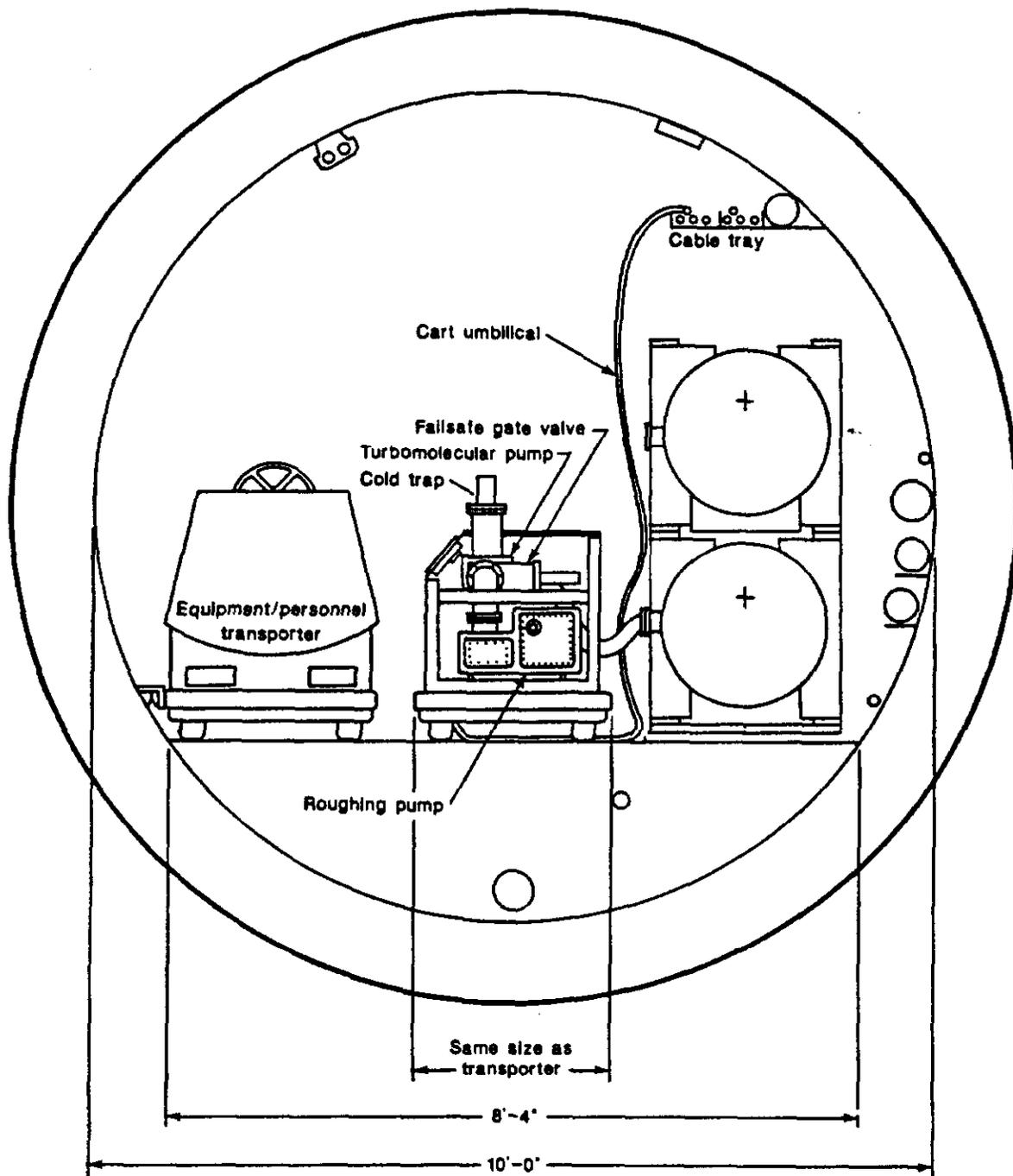
**Fig. 9 Sketch of a pump cart, consisting of a roughing pump, turbo pump, cold trap and a gate valve with associated gauging, controls and computer interface. Such carts will be used for initial pumpdown, leak checking and leak pressure containment.**
