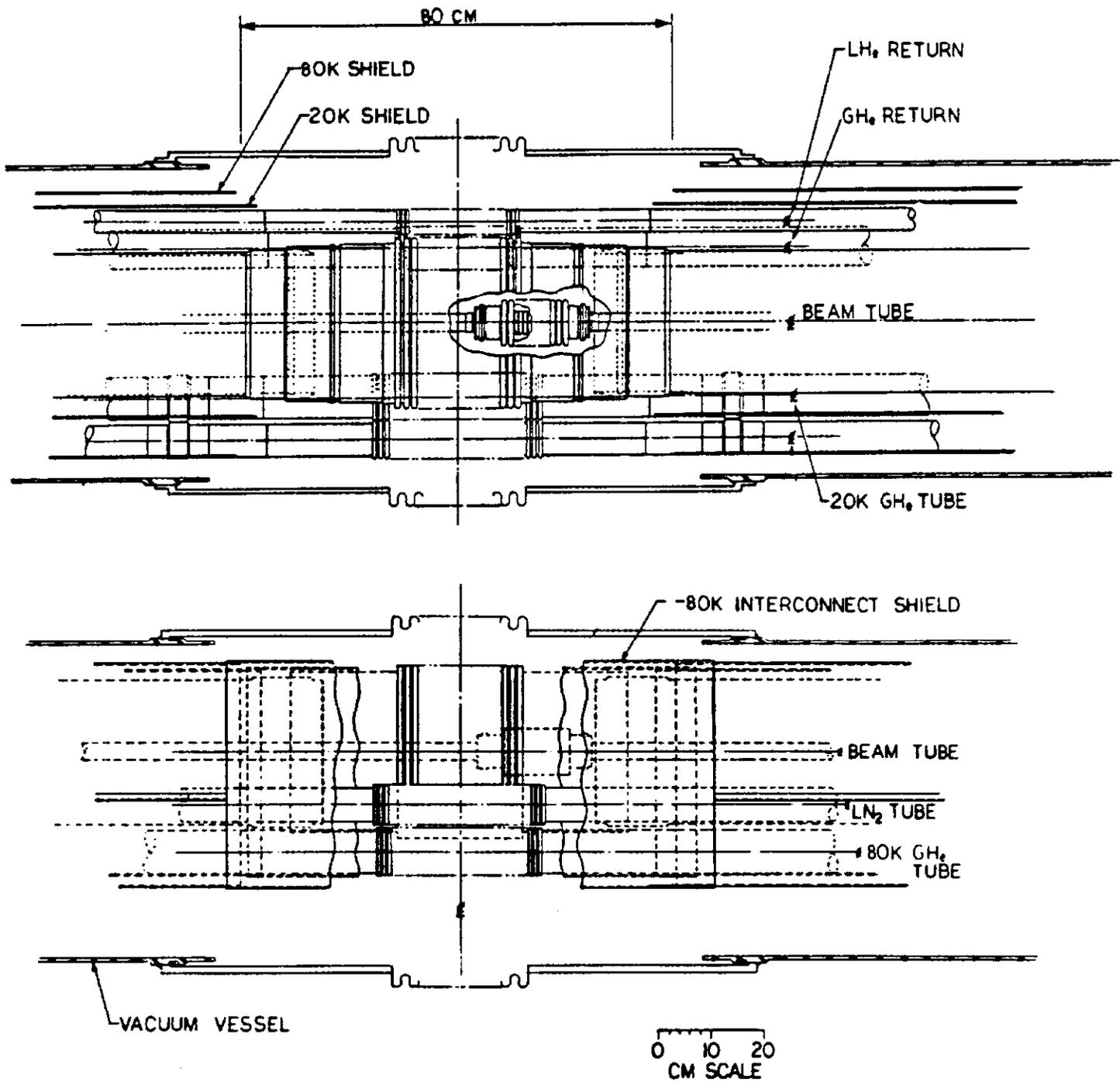
**Fig. 8** Longitudinal sections of the magnet interface piping. All connections are to be welded using automated equipment.
