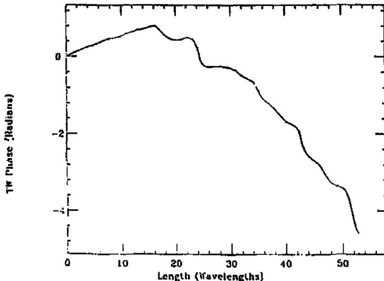
Figure 4c. Relative phase between voltage and current versus distance.
